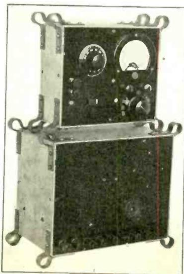
An early model of the Gunn radio altimeter, including the oscillator and the control or indicator unit.
