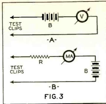
Two test circuits for checking continuity.
