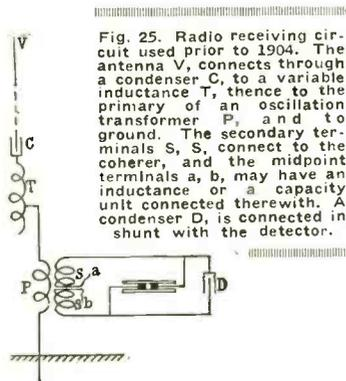
Fig. 25. Radio receiving circuit used prior to 1904. The antenna V, connects through a condenser C, to a variable inductance T, thence to the primary of an oscillation transformer P, and to ground. The secondary terminals S, S, connect to the coherer, and the midpoint terminals a, b, may have an inductance or a capacity unit connected therewith. A condenser D, is connected in shunt with the detector.
