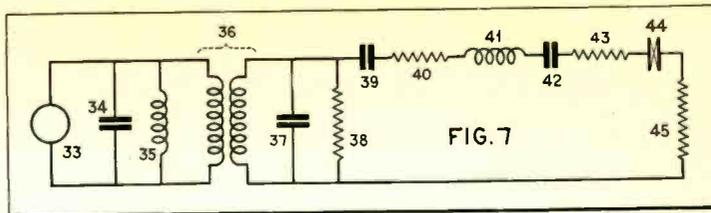
The equivalent diagram of the pickup shown in Figs. 1 and 2.
