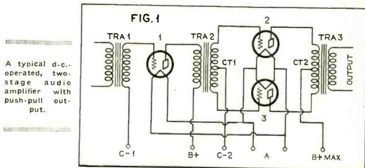
A typical d-c.-operated, two-stage audio amplifier with push-pull output.
