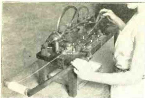
Nucrometer Filament Cutter in DUOVAC Tube Plant
