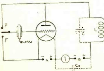
Fig. 22. Circuit connections for a piezoelectric oscillator. The quartz crystal may be inserted between grid and filament or grid and plate, by means of the switch shown on left.
