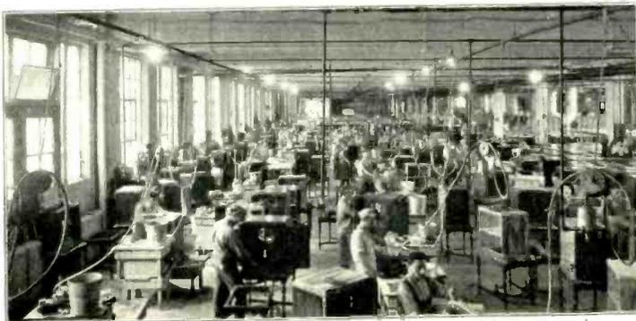
The cabinet-finishing plant of the Grigsby-Grunow Co. where 100 polishing machines, developed by the Paasche Airbrush Co., are doing the work of 400 hand rubbers. The floors in the cabinet shop are of highly-polished hard wood, thus making it possible for a man to slide a line of cabinets from one place to another.
