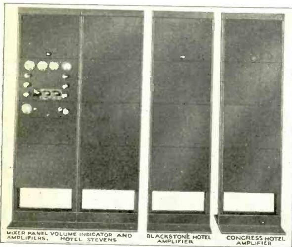
Front view of the amplifier racks installed in the three hotels. The first rack, installed in the Stevens Hotel, contains the three-stage, mixer amplifier, a two-stage amplifier, the volume indicator and the necessary controls. The microphones and pickups fed into this panel.
