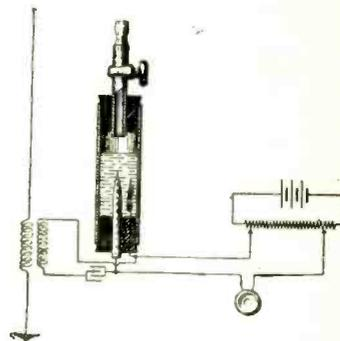
Fig. 24. Fessenden's liquid barretter detector and associated receiving circuits.
