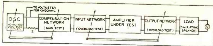
Fig. 2. Schematic diagram of the test panel for making rapid measurements of gain and overload level in amplifiers.
