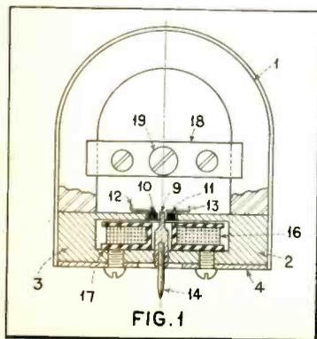
The front elevation of a pickup head. The different parts are explained in the accompanying text.
