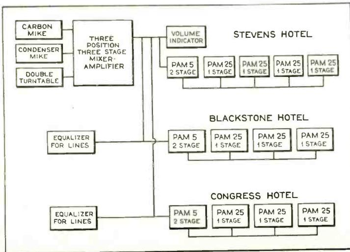
Layout of the equipment which comprised the group address system. Each one stage amplifier fed twelve speakers.
