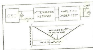
Fig. 1. Outline chart and power level diagram for the gain-measuring method used in the amplifier test set. All impedances are assumed to be matched.
