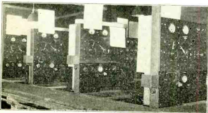
Fig. 4. Four of the group of audio-amplifier test panels as used by the Victor Company for making production inspection tests on completed amplifiers.
