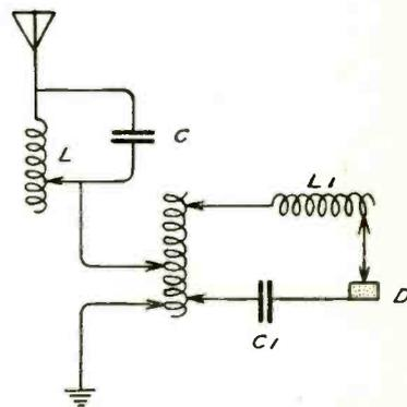
Fig. 26. A typical tuned receiving circuit using a crystal detector.
