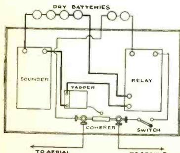
Fig. 23. Actual wiring of instruments used in a radio telegraph receiver employing a coherer as detector. The instrument labeled "tapper" is the de-coherer.
