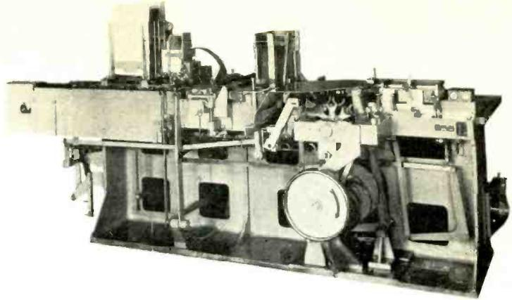
This combination wrapping and cartoning machine for vacuum tubes was developed by the F. B. Redington Co. and wraps 60 tubes per minute at the R.C.A. tube factory at Bloomfield, N. J. The corrugated protector and circular are fed from magazines, shaped, placed over the tube, the whole being slipped into the cartons and the end-flaps tucked in.
