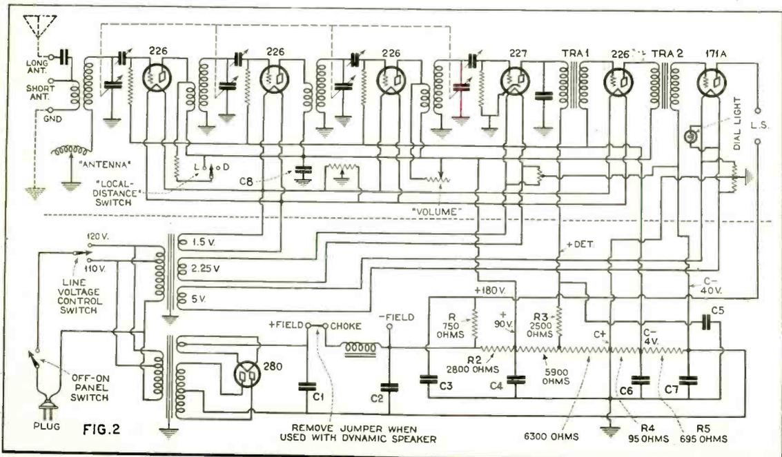
The schematic diagram of the Grebe Synchrophase AC-6.
