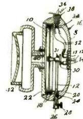
said phonograph or cabinet, and a device in circuit with said radio apparatus and which may be applied to a telephone or a phonograph to transmit or receive and amplify the vibrations of the radio apparatus or the vibrations produced by a record placed in operative relation to the needle of the phonograph.
