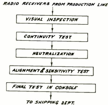
Fig. 3. Receiver inspection and test system.
