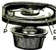
a rocking action on the resistance. Pressure arm "P" together with shaft and bushing is fully insulated.
