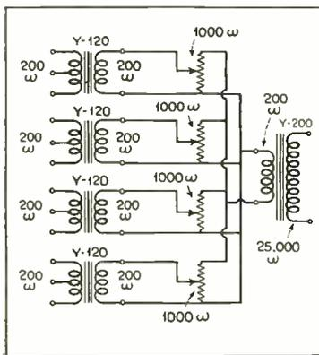
Fig. 16-A. Parallel potential divider type mixer.
