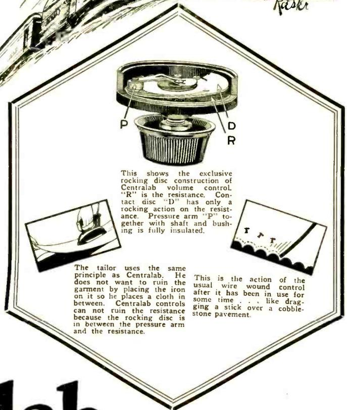
This shows the exclusive rocking disc construction of Centralab volume control. "R" is the resistance. Contact disc "D" has only a rocking action on the resistance. Pressure arm "P" together with shaft and bushing is fully insulated.
