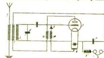
frequency impulses, a detector between the grid and filament of the tube, and means in series with the detector and coupled to said feedback arrangement for biasing the tube in a manner such that sustained radio-frequency oscillations of high amplitude cannot exist.
