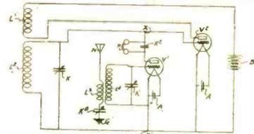
feature resides in the employment of the internal resistance or impedance of a vacuum tube as a variable resistance in the circuit, and the making use of the plate-filament resistance in the reception of the signals.
