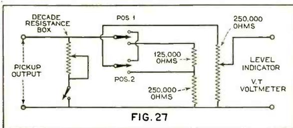
Circuit setting for obtaining impedance of reproducer.
