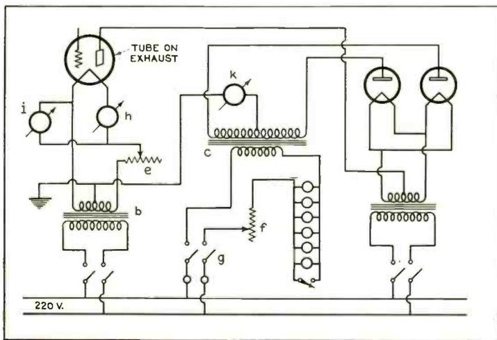
Fig. 2. Power supply unit for exhausting 50 and 75 watt tubes. b Filament transformer—220 v. primary; 2.5 v. secondary, 150 watts. c High voltage transformer—220 v. primary, 6000 v. secondary, 5 KVA, d Rectifier filament transformer—220 v. primary, 2.5 v. secondary, 50 watts. e Rheostat—6 ohms, 9 amperes. f Rheostat—50 ohms, 7½ amperes. g Toggle switch extension handle, h Ammeter 0-5 a-c. i Voltmeter 0-5 a-c. k milliammeter 0-800.
