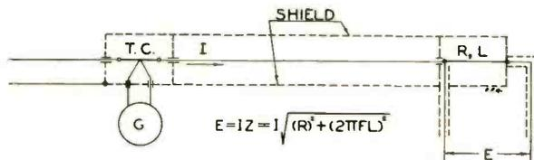
Fig. 3. N. P. L. shielded small impedance (schematic).
