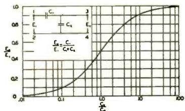
Fig. 2. Capacities as dividing elements.
