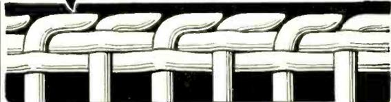
"Sealedged" is rated by many engineers as the highest development in nickel wire cloth construction. Only nickel of highest purity (over 99%) is used. It is the ideal material for grid screen use and for application in other new tubes. In fact, wherever wire screen is used in electron tube practice "Sealedged" should be employed.
