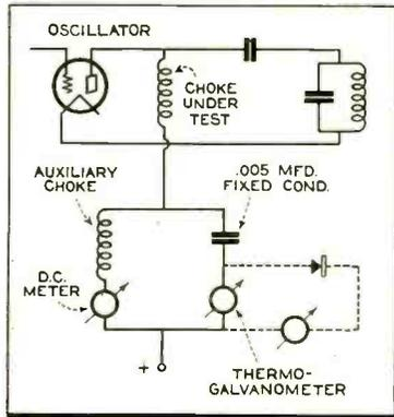
Fig. 3. One method of testing chokes.
