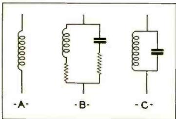
Fig. 1. Theoretical choke as at A. Practical chokes function as B, and C.
