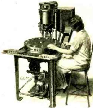
Machine indexes very smoothly and rapidly at fixed intervals of time, regulated by three step pulley on motor. Base holding chuck rotates only when in filling position and automatic filling arrangement moves down to fill base. A uniform filling is assured by this method. A regulating cup is filled with alcohol keeping free the filling device. Track arrangement lifts filled base, making removal of base easy.
