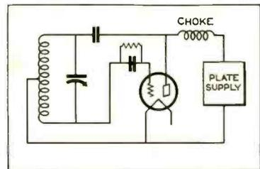
Fig. 2. Shunt-feed Hartley Transmitter circuit, showing choke coil.
