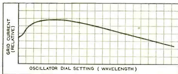
Fig. 5. Typical curve showing variation of grid current with increasing wave length.
