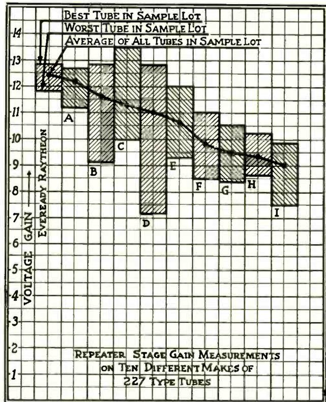
Obviously, their elements did not maintain proper alignment, under conditions of rough handling inevitable in transportation. Eveready Raytheon elements can and do —because of the strength and rigidity of the 4-Pillar construction.
