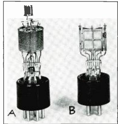
A. Type 24-A tube showing plate, mesh screen, getter cup, support wires and all parts except filament and top cap made of "Svea."
