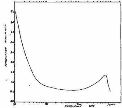
Fig. 2. Dial accuracy curve beat frequency oscillator.
