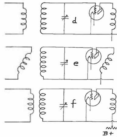
(d) Stabilizing by making the coupling between the primary and secondary coils very loose.
