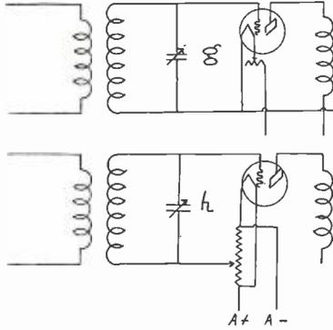
(g) Stabilizing by adjusting the temperature of the r-f. amplifier tube.
