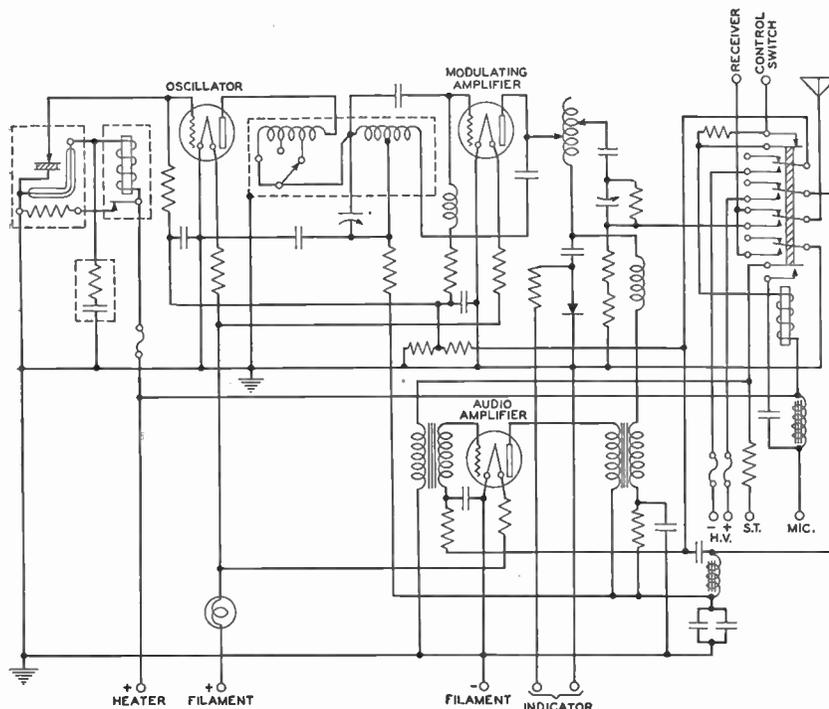
Fig. 1. Schematic diagram of the IIA transmitter.
