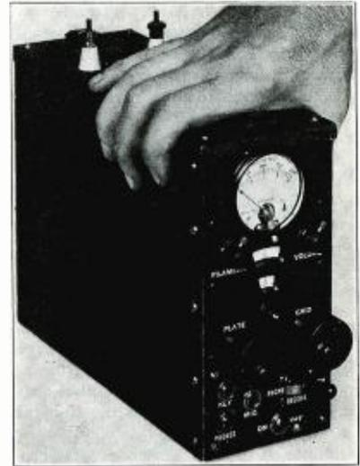
New Transceiver, weight 22 pounds with battery unit. One-half watt power. Five meter wave-band.
