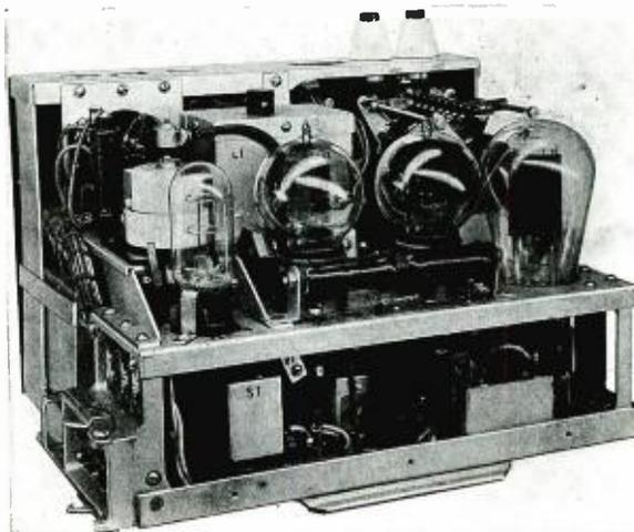
Fig. 2. The extremely compact arrangement of the transmitter is evident when the sides and top are removed. The bulb at the left is the ballast lamp used to control current to the filaments.
