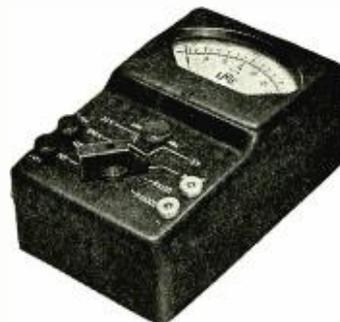
deep. Voltage ranges are 3, 30, 300 and 600. Resistance ranges are 0 to 1,000; 0 to 100,000 and 0 to 1 megohm. With minor wiring changes and the addition of IRC Precision Wire Wound Resistors, various d-c. current readings can be made. The basic meter used is an 0-1 milliammeter.
