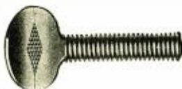
vides a firm finger grip. The screws are rolled-threaded to close limits. They are made for stock in a complete range of sizes—from 3/16 inch—24 by 1/2 inch to 3/8 inch—16 by 3 inches inclusive.
