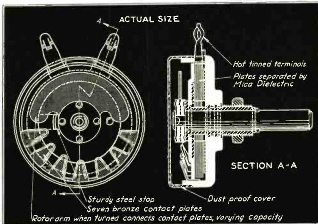
**SPECIFICATIONS**—Standard shaft  $\frac{3}{4}$ " long. Standard bushing  $\frac{3}{8}$ " long,  $\frac{3}{8}$ " diameter, 32 threads per inch. (Shafts and bushings can be made to your specifications.) Standard Capacity has range from 50 M. MFD. to .006 MFD. (Other capacities available from almost zero to .01 MFD.) Dimensions:  $1\frac{1}{8}$ " diameter by  $1\frac{1}{16}$ " deep. OCTAVE TONE CONTROL furnished with or without power switch.
