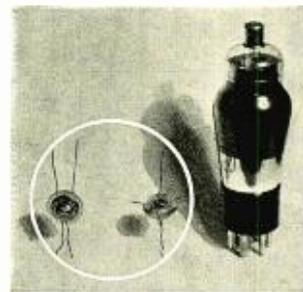
*An example of RCA Radiotron research—a miniature laboratory tube used in research on ultra-short waves.*
