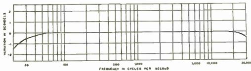
Frequency characteristic of a typical UTC mixing transformer operating at +10 level.
