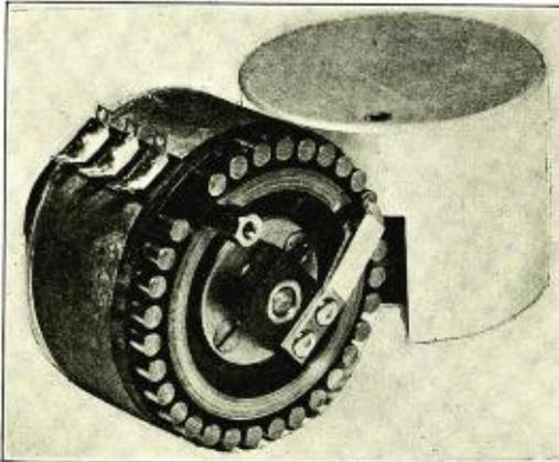
The above mixer is new and entirely different. You will note by its unique construction that the resistance elements are entirely enclosed. No perishable resistance pile winding is used. The silk-insulated resistance wire is wound on thin bakelite strips and placed in a rigid position. The resistance strips are shielded at all times and cannot be tampered with unless taken apart. No tools, soldering iron, dust, water or stray wires can reach the resistance elements.
