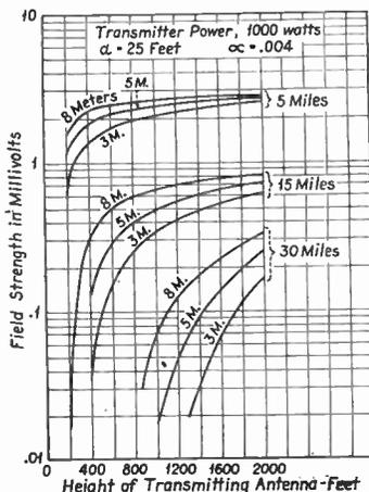
Fig. 1. Full strength versus transmitter antenna height.
