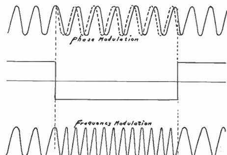
Fig. 1. A wave of constant amplitude modulated in phase and in frequency.
