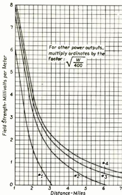
At left: Fig. 2. Field strength versus distance ultra - short waves. Output power: 400 watts. Wavelength: 10 meters. No. 1. Transmitter height —50 feet. No. 2. Ditto—100 feet. No. 3. Ditto—150 feet. No. 4. Ditto—200 feet. Data computed from formulas of Jones (Proc. I. R. E. 21, p. 832, March, 1933).
