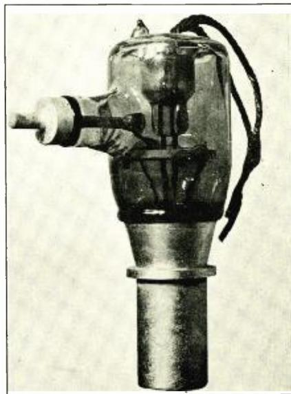
Fig. 6. Type 846 ultra-short wave tube.
