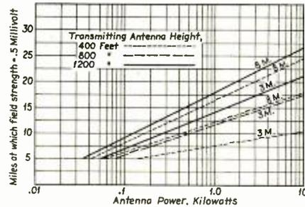
Fig. 4. Half-millivolt range versus kilowatts.
