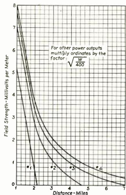
At right: Fig. 3. Field strength versus distance ultra - short waves. Output power: 400 watts. Wavelength: 7.5 meters. No. 1. Transmitter height —50 feet. No. 2. Ditto—100 feet. No. 3. Ditto—150 feet. No. 4. Ditto—200 feet. Data computed from formulas of Jones (Proc. I. R. E. 21, p. 832, March, 1933).
