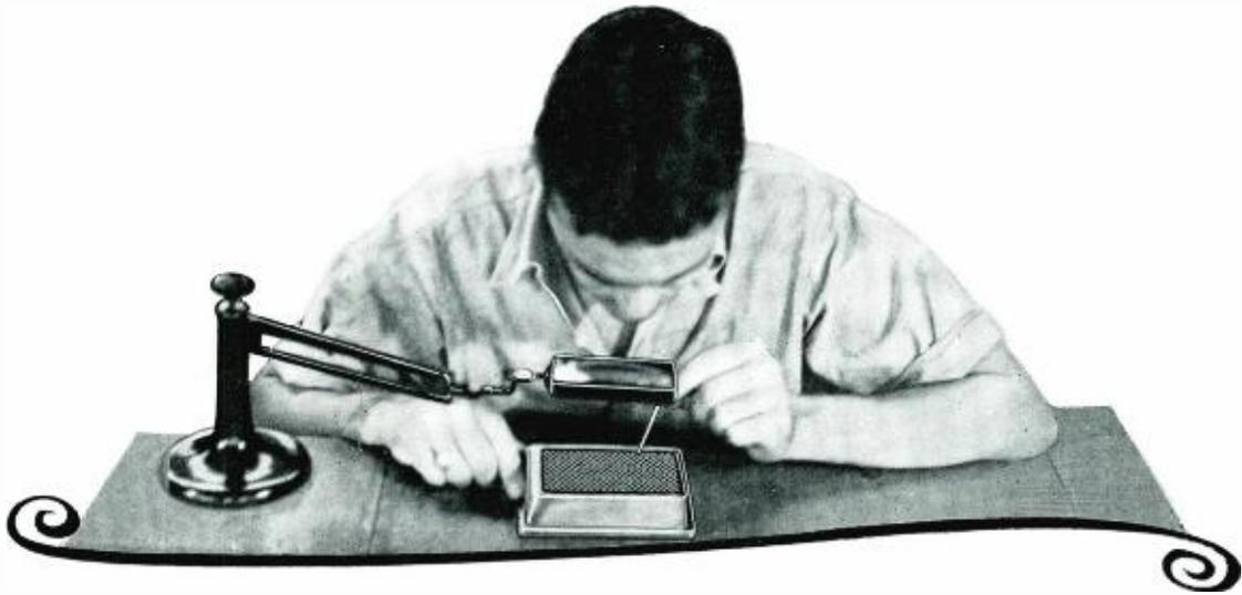
*Photograph of inspector in Summerill Radio Division inspecting Cathode sleeves thru magnifying glass. Nickel sleeves are in a steel box of accurate height as a final check on uniform length of each sleeve.*
