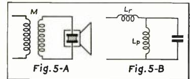
reactance ( $L_r$ ) is obtained to offset the tendency for increase in output with frequency inherent with the crystal.
