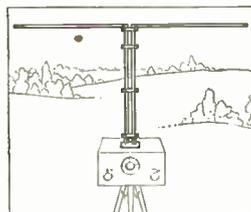
to mount the antenna directly on a transmitter or portable transmitter case, or the antenna may be suspended in the air between convenient supports (for increased optical range) with a transposed transmission line back to the main equipment. Impedance remains accurately matched regardless of the method of use. With the aid of plug-and-jack fittings, the change from direct plug-in mounting on case to overhead suspension may be made quickly and easily without tools. No internal wiring
