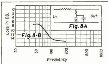
and capacitor are connected in series. This tends to produce sharp attenuation at the resonant frequency if the units are connected in shunt with the line. If connected in series, attenuation is obtained at all frequencies but the resonant frequency. One of the more elaborate types of equalizer covering both high and low end and involving both the shunt-resonant circuit and series-resonant circuit is illustrated in Fig. 11-A with the corresponding frequency characteristic obtained in Fig. 11-B.
