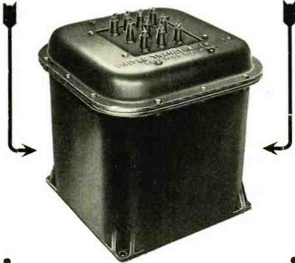
The output transformer illustrated, designed either for 204 A's or 849's in class B, has a linear response from 30 to 12,000 cycles. The unit is oil immersed and shielded in a heavy gauge high permeability casting. All leads are terminated in high tension ceramic bushings. The transformer is insulated for 20,000 volts and will handle 1000 watts audio power.
