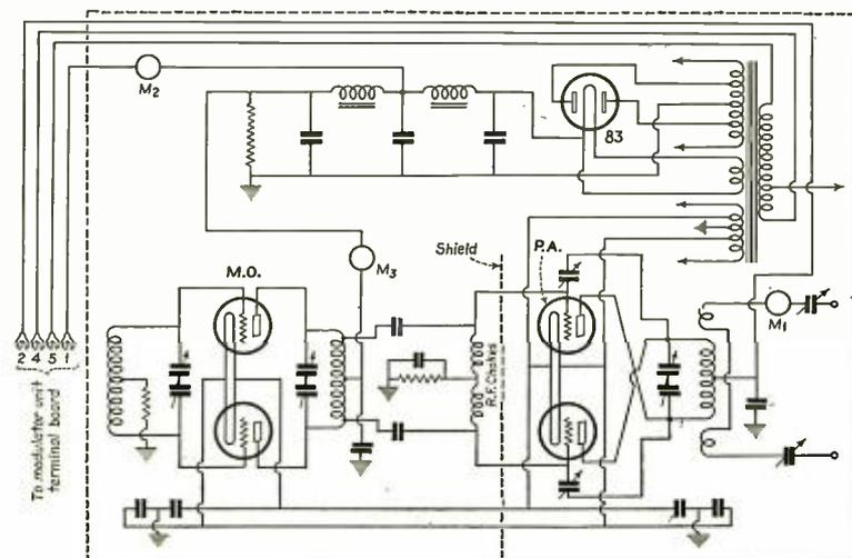
Fig. 2. Circuit of the master oscillator, power amplifier unit, with its individual power supply. Means are provided for increasing the filament and plate voltages on the four tubes.
