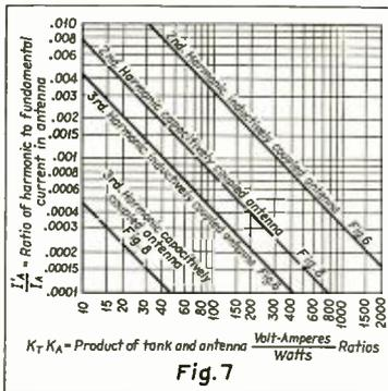
Harmonic content of antenna current for circuits of Figs. 6 and 8.
