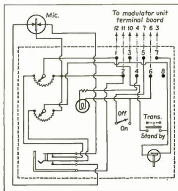
Fig. 4. Circuit of the control unit, with volume control and double-button microphone.
