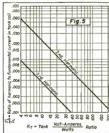
Harmonic content of tank coil current for circuit of Fig. 3.
