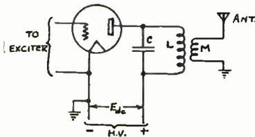
Fig. 1. Simple amplifier circuit.
