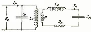
Fig. 6. Inductively-coupled antenna circuit.
