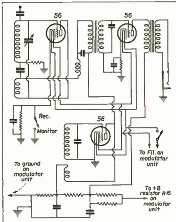
Fig. 5. Circuit of the super-regenerative receiver unit, which may also be used for monitoring.
