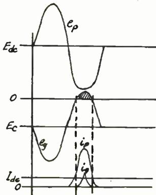
Fig. 2. Tube currents and voltages.
