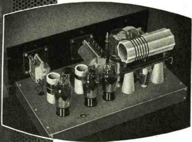
The Collins Radio Company employ ISOLANTITE extensively in the 10-J unit of their type 30 FXB short-wave transmitter.
