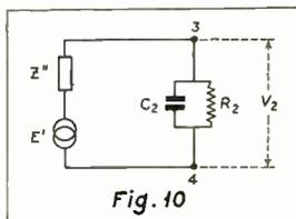
Right: Circuit of Fig. 8 having  $R_2$  paralleled by  $C_2$ , the latter representing stray capacitances.
