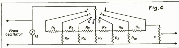
Similar to the circuit of Fig. 3 with the exception that the measuring device, M, is switched along the ladder network.
