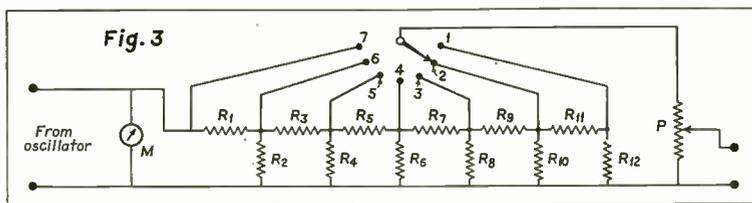
Circuit of attenuator with the potentiometer in the output leg.
