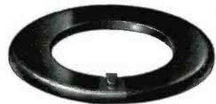
**A SOLID MOLDED RESISTOR—NOT A FILM-TYPE UNIT**—The Type J resistor is homogeneous—in longitudinal section the material is varied to suit specified resistance-rotation curves. After molding, the unit cannot change. Hard service cannot alter its performance. Practically any resistance-rotation curve shape can be provided including straight logarithmic, modified logarithmic, or linear.
