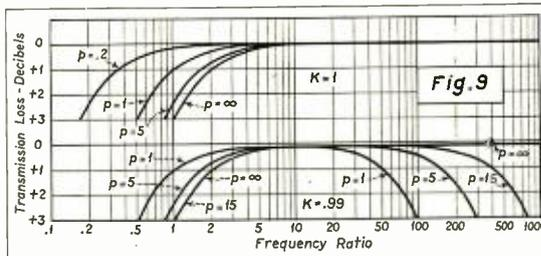
Two families of transmission loss—frequency ratio curves plotted from equation 7.
