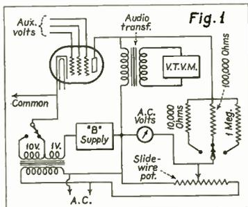
Schematic diagram of the plate-impedance bridge.
