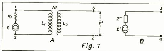
The transformer circuit of A may readily be changed to the simple circuit of B which consists of an emf source and impedance in series.
