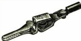
The following are the exclusive design features claimed for this clip: Meshing teeth on three sides of jaws, both screw and banana terminal connections, unusual strength, handiness, and an insulator (sold separately) to prevent short circuits and electric shocks. An internal recess at the end of the insulator automatically snaps around the tubular barrel holding the clip firmly.
