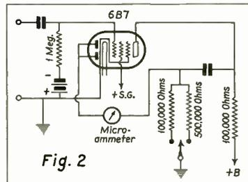
Schematic diagram of the vacuum-tube voltmeter.
