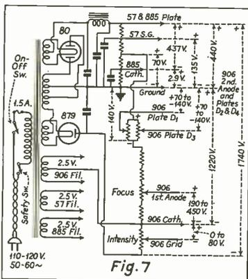
Diagram of the complete power-supply network.
