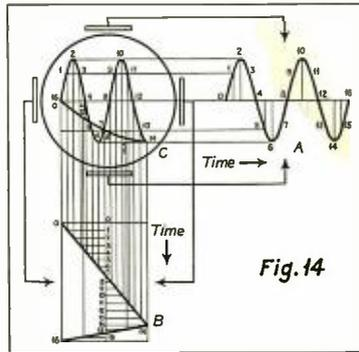
Frequency ratio 1:2 voltages A and B in phase: This shows a sine-wave voltage A applied to the vertical deflecting plates and a saw-tooth wave B applied to the horizontal deflecting plates. Wave B is linear from 0 to 14; hence, on the pattern C, the sine wave A appears undistorted. During the interval 14 to 16, the trace returns to the starting point 16.
