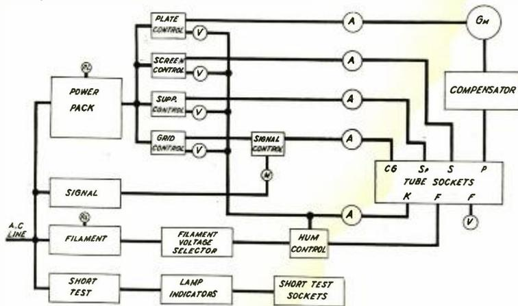
Fig. 2. Block diagram of the vacuum-tube analyzing equipment.
