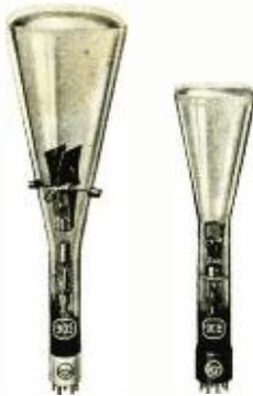
Fig. 1. The 905 and 906 cathode-ray tubes, showing comparative sizes.
