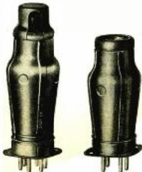
the base. The half shields are then pressed together near the top and the cap snapped on. The shoulder of the bulb acts as a pivot and the halves are forced outward at the bottom, tightening the shield in the base.
