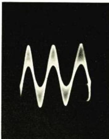
Fig. 25. A 50,000-cycle carrier modulated 50% at 400 cycles with timing axis oscillator set to 16,600 cycles.
