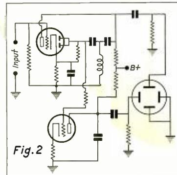
Circuit of high-pass filter, rectifier and amplifier.
