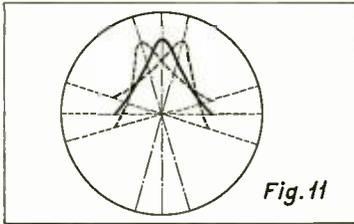
Heavy line indicates image when tube is adjusted correctly in socket. Dotted lines indicate possibilities if adjustable socket is not used.
