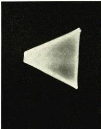
Fig. 23. Trapezoid of carrier with 75% modulation.
