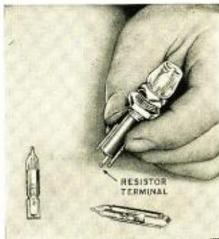
Dead front panel-type mountings, having clear phenolic resin caps, are available. A limiting resistor is used on all neon lamps and, in this case, is built into the mounting. For circuits requiring no resistor (such as oscillators, r-f indication, etc.) a direct terminal is provided. These units are designed especially for small space requirements. The manufacturer is Littelfuse Labs., 4507 Ravenswood Ave., Chicago. Descriptive folder on request.
