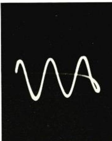
Fig. 26. A 50,000-cycle unmodulated carrier, illustrating the range of the timing axis oscillator.
