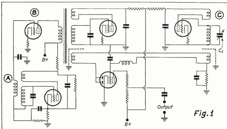
Abbreviated diagram of the oscillator unit.
