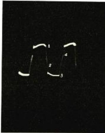
**Fig. 19.** Waveform of properly adjusted auto vibrator.
