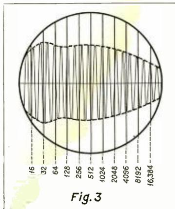
Face on oscilloscope screen for an amplifier passing full a-f range.
