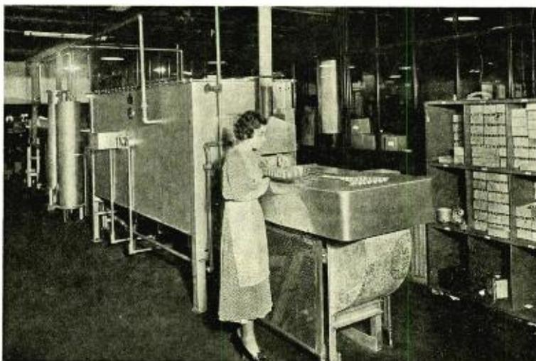
Mesh-belt conveyor-type furnace, 41 kw, for copper-brazing and firing metal-tube parts. Belt 8 inches wide, door opening 6 inches high, heating chamber 7 feet long, cooling chamber 18 feet long.
