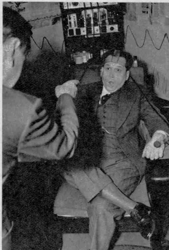
To record the "brain waves," or electrical nerve-impulses set up by fear—the emotion recorded by the psycho-detectometer, electrodes are clamped to hands and at the base of the brain. Some "lie detectors" are based on blood-pressure, perspiration, other reaction indicators
