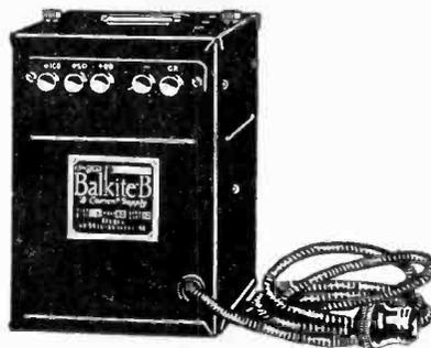
Trade Name—"Balkite B"; Type—Electrolytic; operates from 110-120 volts, 60 cycles, A.C.; also made for 50 cycles; delivers current of 40 milliamperes at 90 volts, with taps for varying output to meet requirements of various sets; replaces "B" battery; Material of Case—Terne plate, enameled; Dim.—7¼ x 6 x 9 in. high; Weight—10 lbs.; Price—\$55.00.
