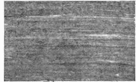
It is very easy to work, can be drilled, sawed, threaded, engraved or stamped without chipping or cracking. It will take a wood screw without drilling. Its surface is glossy and has the general appearance of highly polished hard wood. It is furnished in black, red and brown mahogany.
