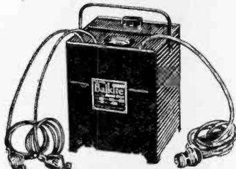
Trade Name—"Balkite"; Type—Electrolytic; operates from 110-120 volts A.C., 60 cycle; also made for 50 cycle; Charging Rate—2½ to 3 amperes, 6 volts; Material of Case—Terne plate, enameled; Dim.—6 x 6½ x 9 inches high; Weight—14 lbs.; Price—\$19.50.
