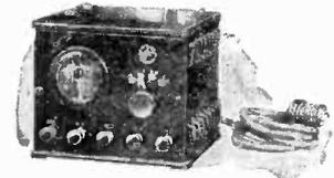
Trade Name—"Radel"; Type—Resistance; operates from 32 volts, D.C.; delivers current at 2, 4, 6 or 12 volts for "A" batteries and 24 volts for "B" batteries; Equipment—Ammeter; Material of Case—Metal, enameled, bakelite panel; Dim.—6 x 6¾ x 6 inches high; Weight—15 lbs.; Price—\$14.50.
