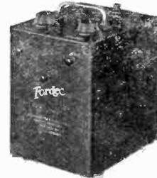
Trade Name—"Fordec"; Type—Bulb rectifier with filter circuit; uses two rectifying bulbs to rectify both sides of wave; operates from 110 volts, 60 cycles, A. C.; delivers 0-45 volts for the detector, 0-140 volts for the amplifiers; maximum current, 75 milliamperes; replaces "B" battery; Material of Case—Metal; Dim.—5½ x 8 x 6 in. high; Weight—9½ lbs.; Price—\$38.50.
