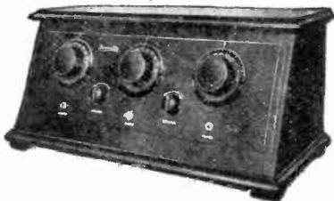
Trade Name—"Champion Five"; Type—Tuned Radio Frequency; Tubes—5; Battery—"A" Storage or Dry, "B" 90 Volts; Controls—4; Tuning, 3; Tube, 5; Antenna—Indoor or Outdoor; Dim.—7 x 8 x 21; Wt.—30 lbs.; Style—Slope Panel; Price—\$65.00.
