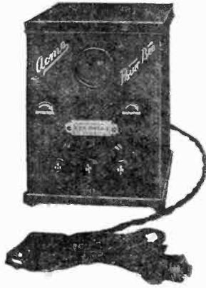
Trade Name—"Power Bee"; Type—Bulb; Operates from 105-120 volts, 60 cycles, A.C.; replaces "B" Battery; delivers current at 0 to 45 volts for detector, and 0 to 130 volts for amplifiers; Material of Case—Metal, enameled; Dim.—4½ x 8 x 7½ in. high; Price—\$27.50.
