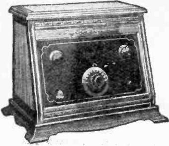
Trade Name—"Mohawk"; Type—Tuned Radio Frequency; Tubes—5; Battery—"A" Storage; "B" 90 Volts; Controls—Tuning, 1; Tube, 2; Dim.—21½ x 16¼ x 14¼; Wt.—30 lbs.; Price—\$150.00.
