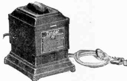
Trade Name—"Tungar"; Type—Bulb; operates from 115 volts, A.C., 25 to 60 cycle; Charging Rate—6 volts, with attachments for 2 and 4 volts; charges "A," with attachments for charging "B" battery; Price—60 cycles, \$18.00; other frequencies up to \$28.00.
