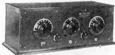
Type—Tuned Radio Frequency; Tubes—5; Battery—"A" Storage; "B" 90 Volts; Controls—Tuning, 3; Tube, 3; Dim.—7 x 21 x 7; Price—\$90.00.
