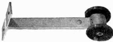
It consists of a brown porcelain insulator of spool shape held in a pressed steel holder formed to permit fastening to any convenient surface by means of nails or screws. The device is rust-proofed by the Udylite process.
