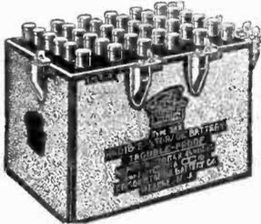
Type—"B" (nickel-iron elements in alkaline solution); Capacity—2500 M.A.H.; Voltage—22½; Material of Case—Molded composition; Finish—Black; Dim.—4¼ x 7¼ x 6½; Price—\$13.60; also 45 volt, Dim. 7¼ x 10 x 6¾, \$24.75 (equipped with Fahnestock clips).
