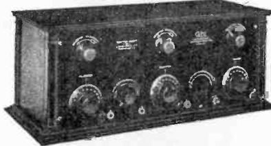
Trade Name—"Coto Symphonic"; Type—Tuned Radio Frequency; Style—Portable; Tubes—4; Battery—"A" Dry; "B" 90 Volts; Controls—Tuning, 2; Tube, 4; Price—\$125.00.
