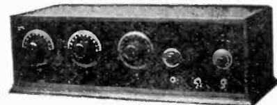
Trade Name—"Concert Grand"; Type—Tuned Radio Frequency; Tubes—4; Battery—"A" Storage; "B" 90 Volts; Controls—Tuning, 3; Tube,
