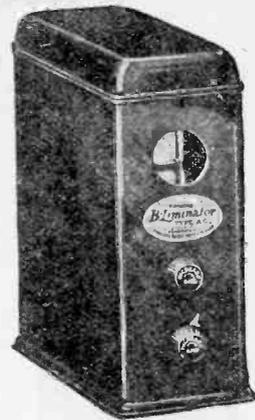
Trade Name—"B-Liminator"; Type—Bulb; operates from 110 volts; 60 cycles, A.C.; delivers current of 25 milliamperes (maximum), 120 (maximum); replaces "B" battery; Material of Case—Metal; Dim.—3 x 7 x 8¼ in. high; Weight—6½ lbs; Price—\$35.00.
