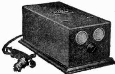
Trade Name—"Rectodyne"; Type—Bulb rectifier with filter circuit; uses two tubes (type 201A) to rectify both sides of wave; replaces "B" battery; operates from 110 volts, A.C.; Dim.—6¼ x 12 x 5 in. high; Price—\$44.00, less tubes. Also made in resistance type with filter circuit; operates from D.C.; replaces "B" battery; Price—\$32.50.
