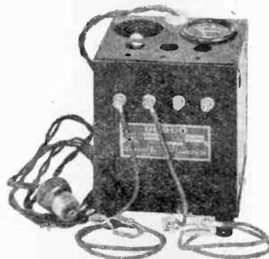
Trade Name—"Delco Jr."; Type—Bulb; operates on 60 cycle, A.C.; Charging Rate—4 amperes, 6 volts; 250-750 milliamperes, 96 volts; charges "B" battery; Material of Case—Zinc; black enamel; Weight—8 lbs.; Price—\$18.50.
