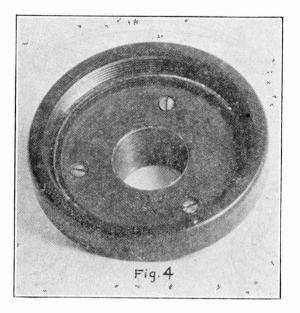
the screw heads will be flush with the cap (Fig. 4). If you are unable to make this cap, there is a cap on the market made for attaching a receiver to a phonograph that sells for a reasonable price. The horn can be made of paper but copper makes a much better job and kicks out more
