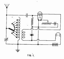
The strength of signals is not proportional to the voltage applied to the grid, but to the square of the applied grid-voltage, and it follows that if the initial voltage of the signals can be doubled by the use of coupled circuits, the resulting signal strength will be four times that available when the grid is connected to the aerial circuit.
