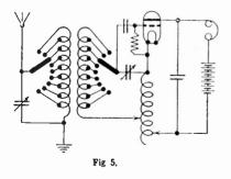
to couple the grid and plate circuits (Fig. 5). This inductance which is connected at one end to
