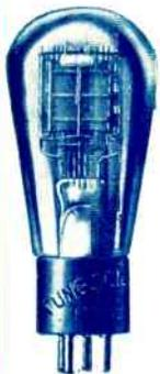
Pentodes are approximately four times as sensitive as type 245 power tube. In addition, they are capable of handling a much higher power output without distortion.
