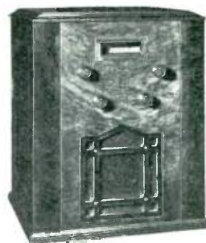
MODEL 376BT —5 tube plus ballast tube improved battery superheterodyne console radio. Range, full standard broadcast band—540 to 1,600 Kilocycles. Operates either on air cell, dry cell or 2-volt storage battery. Cabinet is of figured walnut veneers and American hardwood. Cabinet holds all batteries when dry cell type is used. Less batteries, $44.50
