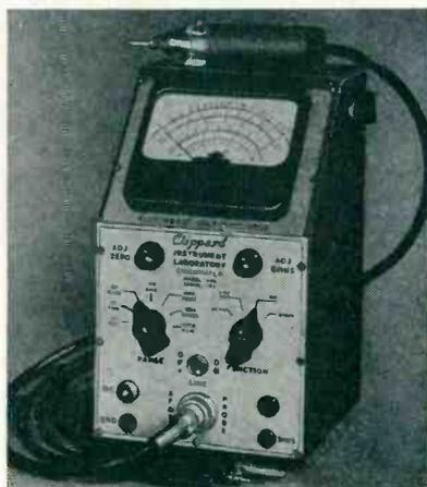
guaranteed in field, its input impedance is less than 7 mmfds., 7 megohms A.C., 28 megohms D.C., assuring minimum circuit disturbances. Please mention **RADIO & APPLIANCE JOURNAL**, Oct., 1947, when writing to manufacturer.
