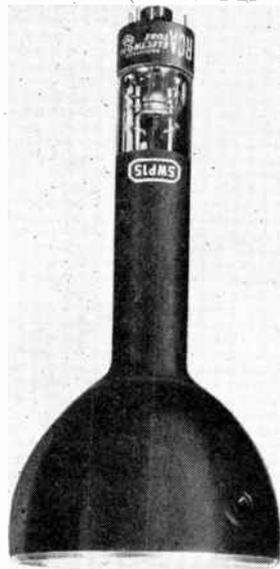
This new Flying-Spot tube furnishes a small, rapidly moving spot of radiant energy for scanning a slide transparency or opaque object. It thus makes possible a relatively simple and inexpensive video-signal generator capable of producing not only a repetitive picture signal like the monoscope, but also of permitting change of picture at will and of reproducing the picture with the halftone fidelity of photographic film.
