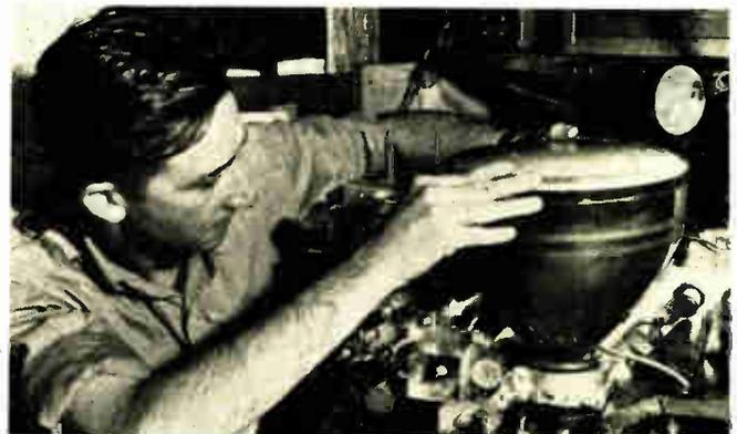
During brief sojourn chassis gets finishing touch with insertion of 10-inch cathode-ray tube and alignment of IF-RF.
