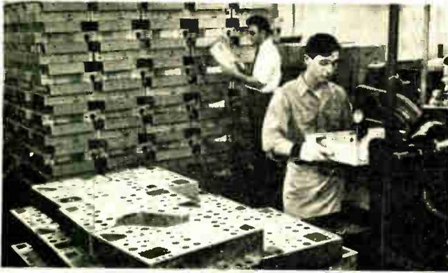
Joining sockets, terminal boards, and condenser wafers to chassis on rivet press. Inspector in rear examines each.
