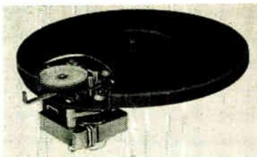
Model DM. above, is a compact GI Smooth Power, low-cost, dual-speed phonomotor with external speed change control. Approximately same size as present speed turntable motors. By shifting speed change lever, which extends beyond turntable rim, novel neoprene, belt-driven step pulley is engaged or disengaged to change speed.
