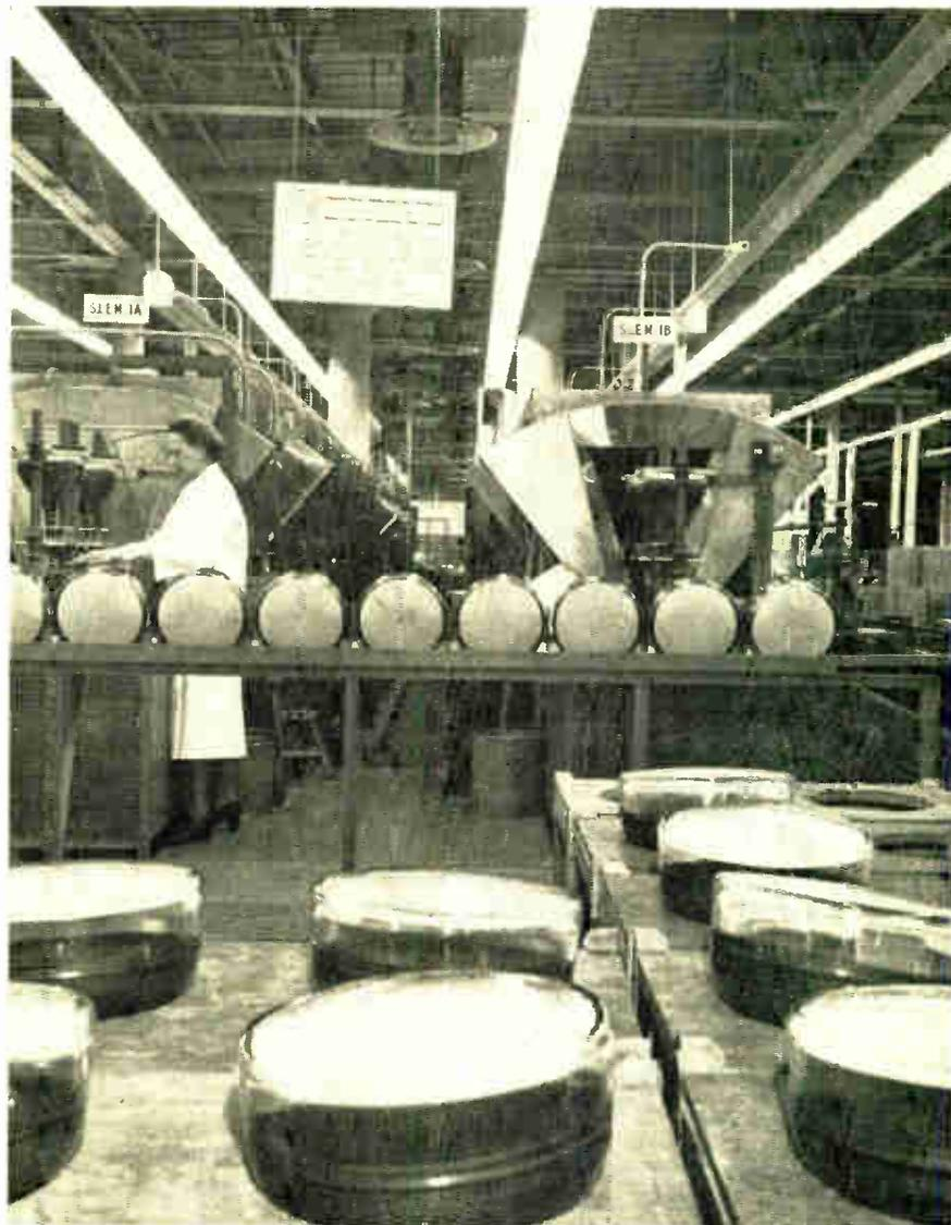
*Tubes, above, being placed on exhaust machine. They are given vacuum ten times that of ordinary radio tube, sealed, and passed by conveyor belt to next stage. Below, testing cathode-ray tube. Tubes must test on all FCC-assigned channels.*
