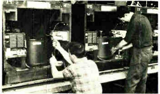
*Workers are making final adjustments on components before consoles move into cabinet-finishing department.*
