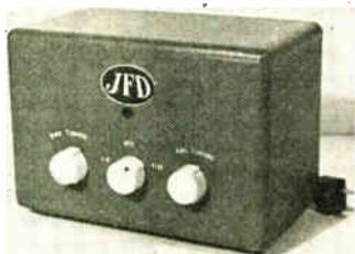
For fringe and remote areas where TV signals are weak, this booster is designed to tune in distant stations and tune out noise and ghosts. Six mc. bandwidth, individual circuits and tubes for upper and lower bands, and separate tuning for upper and lower band circuits. Matches all receivers and antennas. Cabinet in simulated leather available in walnut, mahogany or blonde finishes.
