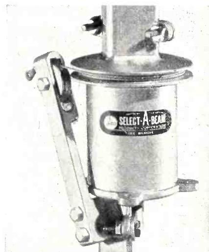
Of aluminum construction and with weather-sealed ball bearing working parts, this TV antenna rotator is operated through a worm-gear control box attached to the outside of the house. Turns antenna 360 degrees. Positions lock automatically, and metering device provides easy and speedy selection of chosen stations.
