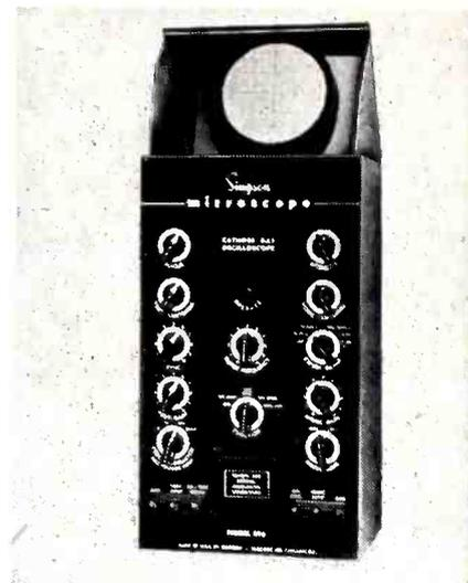
For saving space on the testing bench, this new type oscilloscope has the 5-inch cathode-ray tube mounted in a vertical position. Cathode-ray image is reflected from mirror in adjustable cover at cabinet top, bringing viewing surface near eye level. Mirror and wing sides fold into cabinet when not in use. Priced at \$179.50.
