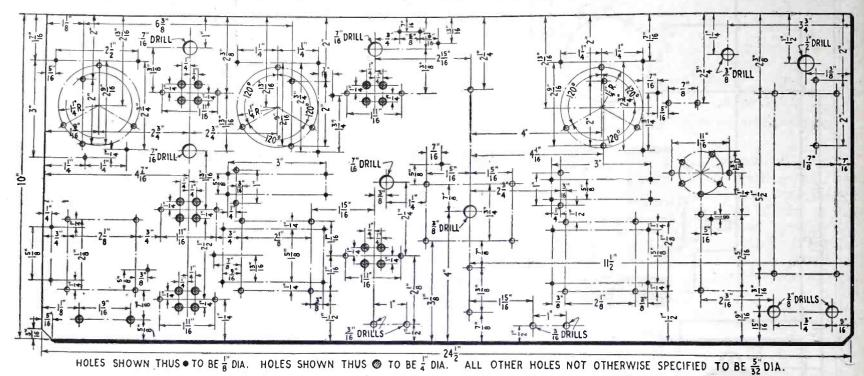
Drilling layout for the sub-panel of the Supreme A. C. Six Receiver.
