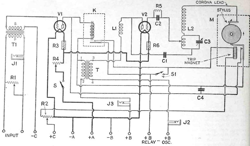
Schematic wiring diagram of the radio picture apparatus described in the article.
