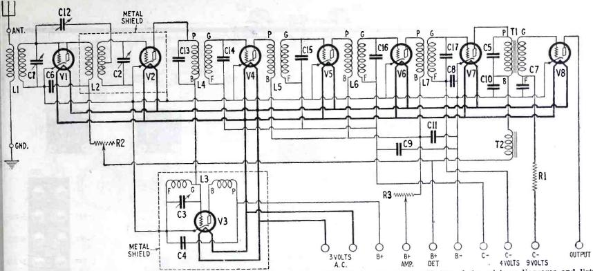
Schematic wiring diagram of the Ultradyne A. C. Commander. All parts are indicated to correspond with the photos picture diagrams and list of parts for the set.
