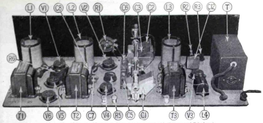
All parts are lettered to correspond with diagrams and list of parts. A rear view of the net.
