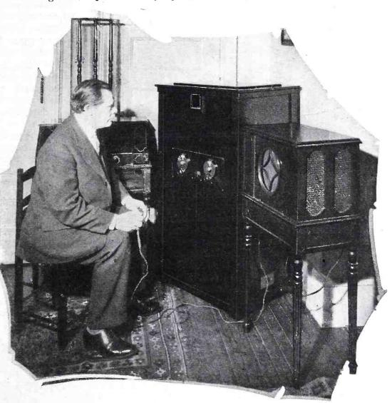
Dr. Alexanderson is shown here tuning the television receiver: the image is seen through the small square opening on a level with the operator's eyes. Notice the broadcast receiver and loud speaker.
