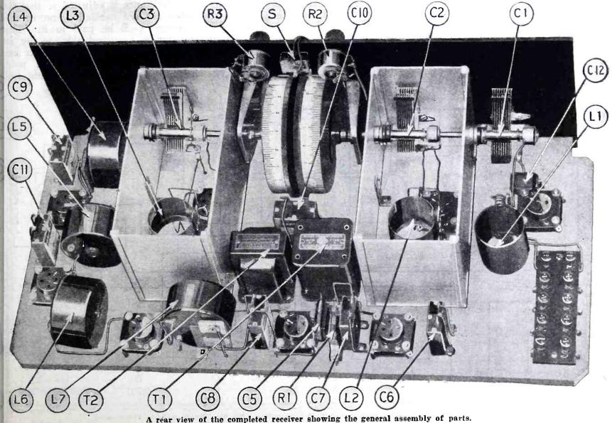
view of the completed receiver showing the general assembly of parts.
