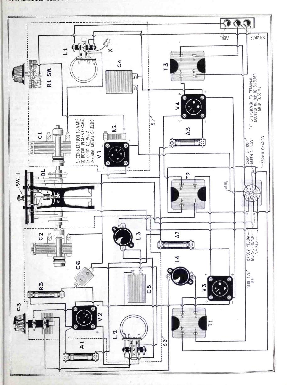
cipally to the fact that the 201A-type tube must be operated with a positive bias on the grid to secure efficient rectification in the grid circuit (that is; with a condenser-leak arrangement). This positive bias is obtained by connecting the leak (R3) to the positive A filament terminal. Under these conditions the grid attracts electrons and this greatly decreases the grid-to-filament resistance, resulting in loss of sensitivity and selectivity.
