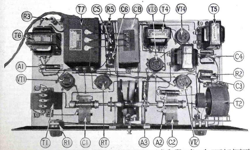
How the set appears looking down on the baseboard from top. Note that complete parts for the "B" supply are also mounted on baseboard.
