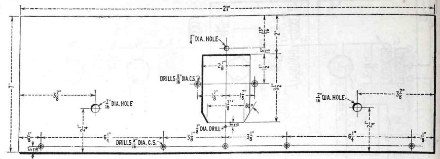
The drilling details for the front panel of the four-tube, screen-grid receiver, illustrated in the photos with this article.
