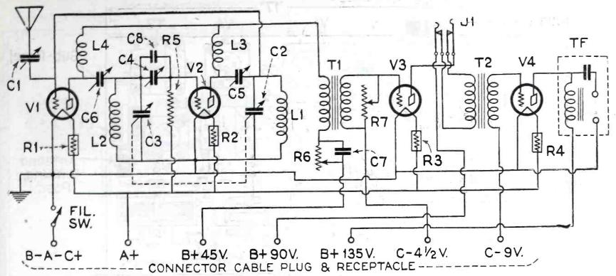
Schematic diagram of the Adventurer Four receiver. Variable condensers C2 and C3 are operated on the single control drum dial.
