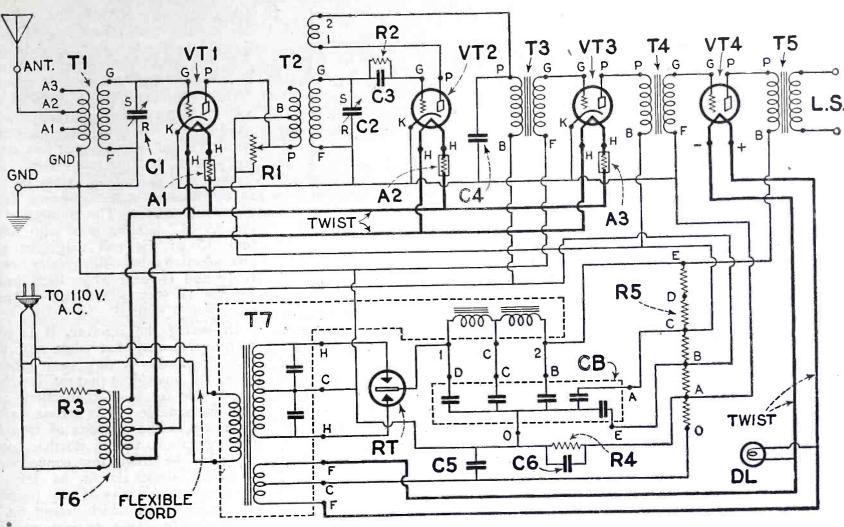
Schematic wiring diagram of the Four-Tube Roberts A. C. Receiver is shown directly above.
