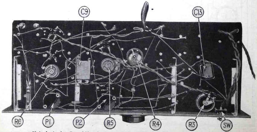
Photo showing how the variable resistances, condensers and Phasatrols are mounted beneath the sub-panel.
