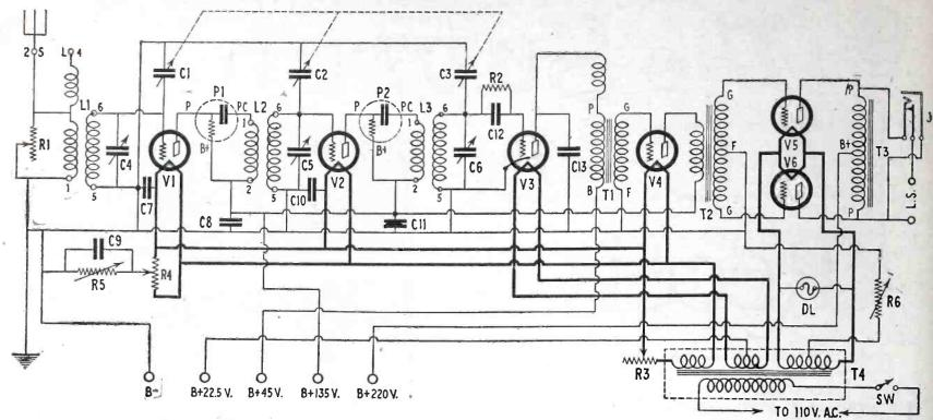
Schematic wiring diagram of the set. Variable condensers, C1, C2 and C3 operate on the one shaft, making the set uni-controlled.
