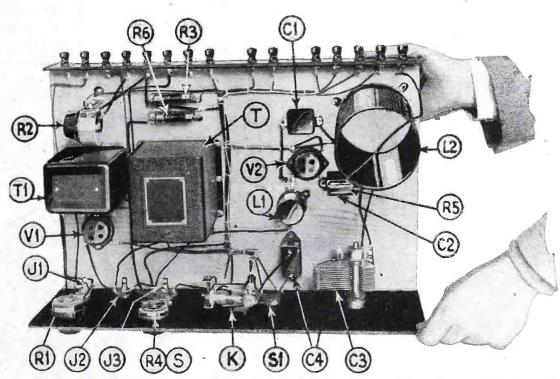
This photo shows a top view of the radio picture receiver. All parts are indicated to correspond with components listed in the text of this article.
