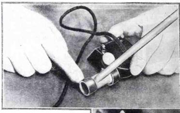
Two photos showing a close-up of the arm piece and method of mounting.
