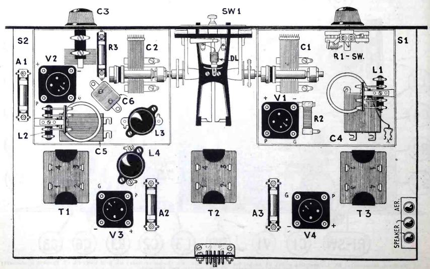
Instrument layout of the set showing the location of all parts. Letter symbols correspond with diagrams, photos and list of parts.
