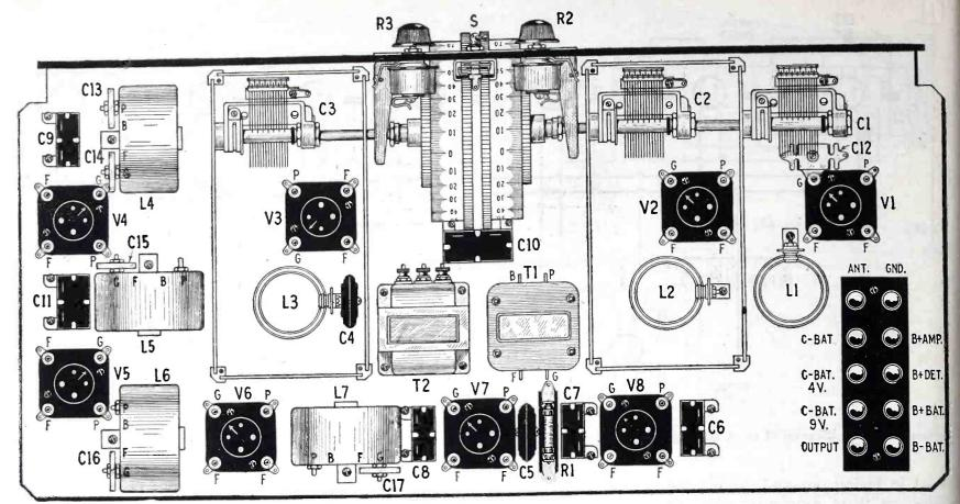
The above layout shows how all parts are mounted on the baseboard and panel. Note the method of mounting the variable condensers on the walls of the aluminum shields.
