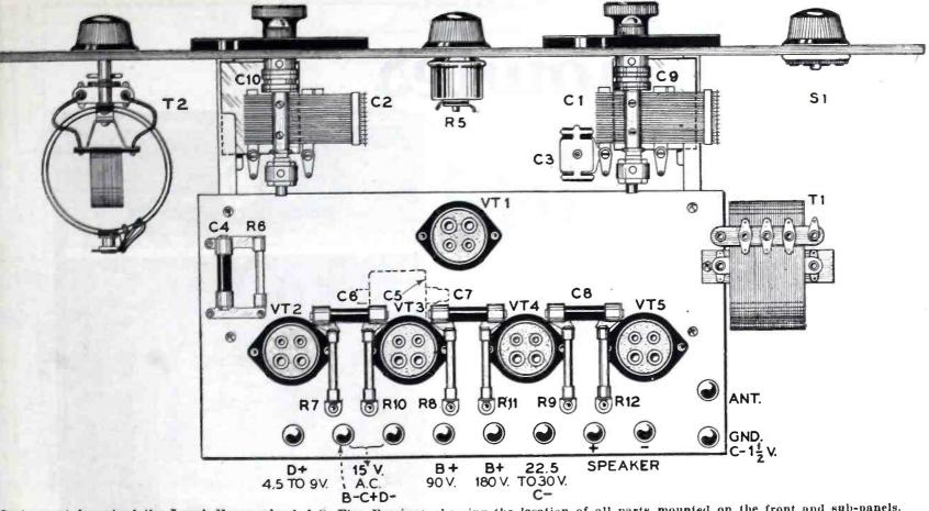
Instrument layout of the Lynch-Hammarlund A.C. Five Receiver, showing the location of all parts mounted on the front and sub-panels.
