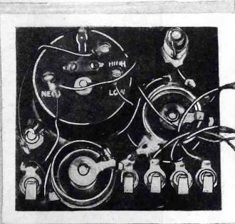
outfit is also shown. This light has a colored glass front with the small electric bulb placed in an upright position in back of it. A testing device of this nature is particularly helpful to the builder while making tests of a receiver on the work bench, since it is possible to immediately ascertain which circuit is faulty or incomplete. The testing outfit is also valuable in determining wheth-
