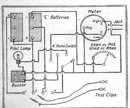
Wiring diagram of the testing set.
