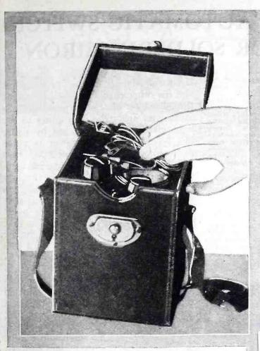
The photos on this p a g e show various details of the radio test set. At the left is complete test set with test cords placed in the top of the camera carrying case. At the r i g h t shows how the two "C" batteries a replaced in the bottom of the carrying case. The three photos directly below show a rear view of the panel, and the l o w e r right h and p h o to indicates the location of the small pilot
