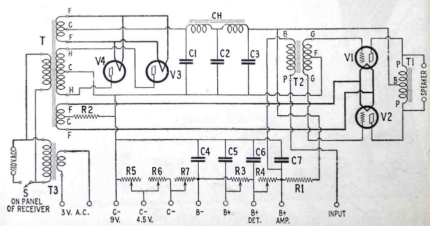
Schematic diagram of the power unit employed in conjunction with the Ultradyne A. C. Commander.
