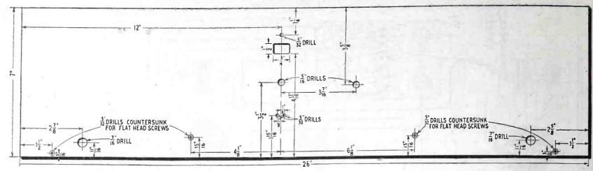
Directly above is the layout for drilling the front panel.
