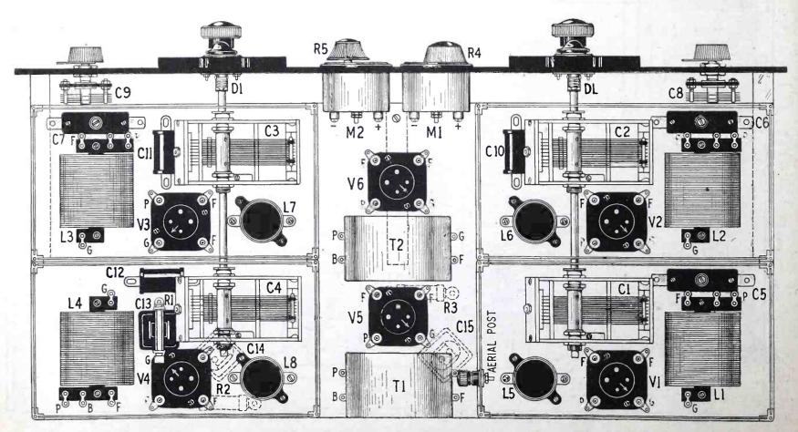
Instrument layout of the receiver indicating the exact location of all components. Parts mounted beneath the sub-panel are shown in dotted lines.
