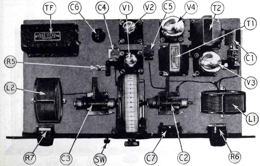
A top view of the set. The best part of the wiring is beneath the baseboard. Holes are drilled in the baseboard close to the terminal of parts and wires are passed through the board to the underneath side.
