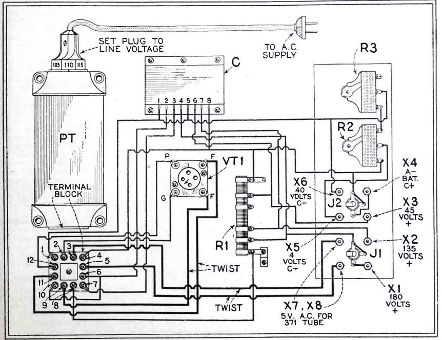
Picture wiring diagram of the power unit employed in conjunction with the Cosmopolitan Screen-Grid Receiver.
