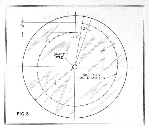
Layout of holes in the revolving disc.
