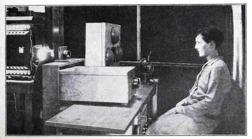
Above shows the relative position of the apparatus used in transmitting by radio. The grouping of the photoelectric cells is shown, three being visible and a fourth behind the amplifier boxes. Note the microphone at the right and the lines of light and shadow on the girl's face.
