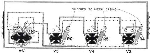
Wiring diagram of the top and under side of the long-wave shielded time amplifier, S3. V3, V4 and V5 are screen-grid tubes. This amplifier is available only as a complete, ready-wired unit. Its wiring is shown as a matter of technical interest.
