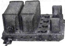
Type PAM 17 is for and supplies field current to dynamic type speakers.
