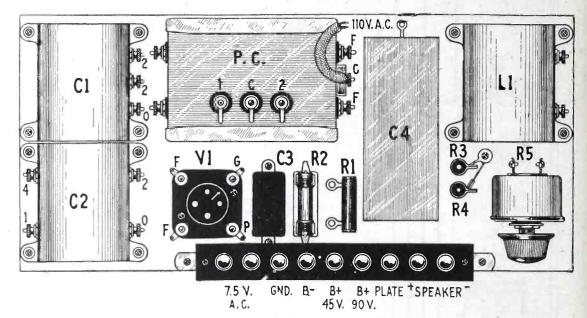
Layout of parts for the power unit employed in conjunction with the Hagerman 210-A.C. Six Receiver. Parts are indicated in symbols to correspond with diagrams.
