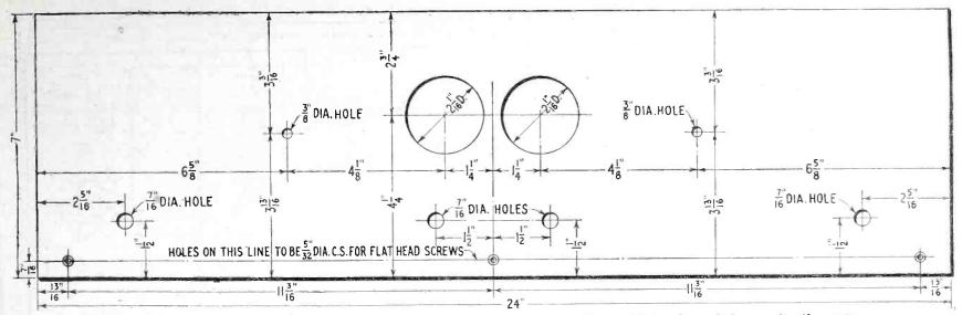
Front panel layout for the receiver giving all dimensions for holes to be drilled. The two large holes are for the meters.
