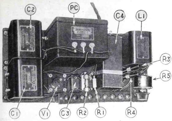
Photo of the power unit. All parts are indicated to correspond with wiring diagrams.
