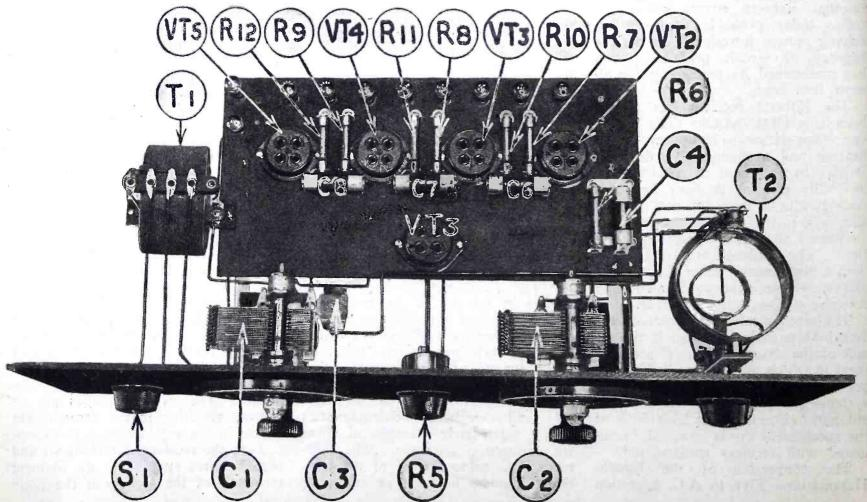
A top view of the set showing all parts mounted on the "deck" and front panel. The Clarostat, R5 is mounted directly in the center of the front panel and is connected in the antenna circuit of the set as shown in the diagrams accompanying this article.
