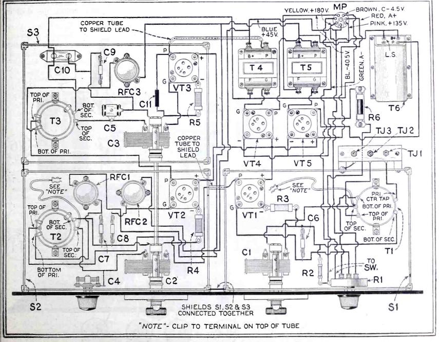
Picture wiring diagram of the Cosmopolitan Screen-Grid Receiver.
