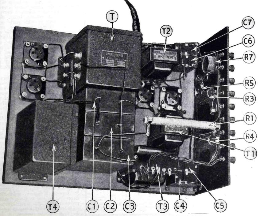
A photographic view of the power unit showing the layout of parts and wiring.
