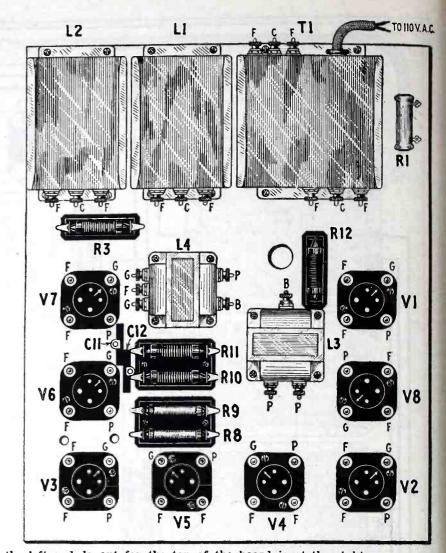
Layout for parts on the bottom of the board is shown at the left and layout for the top of the board is at the right.
