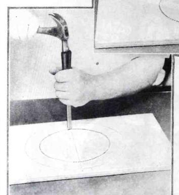
How the hole in the baffle is drilled and cut out.
