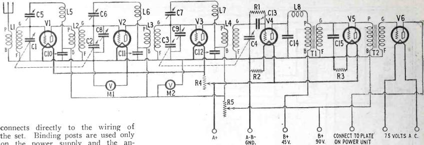
Schematic wiring diagram of the six tube A.C. operated receiver described herewith. Variable condensers C1 and C2 are operated on one shaft and condensers C3 and C4 on another shaft.
