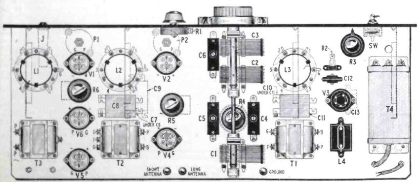
Layout indicating the exact location of all parts. Instruments shown in dotted lines are mounted beneath the sub-panel.
