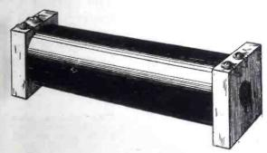
A microphone transformer (modulation transformer) specially designed for use with the Skinderviken Transmitter. These transformers are used for stepping up the low voltage high-frequency currents from the transmitter circuit, to a slightly higher voltage which will permit transmission over greater distances. The coils have many other uses for experimenters, such as for making small medical coils, etc. Primary resistance 11/4 ohms.
