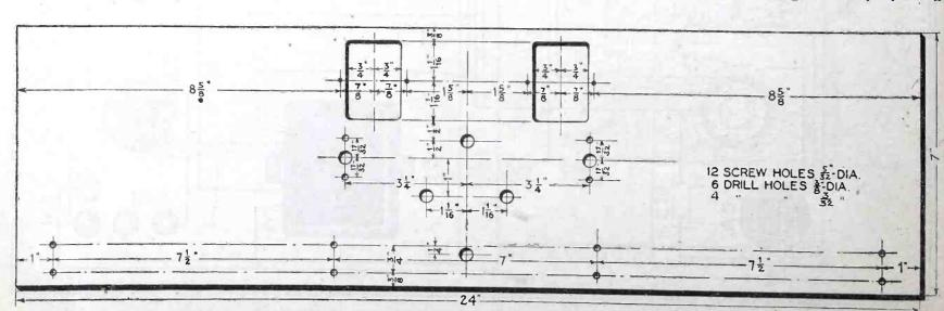
Drilling layout for the front panel of the Improved Screen-Grid Laboratory Super-Heterodyne.
