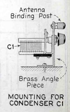
The above sketches show how parts are mounted under the baseboard and at the right shows the method of mounting variable condensers C1.
