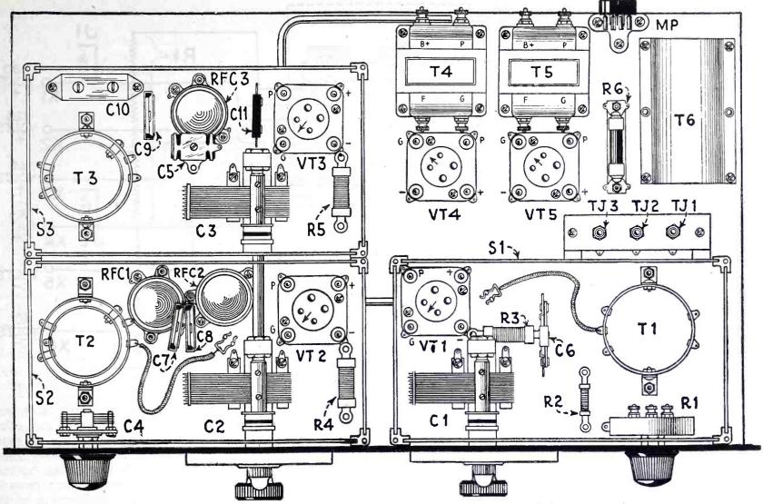
Instrument layout of the set showing the placement and position of all parts.
