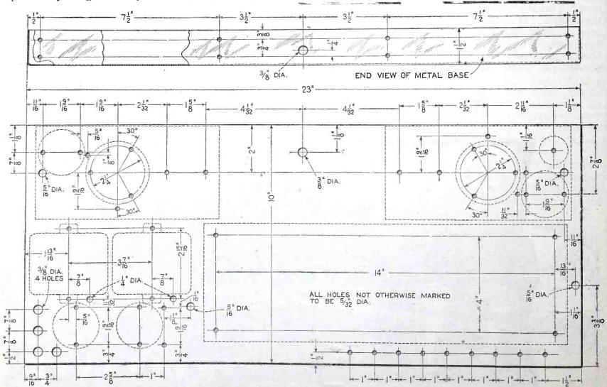
Drilling layout for the steel chassis as used for the Improved Screen-Grid Laboratory Model Super-Heterodyne. Dotted lines indicate location of apparatus to be mounted on the chassis.
