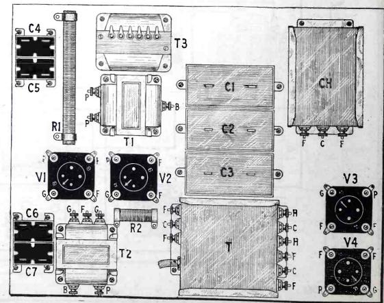
At the left shows how the variable resistors of the power unit are mounted on the panel while at the right shows the arrangement of parts on on the baseboard.
