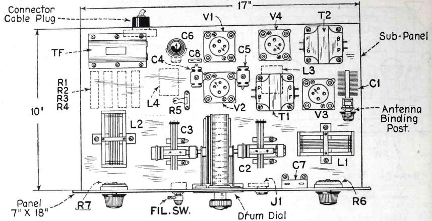
Instrument layout of the set. Parts to be mounted beneath the baseboard are indicated in dotted lines.
