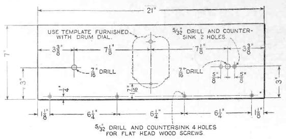
Dimensions for drilling the front panel of the Four-Tube Roberts A. C. Receiver.
