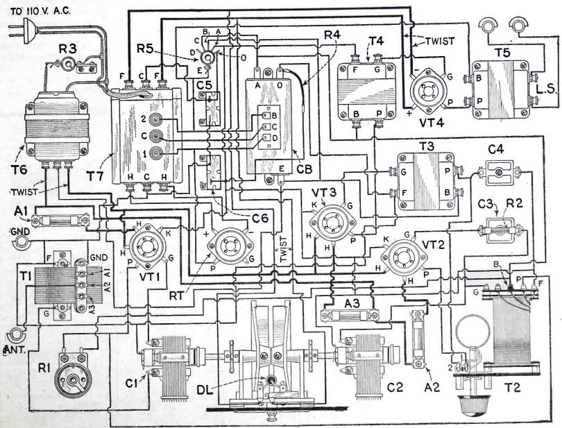
Picture wiring diagram for the Roberts A. C. set. All parts are indicated to correspond with references in the text, schematic diagram, photos, instrument layout and list of parts.
