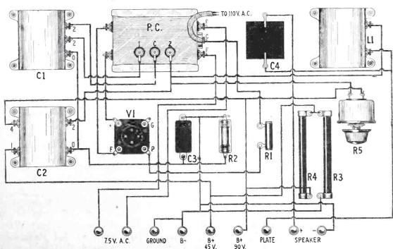
Picture wiring diagram of the Hagerman 210-A.C.-Six power unit.
