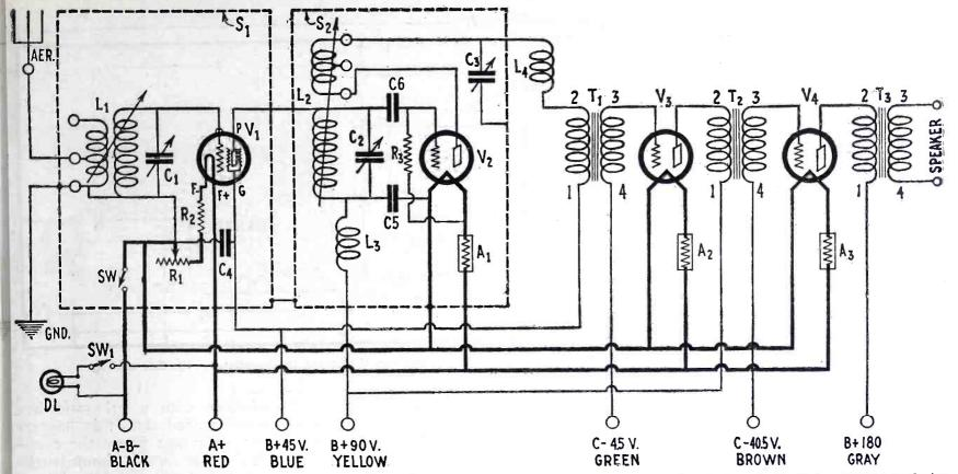
The schematic diagram of the Knowles screen-grid receiver described in the article herewith. The dotted lines indicate the shields enclosing R. F. portions of the circuit.
