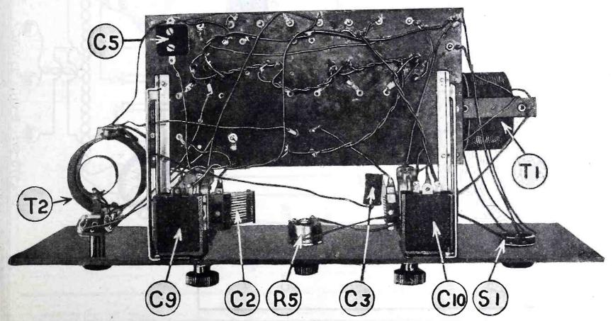
A bottom view of the set showing how the two by-pass condensers, C9 and C10 are mounted. Note the 15-volt A.C. leads are twisted.
