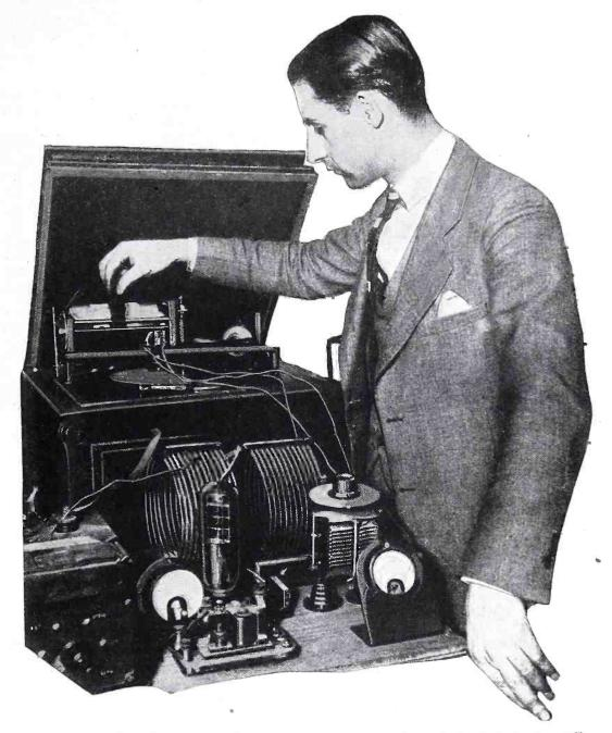
Above is the picture transmitter showing simplicity of equipment, hooked up to ordinary victrola. A short wave transmitter is used in conjunction with a photo pick-up device. Experimental tests are being conducted daily over a broadcast station in New York.
