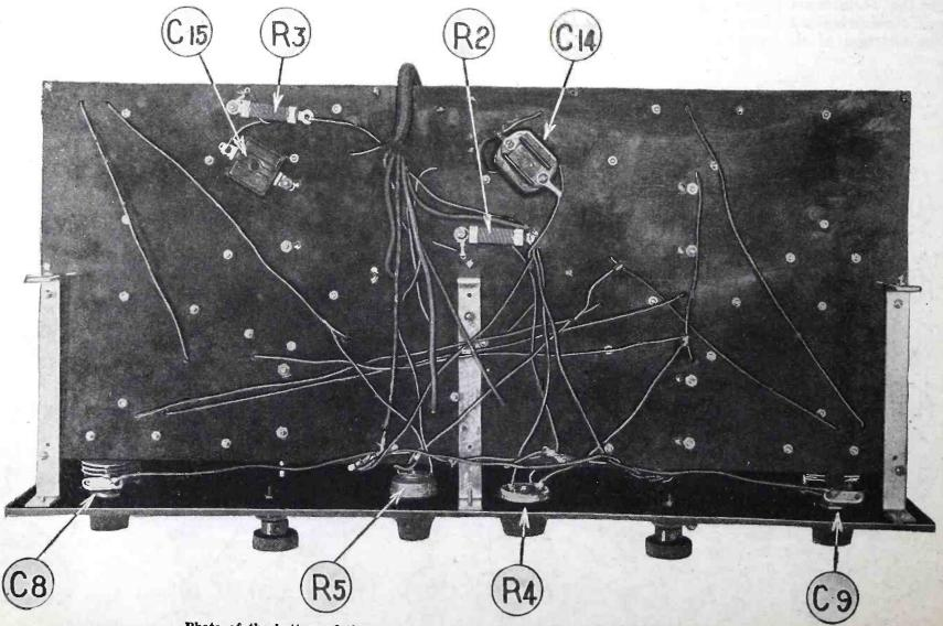
Photo of the bottom of the sub-panel showing condensers, fixed resistors and wiring.
