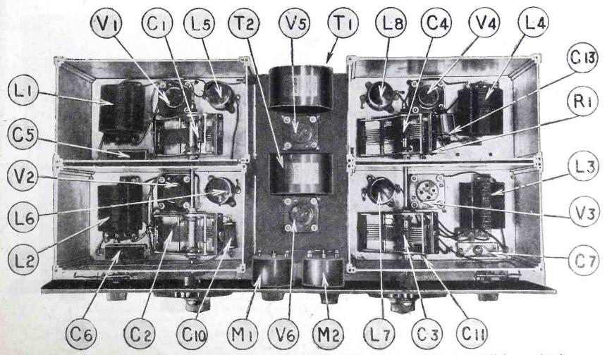
A top view of the Hagerman 210-A.C.-Six Receiver showing the arrangement of parts within the four shielded compartments.
