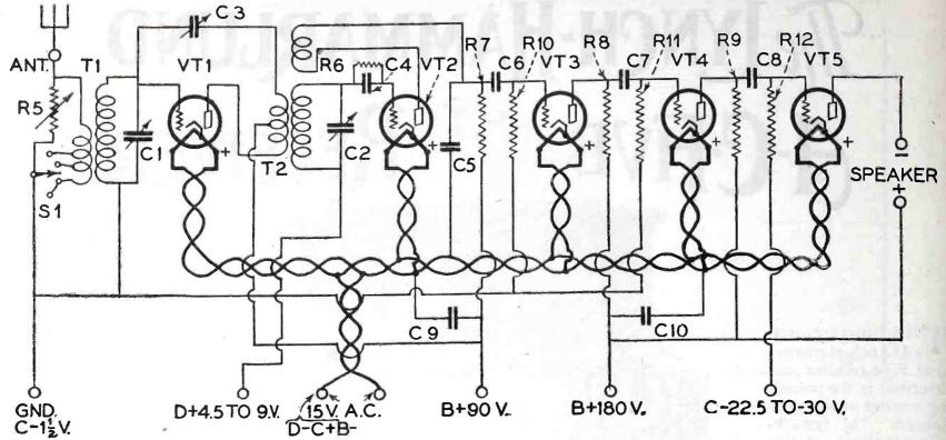
Above shows a schematic wiring diagram of the Lynch-Hammarlund set wired for A.C. operation. All parts of the circuit are indicated to correspond with photos, picture wiring diagram and list of parts.
