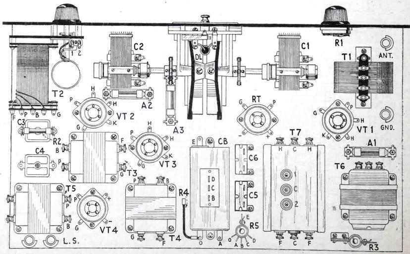
Instrument layout showing the placement of all parts on the baseboard and front panel.
