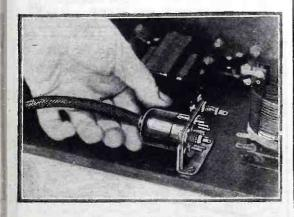
Mount the cable connector at right angles with the edge of the baseboard.
