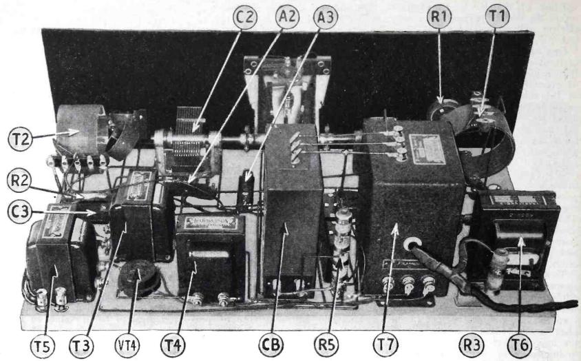
A rear view of the set showing the "B" supply condenser block, CB, power compact, T7, filament transformer, T6 and resistors, R3, R5, as well as other parts of the set.
