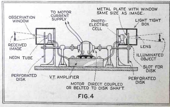
The experimental television apparatus can be arranged as shown above.
