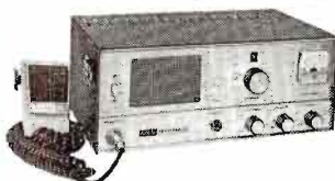
New Model 779 Sentinel 23 CB Transceiver. 23-channel frequency synthesizer provides crystal-controlled transmit and receive on all 23 channels. No additional crystals to buy ever! Features include dual conversion, illuminated S-RF meter, adjustable squelch and noise limiter, TVI filter, 117VAC and 12VDC transistorized dual power supply. Also serves as 3.5 watt P.A. system. $169.95 kit, $189.95 wired.
