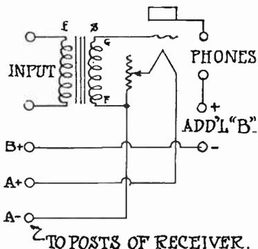
ment in results is not always obtained, though oftentimes the amplifier operates more quietly when the cores are connected in this manner. None of the usual amplifying transformers have binding posts for making a connection to the core. A connection may be obtained by loosening one of the bolts holding the core in place and slipping a wire under the head. Tightening up the bolt will then hold the core firmly, giving also a sufficiently good connection for the purpose desired.
