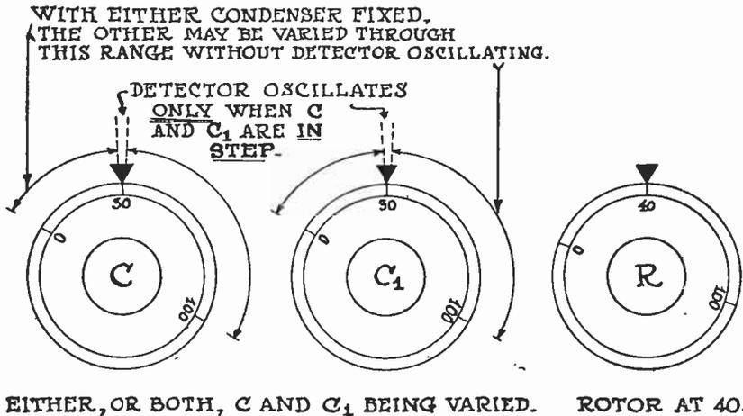
UNDER THESE CONDITIONS REDUCE ROTOR SETTING SLIGHTLY FOR BEST RESULTS.
