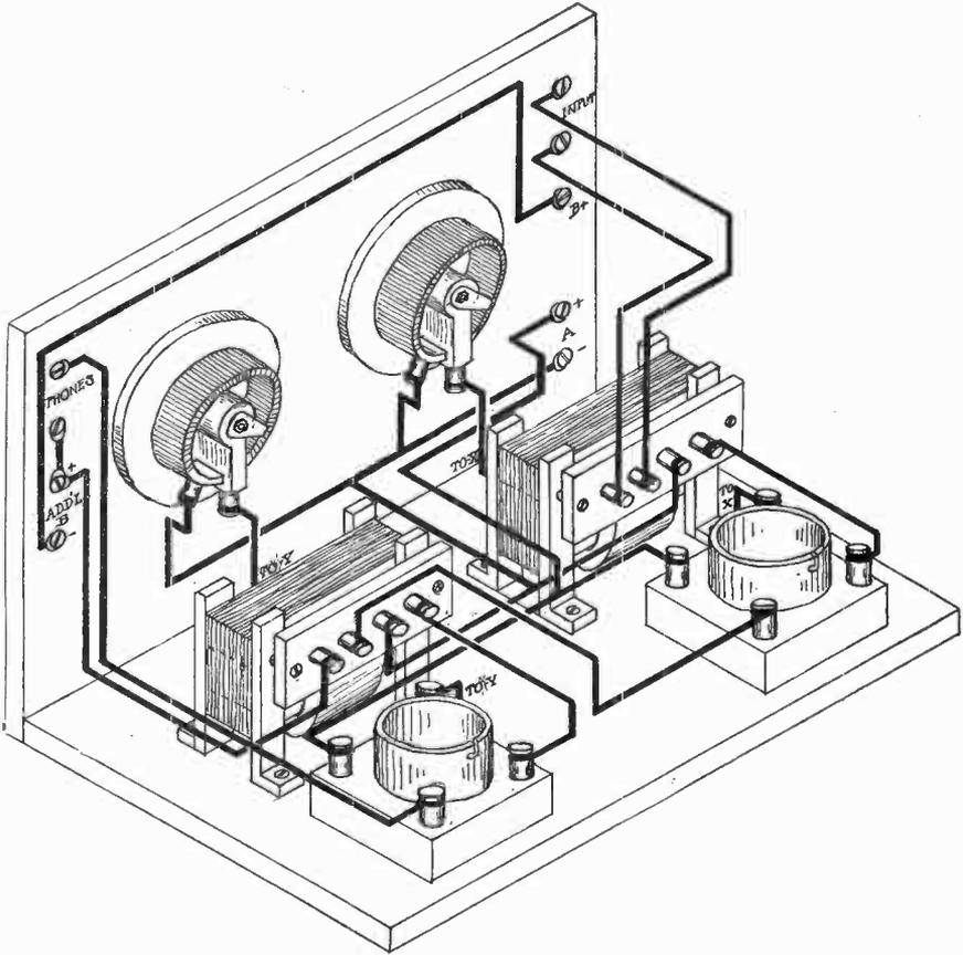
If two stages of audio-frequency amplification are desired, and may be constructed at the same time, this assembly drawing will serve as a guide in laying out the apparatus. This amplifier, as well as the one preceding, may be used with any type of receiving set. The special points given in the accompanying article should be carefully considered in constructing either of these amplifiers.
