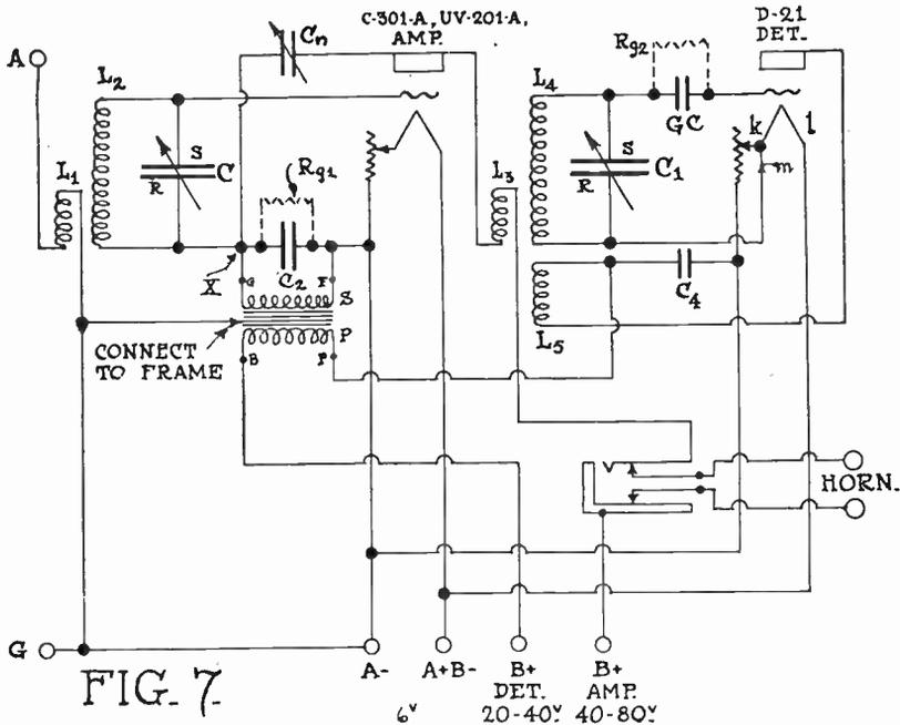
bus-wire secured to the bolts of the first condenser. These pieces of bus-wire are fastened to the coil form by means of a 6-32 brass machine screw  $\frac{3}{8}$  or  $\frac{1}{2}$  inch long, passed through the winding form. The variocoupler form automatically takes care of the mounting of the second transformer.
