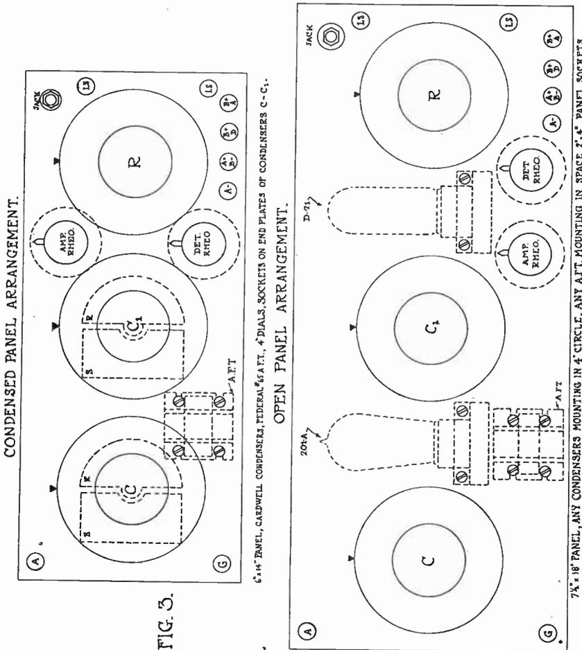
6" x 14" PANEL, CARDWELL CONDENSERS, FEDERAL 5/8" A.F.T., 4 DIALS, SOCKETS ON END PLATES OF CONDENSERS C-C1.
