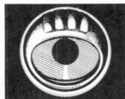
Fig. 3. Above is shown a tuning eye indicator or "Magic Eye" which facilitates in the proper tuning of not only domestic broadcasting stations but short-wave stations as well.
