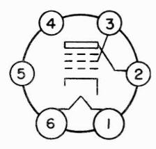
Fig. 6. Typical connection for 6-prong tubes, such as 6D6, 58, 2A5, 41, 42 from top of socket.
