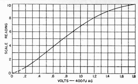
Fig. 2. Curve showing sensitivity of signal tracer, with input volts plotted against arbitrary units with which meter dial is calibrated.
