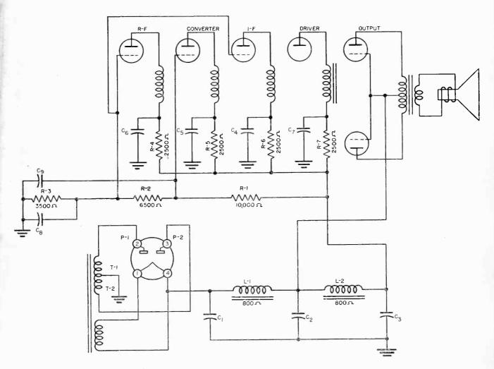
Fig. 3. D-C power distribution throughout 7-tube super-heterodyne.
