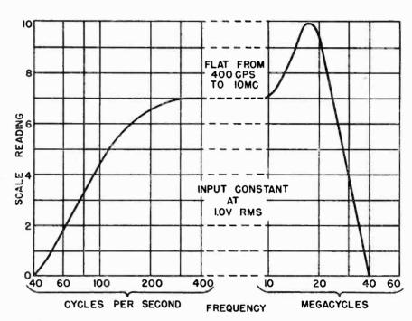
Fig. 3. Frequency response curve, flat over most useful range of frequencies, with reduction in sensitivity at low frequencies to reduce hum readings. Peak at 17 mc is caused by resonance in probe circuits.
