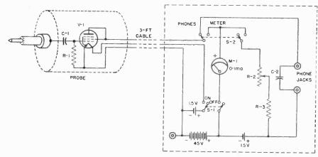
Fig. 1. Schematic of CA-11 Signal Tracer, applications of which are discussed in this article.
