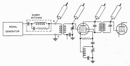
Fig. 4. Method of using tracer to follow passage of signal from stage to stage.
