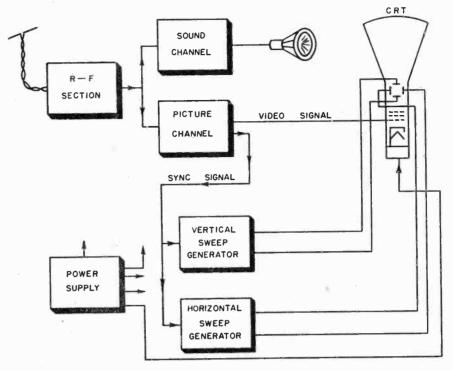
Fig. 2. Major sections of typical television receiver showing function of each portion of the circuit.
