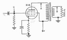
Fig. 5. Typical circuit of 6V6 output tube, used in determination of transformer impedance ratio and gain of the stage.
