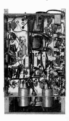
Bottom view of television receiver. Note the high voltage wiring.
