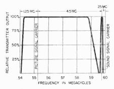
Fig. 1. Frequency division of typical television channel.
