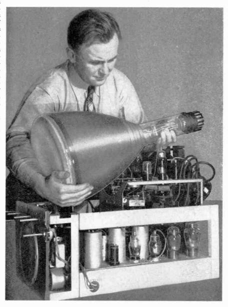
The author removing the cathode ray tube from a television receiver.
