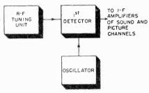
Fig. 5. R-F, first detector, and oscillator arrangement in R-F section of television receiver.
