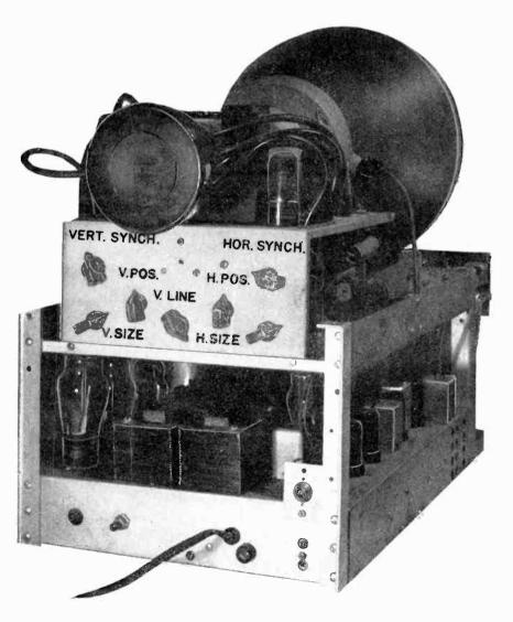
Rear view of a table model television receiver showing controls.
