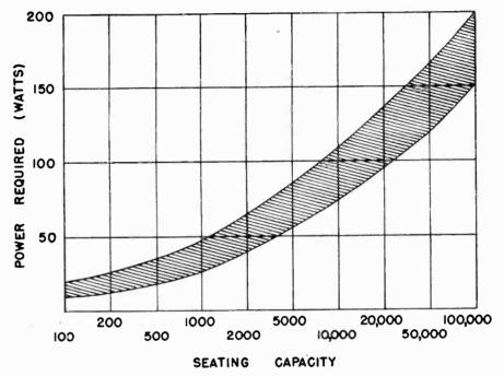
Fig. 1 Curve showing approximate power required for adequate coverage of audiences of various sizes. Upper limits of shaded area should be used for locations with high noise level, or where maximum fidelity of music reproduction is desired.
