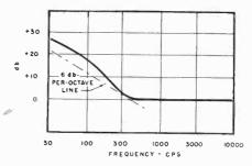
Fig. 2 Frequency response curve for network.
