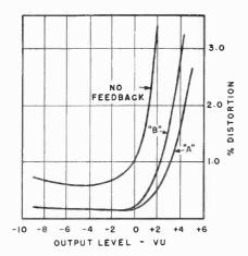
Fig. 6 Distortion curves for complete amplifier.
