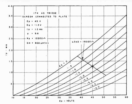
Fig. 3 Plate family for IT4 connected as a triode.
