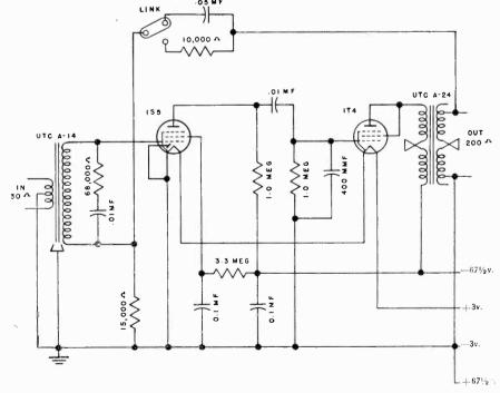
Fig. 4 Schematic of complete amplifier, equipped with link to provide flat or equalized operation of the amplifier.
