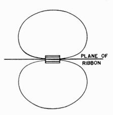
Fig. 4 Directivity curves for velocity or ribbon microphones.
