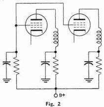
When trouble-shooting noisy receivers, a stage-by-stage elimination process is of great assistance. Starting from the output stage and working toward the input, short circuit the input of each stage. For example, if shorting the grid of the output stage stops the noise, and shorting the grid of the driver stage does not stop the noise, the noise must originate in the driver stage.
