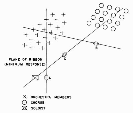
Fig. 3 Possible placement of microphones for chorus, singer, and orchestra to reduce pick-up of any section on other microphones.
