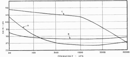
Fig. 5 Frequency response of amplifier under various conditions. Curve A represents equalized condition for phono reproduction; B is response with link on flat; C is response without equalization.
