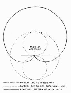
Fig. 5 Addition and subtraction of the sound energy received by the two sections of the uni-directional microphone produce the overall pattern known as a "cardinid"
