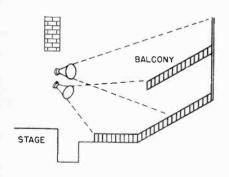
Fig. 7 Arrangement of loudspeakers for the most efficient coverage of orchestra and balcony seats in a theatre with using speakers with wide angles of distribution.
