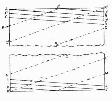
Fig. 7. Diagram of path followed by electron beam in scanning target of camera tube or screen of kinescope.
