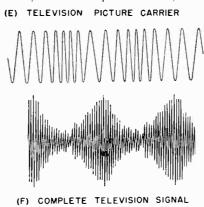
Fig. 10. Sound- and picture-modulated carrier signals.
