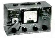
"VOMAX" is standard of comparison: D. C. volts; .05/3000 at 51 and 126 megohms
