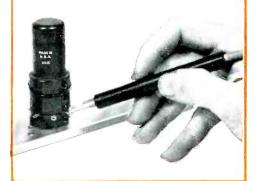
THIS BRAND-NEW INSTRUMENT (Type 167-B) is a low-cost answer to easy alignment of complex receivers. It has an extremely wide frequency range—generating fundamental signal voltages over six bands from 100 kc to 30 mc. Harmonics of the last band can be used for very-high-frequency testing.
