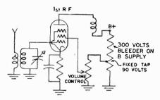
Fig. 6 Combination antenna shunt and C bias method of volume control.
