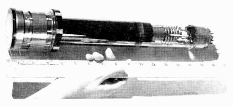
Fig. 5. The RCA Image Orthicon, a super-sensitive camera tube of recent development.
