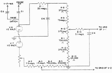
Fig. 7 Simplified diagram of the AC voltmeter input circuit.
