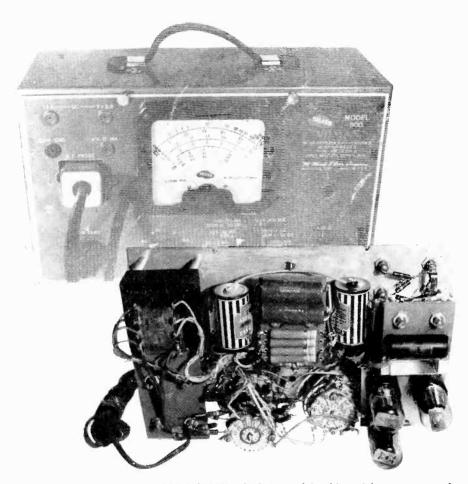
Fig. 2 The Silver Model 900 VOMAX which is used in this article as an example of the electronic volt-ohmmeter.
