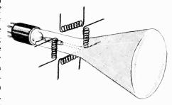
Fig. 8. Cathode ray tube showing position of deflecting coils.
