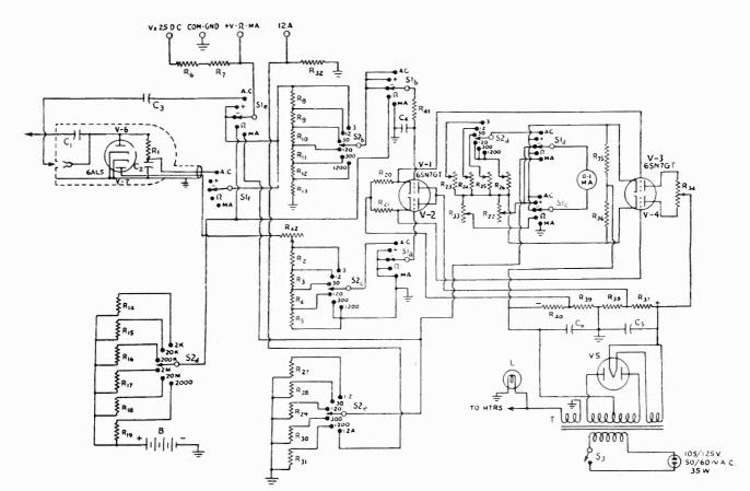
Fig. 5 The circuit used in the VOMAX.
