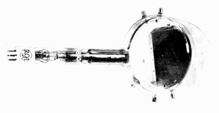
Fig. 3. An RCA Iconoscope (camera tube) of the large studio or professional type.
