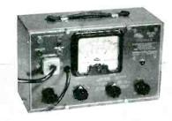
"VOMAX" is standard of comparison: • D. C. volts; .05/3000 at 51 and 126 megohms • A. C., a.f., r.f. volts; .05/1200 at 6.6 megohms • D. C.; .05 ma\_/12 amp. • Decibels; -10/+50 PLUS visual dynamic signal tracing.
