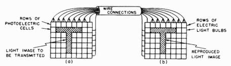
Fig. 1. Elements of the simplest television system. One similar to this is in use at Times Square, New York.
