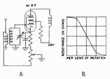
Fig. 7 Screen voltage method of controlling the output of a receiver.
