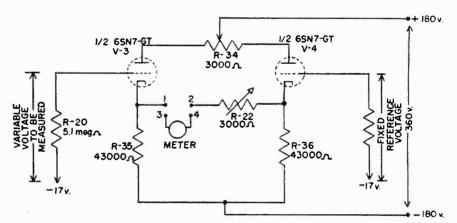
Fig. 6 Simplified diagram of the DC metering circuits.
