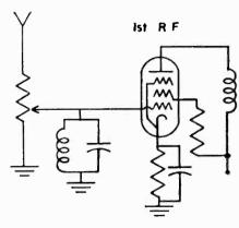
Fig. 5 Antenna shunt method of controlling the output of a receiver.
