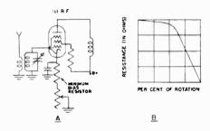
Fig. 4 Variable C bias method of controlling the output of a receiver.
