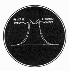
Fig. 8. Pattern obtained from a properly aligned discriminator using the method described in the text.
