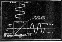
Fig. 5 When two sine wave voltages which are in phase are applied to the vertical and horizontal plates of a cathode-ray tube, the beam forms a straight line on the screen as shown.
