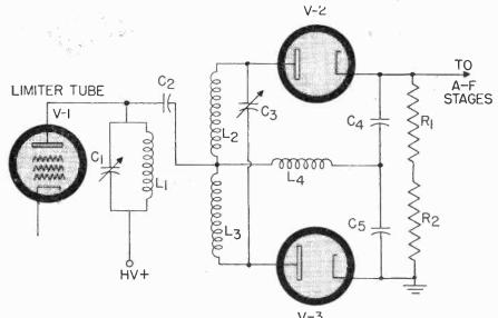
Fig. 1 A typical discriminator circuit, Foster-Seeley type.
