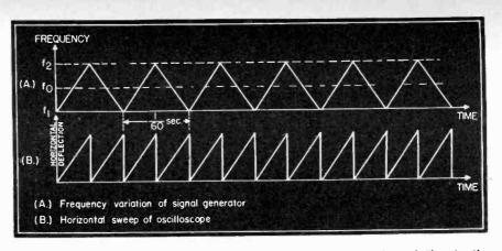
Fig. 7 The frequency variation of the signal generator and its relation to the horizontal sweep of the oscilloscope.
