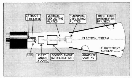
Fig. 3 The upper illustration shows a 3" electrostatically deflected cathode-ray tube of the type commonly found in test oscilloscopes. The lower illustration shows the internal construction of this type of tube.
