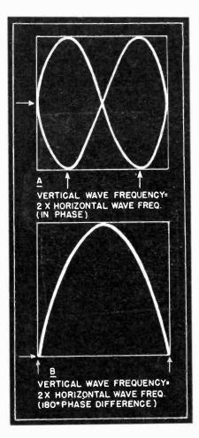
Fig. 7 A shows the pattern obtained when two voltages in phase (one which is twice the frequency of the other) are applied to the vertical and horizontal plates of a cathode-ray tube. B shows the pattern obtained from the same voltages when one is 180° out of phase with the other.
