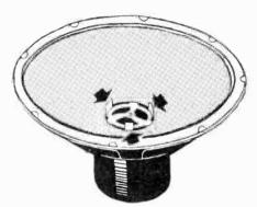
Fig. 1 Placement of shims used when realigning the voice coil of a speaker.
