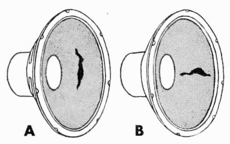
The tear A can be repaired while the one on speaker B cannot.
