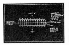
Fig. 4 The electrostatic field set up by the potential applied to the plates changes the direction in which the electron stream is travelling.
