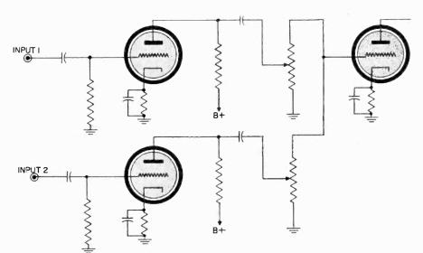
Fig. 12 This circuit is satisfactory for mixing two inputs, although some loss in low frequencies results at low settings of the controls.
