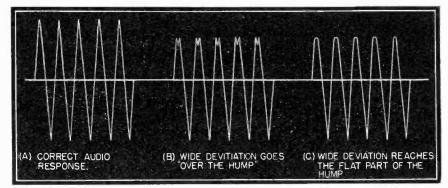
Fig. 3 The effect on the output of a discriminator of a too widely deviated signal.
