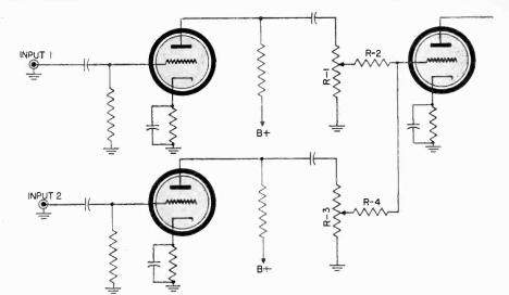
Fig. 11 One method of mixing inputs from two microphones. This method is in common use, and is quite satisfactory.
