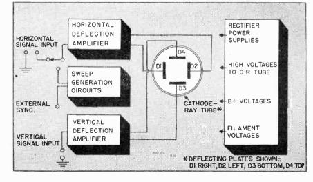
Fig. 1 Block diagram of a cathode-ray oscilloscope.
