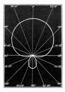
Fig. 4 The Super-Cardioid, resulting from varying sensitivity of one element with respect to the other.
