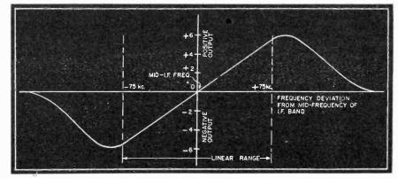
Fig. 2 Output curve of a typical discriminator.
