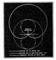
Fig. 3 Addition and subtraction of the sound energy received by the two sections of the uni-directional microphone produce the overall pattern known as a Cardioid.
