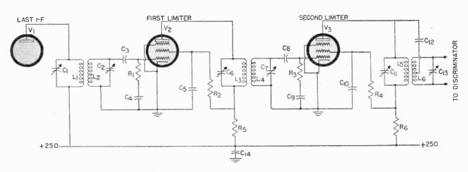
Fig. 6 A two-tube or double limiter circuit.
