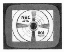
Fig. 8 A test pattern with the horizontal width and vertical height reduced to align the picture parallel to the mask.
