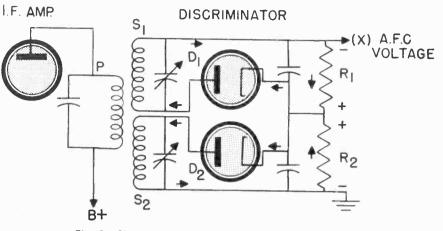
Fig. 3 Simplified diagram of a discriminator circuit.
