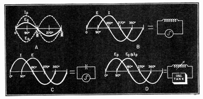
Fig. 2 The voltage and current relationships in an oscillator.
