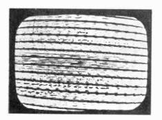
Fig. 17 A test pattern with the horizontal frequency control incorrectly
