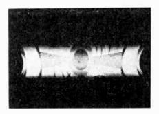
Fig. 9 A test pattern showing the effects of ripple voltage due to a faulty high voltage power supply.
