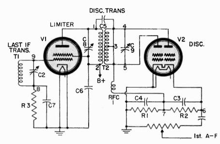
Fig. 4 Partial diagram of a typical limiter and discriminator circuit.
