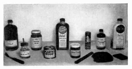
Fig. 1 These are the basic materials needed for cabinet repair work. From left to right they are: Rubbing Oil, Spatula, Alcohol Lamp, Wood Glue, Plastic Wood, Scratch Remover Polish, French Varnish, Stick Shellac, Scratch Stick, Stain, Steel Wool, Sandpaper, Polish, and a Felt Pad.
