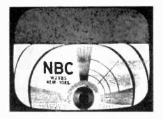
Fig. 14 A test pattern with the vertical centering control incorrectly set.
