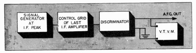
Fig. 6 Connections used for the signal generator and VTVM when adjusting the AFC circuit.
