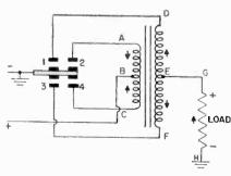
Fig. 9 A circuit diagram for a synchronous type vibrator supply.
