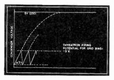
Fig. 6 Graphical illustration of the action which takes place in a thyratron tube.
