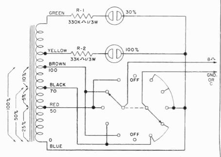
Fig. 3 The circuit used in the output level indicator.
