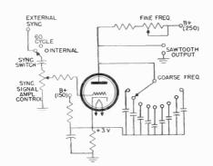
Fig. 4 Thyratron sweep generator circuit as used in the DuMont 208B oscillograph.
