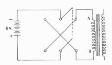
Fig. 3 Switching system used to reverse current flow in a transformer primary.
