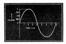
Fig. 1 Voltage units plotted against units of time give a graph as shown above when the voltage is varying in sine wave fashion.
