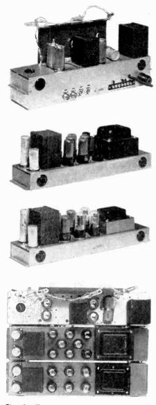
Fig. 1 The three upper units, a fourchannel input unit, a 30-watt amplifier stage, and a 40-watt amplifier stage are plugged together as shown by the photo at the bottom to make a complete 75-watt amplifier.
