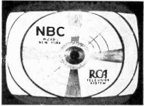
Fig. 11 A test pattern with the vertical height control incorrectly set.
