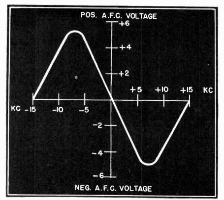
Fig. 4 Typical discriminator output curve.
