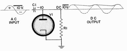
Fig. 2 The AC input is rectified by the diode and fed to the meter circuit.
