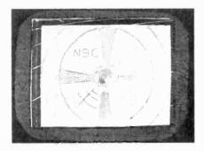
Fig. 21 A test pattern showing the picture size produced by the blanking action.
