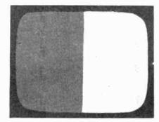
Fig. 19 The pattern produced in the horizontal scanning amplitude test with a 15,750 cps signal on the grid.
