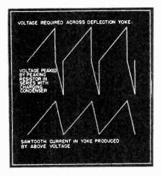
Fig. 15 The voltage and current wave forms required for the magnetic deflection system.
