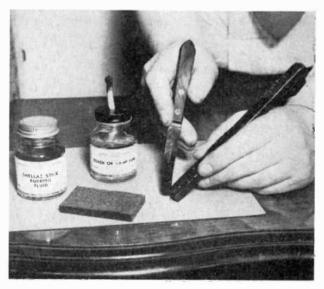
Fig. 4 Melt a portion of the shellac stick onto the hot spatula.
