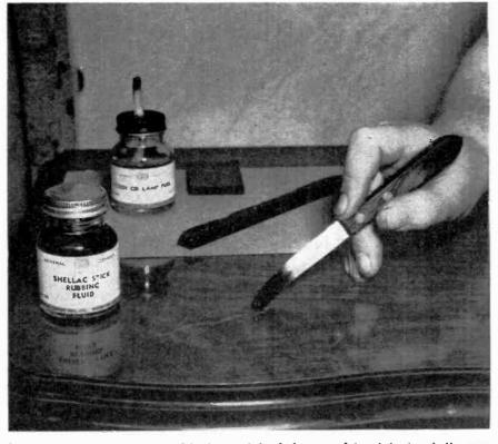
Fig. 5 Fill in the scratch with the spatula, being careful not to touch the surrounding surface.
