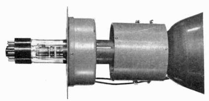
Fig. 5 The arrangement of the focus coil and the deflection yoke on a magnetically focused and deflected tube.
