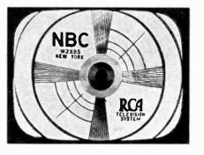
Fig. 1 A normal test pattern.
