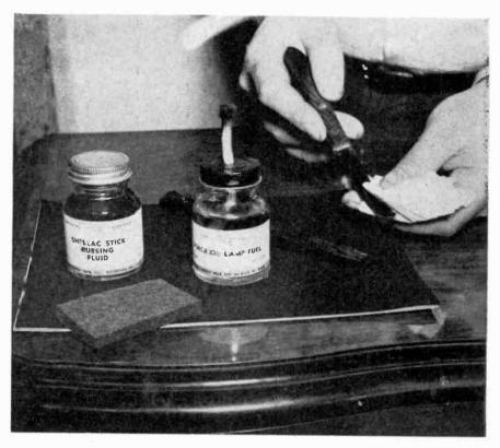
Fig. 3 Wipe the spatula carefully to remove carbon after heating it over the alcohol flames.
