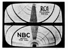
Fig. 12 A test pattern with the vertical synchronization control incorrectly set—the picture moves continually, giving a rolling effect.
