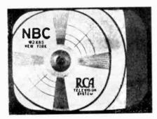
Fig. 23 A test pattern with the horizontal centering control incorrectly set.
