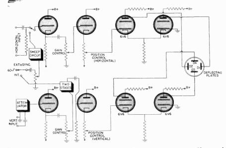
Fig. 7 Simplified schematic diagram of the horizontal and vertical amplifiers used in the DuMont 208B.
