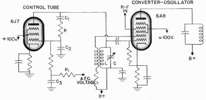
Fig. 5 Simplified diagram of the control tube circuit and the converter-oscillator circuit in a receiver using automatic frequency control.
