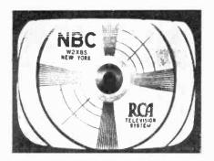
Fig. 16 The fold-over effect caused by improper peaking in the vertical scanning circuit.
