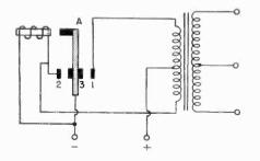
Fig. 6 The primary circuit of a vibrator supply.
