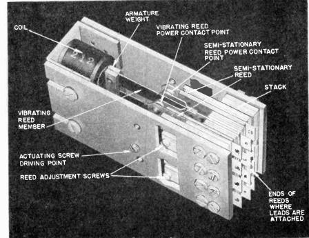
COURTEST OF ELECTRONIC LABORATORIES, INC. Fig. 5 A typical vibrator unit.
