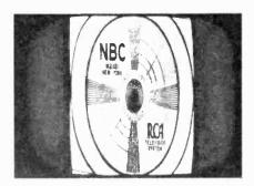
Fig. 20 A test pattern with the horizontal width control incorrectly set.
