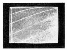
Fig. 6 A correctly oriented scanning raster. Note the angle of the retrace lines.
