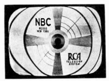
Fig. 25 A test pattern showing nonlinear horizontal deflection.
