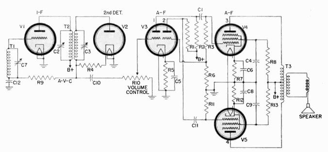
Fig. 3 Partial diagram of a superhet receiver using a phase inverter and push-pull output.
