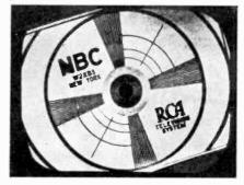
Fig. 7 An incorrectly oriented picture caused by a misaligned deflection yoke or electrostatic tube.
