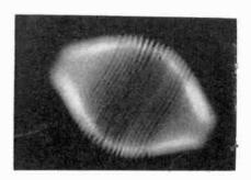
Fig. 6 Vibration caused by the speaker caused the old filament to vibrate like this. It bent in the middle and did not last long.
