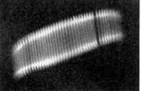
Fig. 8 When the new lamp is subject to vibration, the filament moves back and forth but it does not bend.
