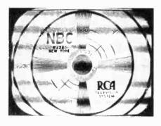
Fig. 3 A test pattern showing sound modulation in the picture caused by improper alignment of the sound traps.
