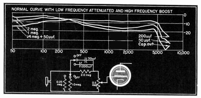
Fig. 7 This circuit permits independent variation of the high and low frequency response. The curve shows the response with various combinations of resistance and capacitance.
