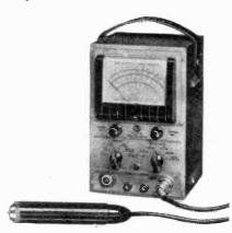
ures voltages up to 1000 volts and resistances of from zero to 1,000 megohms.
