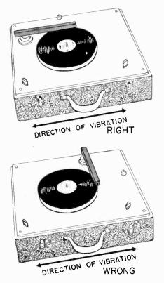
Fig. 4 Method of mounting pickup to minimize the effects of vibration. The pickup arm should be parallel to the direction of vibration.
