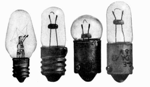
Fig. 1 The four common types of lamp construction. From left to right: The C-7 bulb with miniature screw base; the T-3 bulb with miniature screw base; the G-3 bulb with miniature bayonet base; the T-3 bulb with miniature bayonet base.
