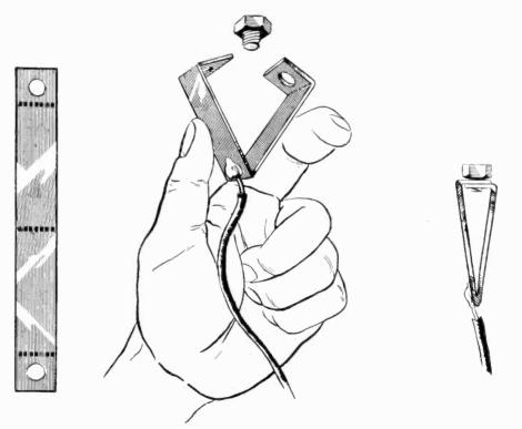
Fig. 3 This clamp is useful when making connections to automobile ammeters. It is made from a small strip of brass.
