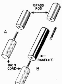
Fig. I. Two types of wand can be made. The one with the bakelite center is more useful.
