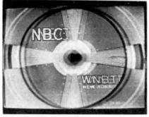
Fig. 17 Ghosts in a picture produced by reflections from structures in the neighborhood of the receiver.
