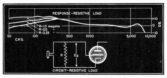
Fig. 5 Method used to connect a crystal pickup to an input stage. The curve above shows the effects upon the response of changes in the value of R. Decreasing the resistance decreases the low frequency response.
