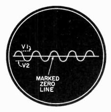
Fig. 5 The DC Voltage is indicated on calibrator voltmeter. The RMS value of the hum is equal to V2 minus VI divided by 2.828.
