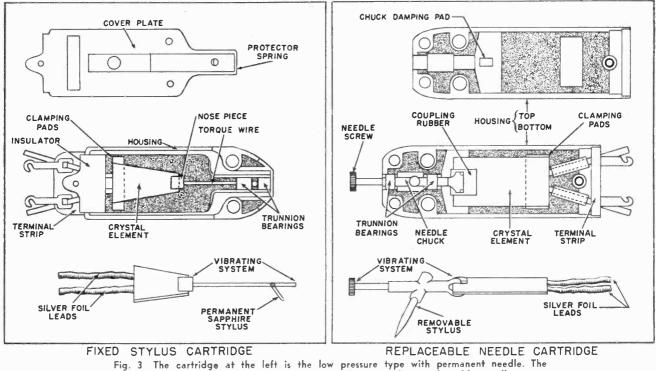
cartridge at the right is the conventional type with a replaceable needle.
