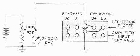
Fig. 1 Connections used when calibrating the oscilloscope. The terminal block shown is that used on the DuMont 208B but the same method can be used with other oscilloscopes.
