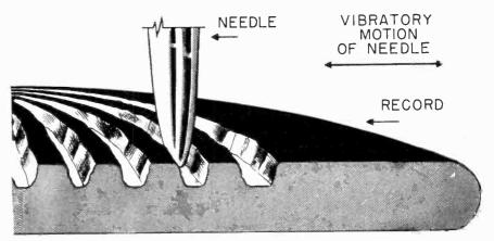
Fig. 2 A greatly enlarged view of a record and needle, showing the needle following the record grooves. The needle is vibrated in proportion to the amplitude of the recorded sound.
