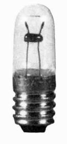
Fig. 7 The new lamp construction which eliminates the effects of vibration. Note the change in the bead position in relation to the filament.
