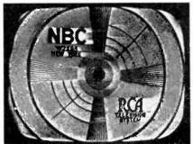
Fig. 10 A test pattern showing loss of low video frequencies due to improper alignment of the video amplifier.
