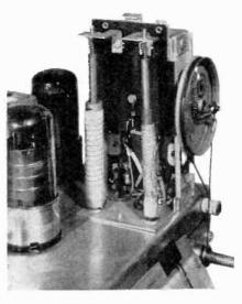
as the Vario-Tuner. The unit is designed to replace the coil and condenser combinations used in conventional broadcast receiver mixer and oscillator stages. It is more efficient, smaller in size, and easier to install than the older gang tuning condenser systems.
