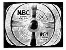
Fig. 11 A test pattern showing loss of high video frequencies due to improper response of the video amplifier.
