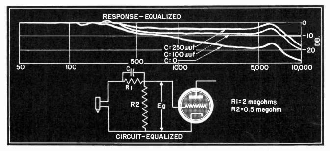
Fig. 6 In this circuit an equalizer has been added. The capacitance C affects the high frequencies while the resistances R-I and R-2 primarily affect the bass response. The curve shows the effect of various values at C.
