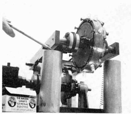
Fig. 9 This gadget is used to check the shock resisting qualities of panel lamps.
