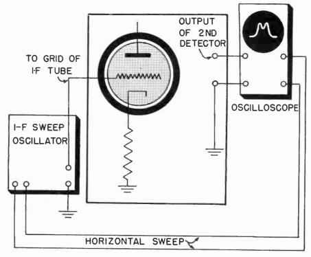
Fig. 12 The connections used when aligning the intermediate amplifiers using the sweep oscillator.
