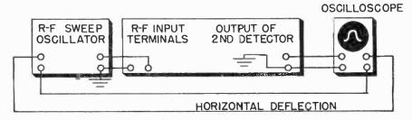
Fig. 15 Connections used when aligning the radio frequency section using a sweep oscillator and oscilloscope.
