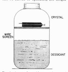
Fig. 8 A crystal cartridge may be stored in this way in humid climates to prolong its life. The desiccator consists of a jar with a piece of ordinary wire screen fitted into it to hold the cartridge above the desiccator liquid. The top should be closed tightly.
