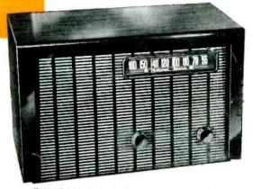
**COMPANION MODEL No. 571.** 5 Tubes. AC-DC. Superbeterodyne Circuit. Built-in Antenna. Automatic Volume Control. 2-Gang Air Condenser Tuning. Illuminated Slide-Rule Dial. Standard American Broadcasts. Walnut Veneer All-Wood Table Cabinet, 13<sup>8</sup>6" x 7%" x 8%".
