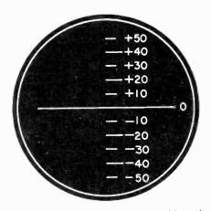
Fig. 2 An Oscilloscope screen calibrated by the method explained in the text. The markings are made with a soft red or blue china marking pencil.
