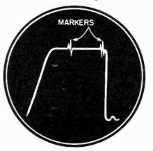
Fig. 13 An intermediate frequency response pattern showing marker pips.
