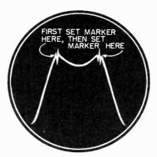
Fig. 7 The oscilloscope pattern obtained when using the sweep generator.
