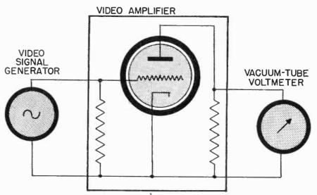
Fig. 5 Method used to measure the video amplifier response with a signal generator
