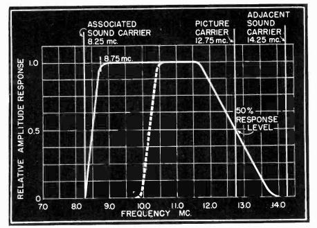
Fig. 2 Ideal picture intermediate frequency response.
