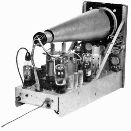
The RCA Model 160 Cathode Ray Oscilloscope. Note the shield covering the Cathode ray tube. The tube with the large cap on top is the high voltage half-wave rectifier.
