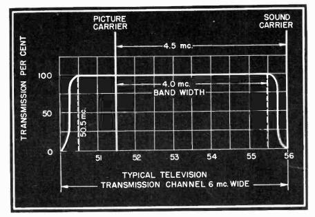
Fig. 4 A typical 6 Mc television channel.
