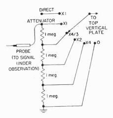
Fig. 3 A simple attenuator used to extend the measuring range of the oscilloscope. The attenuator should be mounted on a small box or chassis.
