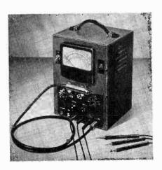
Measurement ranges of the Polymeter include: DC volts, 0-1000, in six ranges; AC volts, 0-300, in five ranges. Current measurements are provided for by seven ranges, and resistance by six ranges up to 1000 megohms.
