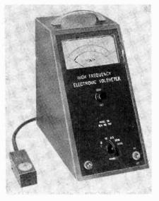
capacity of 5 micro-microfarads or more, the loading and detuning of very high frequency circuits have presented a serious problem, to which Model 32 supplies the
