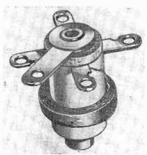
This new adjustable inductance coil can be used for replacement in any radio employing a pentagrid converter and 455/6 kc IF's. A bifiliar winding acts as the grid coupling capacitor when required; and its inductance is adjustable by means of a movable iron core to replace any oscillator coil. It is furnished complete with instructions for use.
