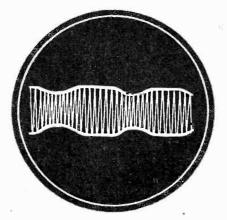
Fig. 9 The pattern obtained with the test setup of Fig. 7 when distortion is present in the receiver.
