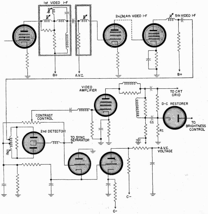
Fig. 2 A simplified schematic diagram of the video channel of a television receiver
