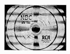
Fig. 8 A test pattern showing the effect caused by sound modulation in the video channel.
