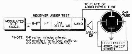
Fig. 1 Method used to check a receiver for overloading. The RF signal generator is set at a point on the broadcast band and its output is modulated by a 400-1000 cycle audio signal.
