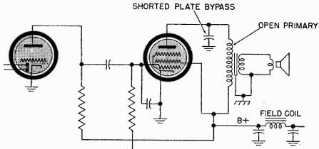
Fig. 2 In a set using a field type speaker, if no stations nor static can be heard but the speaker emits a low hum, the trouble is usually one of those indicated above.
