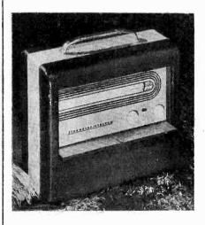
and is housed in a maroon leather-finish fabric case with gray trim. Special features are a tuned radio frequency stage and a built-in low inductance loop. The portable
