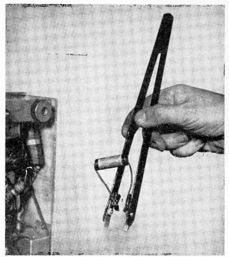
Fig. 3 A handy gadget for use when bridging by-pass condensers to check for opens. Two battery clips are mounted at the ends of the tongs. The battery clips project past the end of the tongs. The proper size condenser is selected and connected to the two clips. A .1 ufd condenser can usually be used to check all the by-passes on a set.
