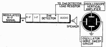
Fig. 5 Method used to check for distortion in the circuits up to and including the second detector.
