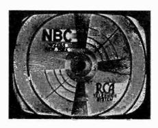
Fig. 7 A test pattern showing the effect of loss of low video frequencies.
