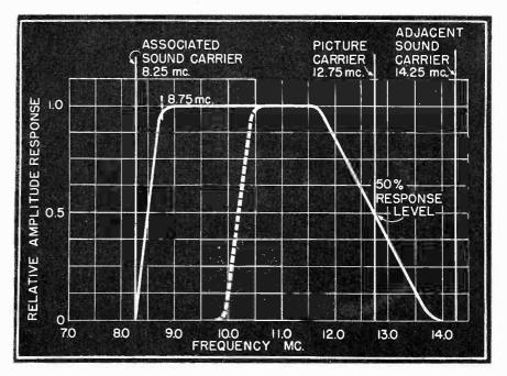
Fig. 3 The ideal picture intermediate frequency amplifier response curve.
