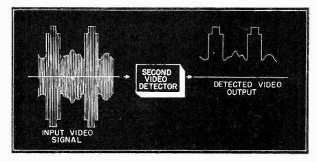
Fig. 4 The input and output signals of the second video detector.
