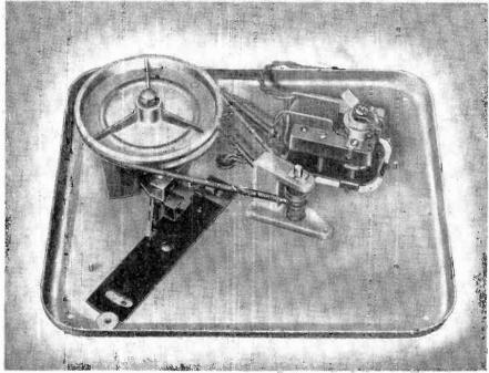
Fig. ? A toggle post drop type record changer. This type of record changer is rapidly gaining in popularity.
