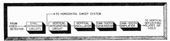
Fig. 1 A block diagram of the vertical sweep system used in a television receiver.
