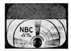
Fig. 12 A test pattern illustrating the effect of an incorrectly set vertical centering control.
