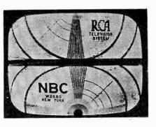
Fig. 9 A test pattern showing the loss of vertical synchronization.
