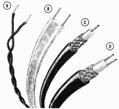
Fig. 1 Four types of transmission line now being used with FM and television antennas: (A) Twisted pair; (B) Two wire parallel conductor; (C) Coaxial cable; (D) Shielded parallel pair.
