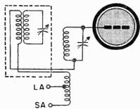
Fig. 5 An absorption type wave trap.
