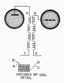
Fig. 3 The construction of an untuned RF coil used in the older receivers.
