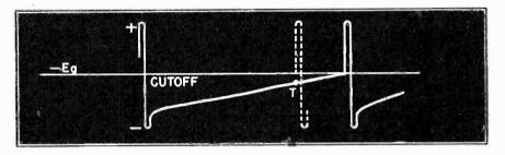
Fig. 7 The waveform of the signal on the grid of the blocking oscillator tube.
