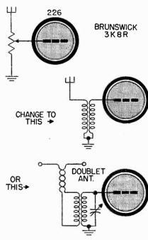
Fig. 2 Either one of the above methods of coupling the antenna is an improvement over the original.
