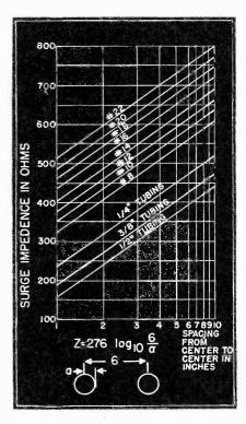
Fig. 4 A chart giving the impedance of two wire parallel transmission line (air dielectric) using various combination of spacing and conductor size.
