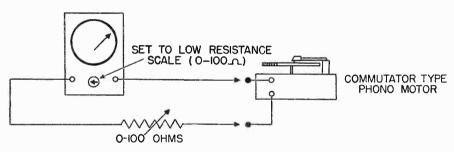
A resistor and ohmmeter connected across the commutator as shown above is used to check brush contact as described in the text.
