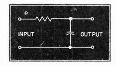
Fig. 5 A resistance capacitance network used to integrate the vertical serrated sync pulse.
