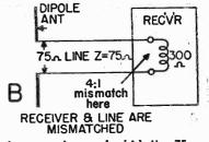
Fig. 6 Correctly and incorrectly matched antenna systems. In (A) the 75-ohm line matches at both the antenna and receiver ends; and, therefore, the match is correct. In (B) the 75-ohm line matches the antenna but does not match the input of the receiver.
