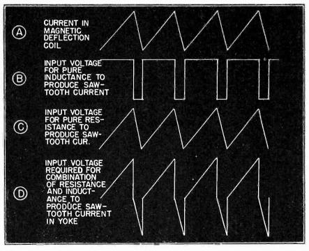
Fig. 8 The waveforms necessary to obtain magnetic deflection: A, the waveform of the current in the magnetic deflection coil; B, the input voltage necessary to produce a saw-tooth current in a pure inductance; C, the input voltage necessary to produce a saw-tooth current in a pure resistance; D, the input voltage required to produce a saw-tooth current in a combination resistance and inductance such as found in the yoke.
