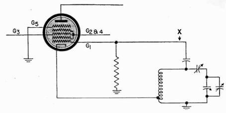
Fig. 7 6SA7 pentagrid converter.
