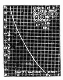
Fig. 9 The length of a quarter wave matching stub for the various FM and television frequencies is shown in the above chart.
