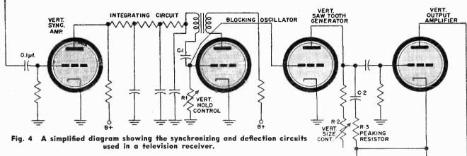
to the clipping action. Usually another stage of sync amplification is used; and sometimes even a second sync separator is introduced that clips noise pulses that might exist on the sync signal. Such a sync separation circuit is used in the RCA TRK 120 and is shown in Fig. 4.
