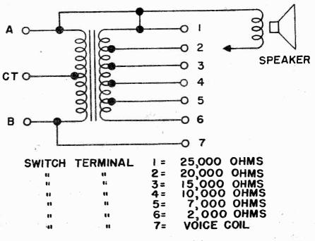
Fig. 5 The circuit diagram of the completed universal speaker.
