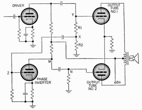
Fig. 2 A phase inverter circuit using two triodes. This circuit is one of the most popular now in use.
