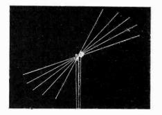
Fig. 10 The Andrew Di-Fan antenna. This antenna covers an extremely wide band of frequencies without serious attenuation.
