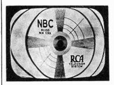
Fig. 9 A test pattern showing horizontal non-linearity.
