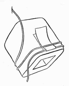
Fig. 2 As shown above, when starting the winding, a piece of paper is used to hold the first turn in place.
