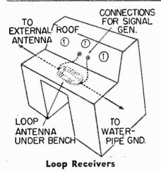
A REPLACEMENT loop antenna fastened underneath the work bench and connected to an outside antenna and ground, as shown in the diagram, will greatly improve the reception of loop receivers standing on the top of the bench. In areas where it is normally necessary to use an outside antenna to secure adequate reception, the auxiliary loop is particularly helpful. The loop is also useful in aligning AC-DC type receivers.
