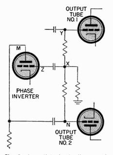
Fig. 3 A partial circuit diagram of the self-balancing type of phase inverter. In this circuit negative feedback is used to balance the signals on the grids of the two tubes used in the phase inverter.
