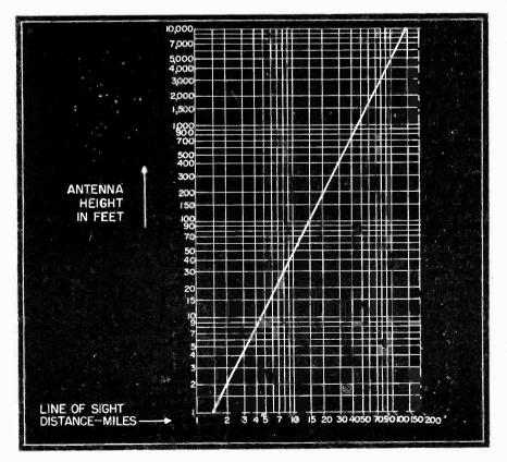
Fig. 9 The above graph shows the relation between antenna height and line of sight transmission distance.
