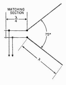
Fig. 12 The rhombic antenna. This antenna gives a low angle of reception and comparatively wide band coverage.
