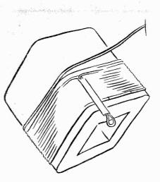
Fig. 3 The taps are made by twisting a pigtail of wire and bringing it to the edge of the winding between layers of insulating paper. The taps may be tagged or identified by their length.
