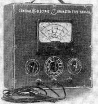
is a 20,000 ohms per volt multi-range instrument. The YMW-1A specifications include resistance with a total coverage of lohm to 20 megohms; voltage, AC and DC, 0-1000 volts; current, 0 to one-half ampere; decibels, minus 4 to plus 62, all designed in convenient ranges.
