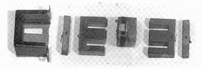
Fig. 1 The completely disassembled transformer ready to rewind.
