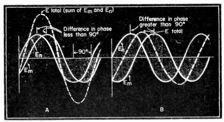
Fig. 5 Graphs of sine waves showing how two AC voltages can produce a sum voltage whose amplitude varies with a change of phase between them.
