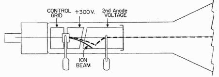
Fig. 2 This diagram shows the operation of the ion trap.
