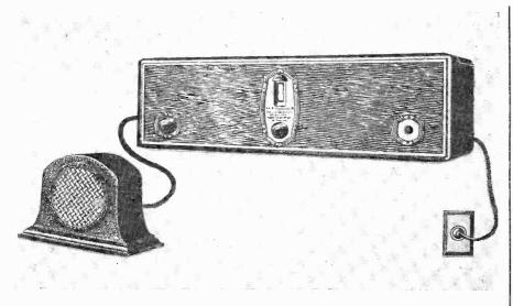
Fig. 8 One of the first "all AC" receivers, the Radiola 18.
