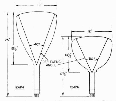
Fig. 8 Showing relative size and shape of old type 12AP4 and new type 12JP4 cathoderay tubes. Though the screen diameters are the same, the new tube is approximately  $7\frac{1}{2}$ " shorter.
