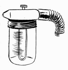
the sprayer head by means of the flexible cable to that point where the dust bag had been attached. The flexible cable is a part normally supplied with the machine and, therefore, does not represent any additional expense. A push-button affair on top of the sprayer head controls the flow of paint.
