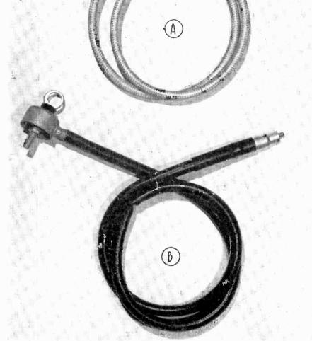
Fig. 1 Two types of antenna lead-in cable for automobile use: A, Polyethylene insulated type; B, older type using paper loom construction and shield can fitting. Choice of lead-in cable can have an important effect on efficiency of the automobile receiver.
