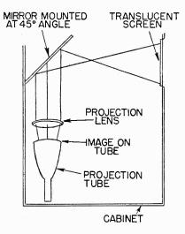
Fig. 10 Projection system using refractive lens.
