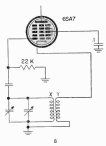
Fig. 4 Similarity between the conventional "tapped coil" (Hartley) oscillator and the type used in the receiver described in the text.
