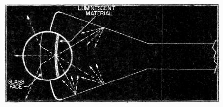
Fig. 3 Conventional cathode-ray tube showing typical distribution of light from a spot.
