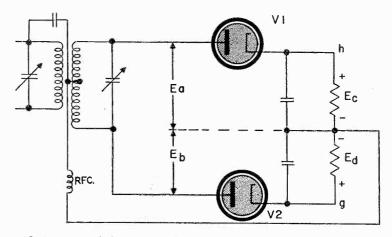
Fig. 6 Basic circuit of the Foster-Seeley discriminator. In practice, point g is usually grounded. Then the audio output appears at point h and AVC or tuning eye voltage can be obtained from the center tap of the resistor.
