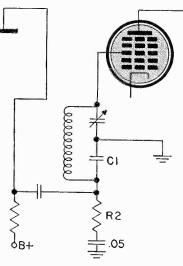
Next we present an analysis of the Buick model 980744-5 which is typical of good quality automobile receivers. It will be noticed in the schematic that all coils used are equipped with adjustable slugs. A ganged permeability (slug) tuner provides the tuning and tracking. Slugs S1, S2 and S3 are mechanically connected in the tuning unit to provide this tracking.
