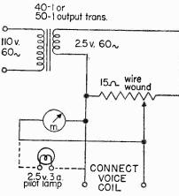
coil of the speaker being tested. Advance the wire wound resistor until the 60 cycle hum is heard in the speaker. This hum should be steady and the bulb should not flicker. Otherwise, an intermittent condition is indicated.
