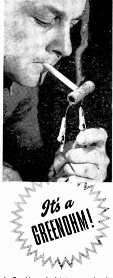
★ Try this overload test on your favorite power resistor. Here's a GREENOHM on 500% overload. It's hot enough to light a cigarette. Yet its special cold-setting inorganic cement coating doesn't soften, bubble or change. When cooled, it doesn't crack, peel, flake. Yes, GREENOHMS can take it. They're tough.
