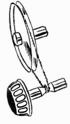
are used, trouble is experienced with the cord slipping off the drive shaft. This trouble can usually be eliminated by filing a slight groove around the shaft. A small rat tail file can be used for this purpose.
