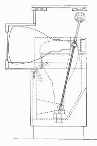
Fig. 6 Lift mechanism for 20" tube.
