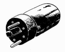
connected to the filament. If we remove a tube with similar filament rating and replace it with the dummy, that circuit has been made dead and we can test accordingly.
