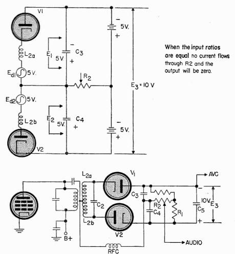
Fig. 8 The ratio discriminator. Below: Schematic diagram, Above: equivalent circuit discussed in the text.
