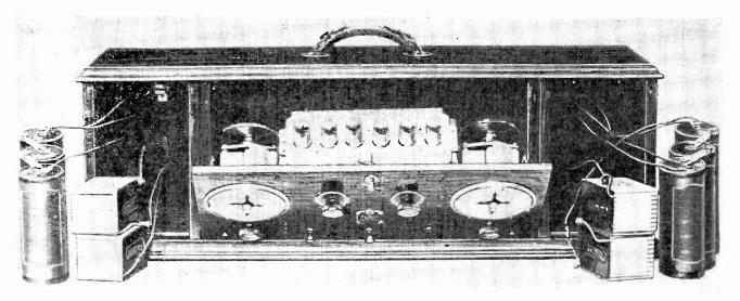
Fig. 6 A definite step forward was marked by the development of this Radiola battery powered superheterodyne.
