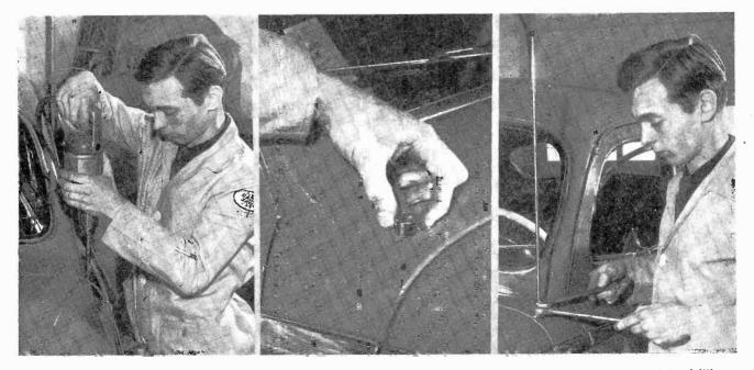
Fig. 4 Steps in making a top cowl antenna installation. Left, hold the drill in vertical position to complete drilling operation; center, using mounting fitting as a template to determine location of mounting hale for a top cowl installation. This gives finished job custom fitted appearance. Right, tightening mast in desired alignment.
