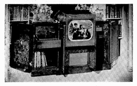
Fig. 7 Television receiver with 20BP4 tube.
