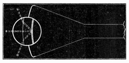
Fig. 4 Cathode-ray tube with aluminum backed screen showing gain of light output.
