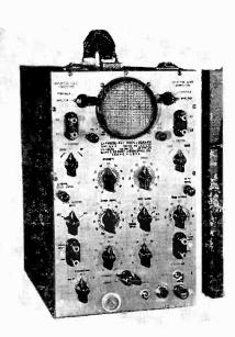
Fig. 7 The DuMont Type 224A cathode-ray oscilloscope.
