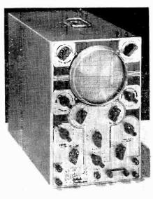
Fig. 8 The Hickok Type 195 cathoderay oscilloscope.
