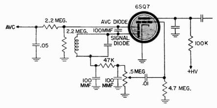
Fig. 1 Typical 2nd detector and resistance coupled audio stage.
