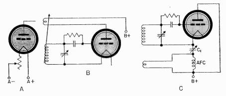
Fig. 1 Earliest methods of control, (A) filament and rheostat, (B) tickler coil variation, (C) capacity feed back control.
