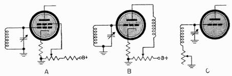
Fig. 4 How volume control is accomplished by variation of the voltage on a tube element.
