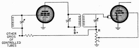
Fig. 5 Modern method of volume control used in superheterodyne receivers.
