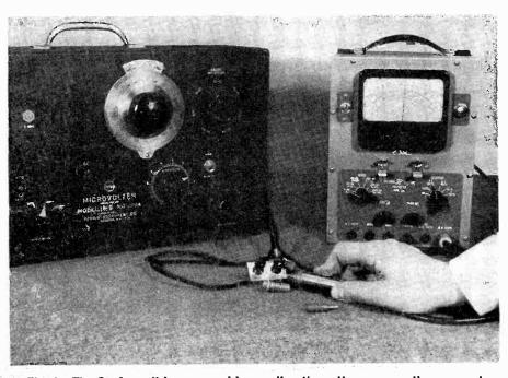
Fig. 8 The Q of a coil is measured by reading the voltage across the resonant circuit. RF energy is provided by a signal generator.
