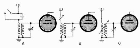
Fig. 2 Early methods used in TRF receivers.
