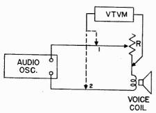
Fig. 2 Diagram showing how a VTVM may be connected to measure voice coil impedance.
