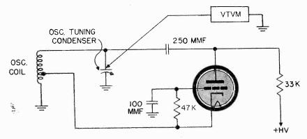
Fig. 6 How to measure the RF output of typical oscillator.
