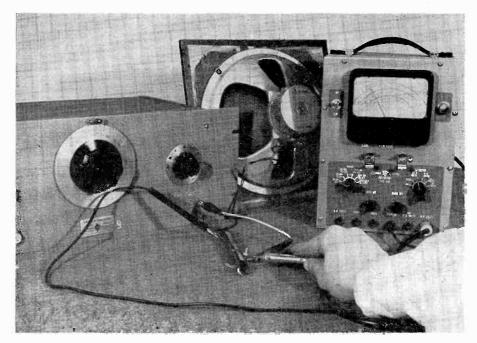
Fig. 3 A typical setup for measuring the impedance of a speaker voice coil.
