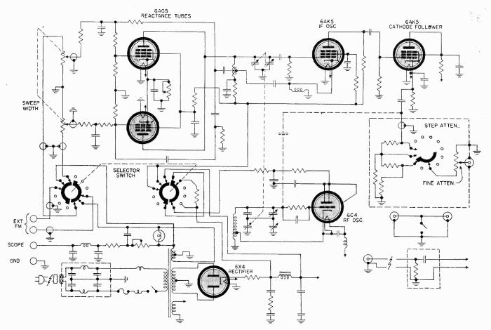
Fig. 2 Complete schematic diagram of the WR53A signal generator.
