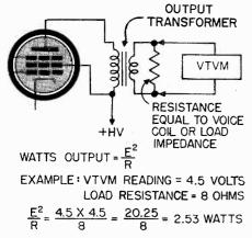
Fig. 4 Diagram showing how to measure audio output power in watts with a YTVM.
