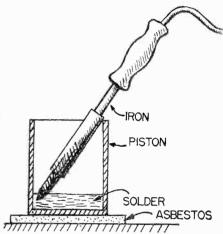
with bar solder. Pistons and irons vary in size so the piston should be chosen to suit the iron. The iron may be left on indefinitely without overheating or becoming "untinned."
