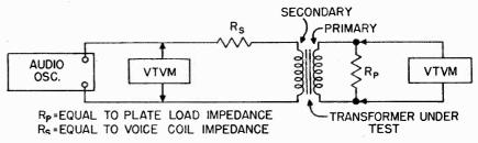
Fig. 5 Measuring the frequency response of an audio transformer.
