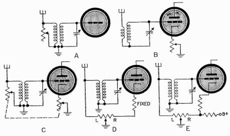
Fig. 3 Antenna shunt and bias method of control.
