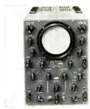
10% from 5 to 200,000 cps. A low voltage version of the instrument is also available as type 250-A. Accelerating potential for the 5CP-A used in this type is 3,000 volts. Detailed information is available from DuMont Labs, Instrument Div., Clifton, N. J.
