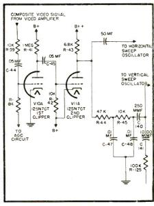
Fig. 3 Some Motorola receivers contain this dual triode which acts as a double clipper
