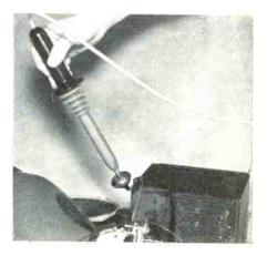
measuring d-c output voltage of pulseoperated and r-f power supplies. For example, if the probe is used with a 100-volt VoltOhmyst meter scale to measure 10,000 volts, the effective resistance of the meter across the voltage source is more than 100,000 ohms per volt deflection. This is especially important where measurement of B plus voltages must be made without loading the circuit. The probes have complete safety features. RCA, Camden, N. J.
