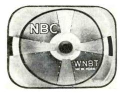
Fig. 4. How non-linear sawtooth affects picture by crowding the lines on one side
