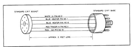
Fig. 1 How the jumper cable is constructed
