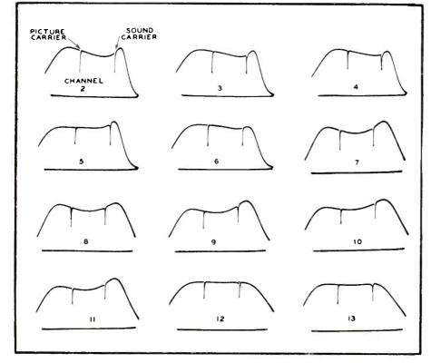
Fig. 3 Typical r-f response curves measured at the oscilloscope terminal.
