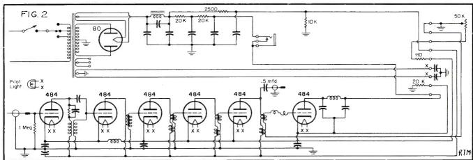
Fig. 1. Circuit diagram of the original Sparton Model 9-30 receiver original tuning section, audio output section, and loudspeaker, and use used by the author for raw material in building his broad-band R.F. of six amplification tubes for R.F. Signal being traced is fed into the Amplifier. Fig. 2. Diagram of circuit as altered. Note absence of grid of the first 484 through input probe.
