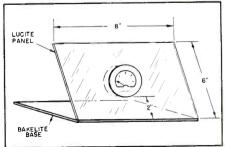
Fig. 2 Mounting ma d-c meter
