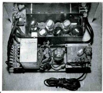
A top view of the unit. Note the .5 mfd., oil-filled condenser mounted inside the case near the filter condenser bank. The co-ax leads going from the panel outlets to the amplifier can be seen. The amplifier cover has been removed.
