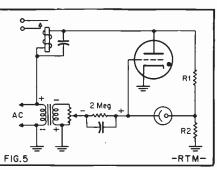
AC operated circuit with voltage divider supplying anode voltages for phototube.
