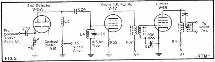
Sound trap take-off circuit in the Emerson Model 609 intercarrier sound receiver. The video signal is taken from the output of  $V_{5a}$  and is coupled to the contrast control,  $R_{10}$ , through the inductance  $L_2$ . The signal reaches the grid of the picture tube through the video amplifiers. A 4.5 Mc beat signal is developed across the trap  $L_1C_{70}$  and fed
