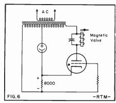
Flame-failure control circuit. Phototube "watches" pilot light of gas or oil burner and closes valve if pilot is extinguished, preventing dangerous accumulation of unignited fuel.
