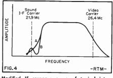
Modified IF response curve of typical intercarrier receiver.
