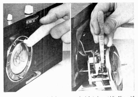
A common clock radic item, a knob that screws onto the shaft, is shown at left. Filing switch contacts with a fingernail file (right) will often cure set difficulties. In removing clock-radio set back (below) watch out that leads to the built-in antenna are replaced in correct order. Best procedure is to make a note of which wire goes to each tie-point.
