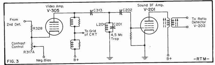
Sound separation circuit in Admiral 20XI receiver. Unlike the circuit shown above, this variation takes the sound signal from the video amplifier rather than from the second detector. A strong 4.5 Mc signal in the trap L<sub>201</sub>C<sub>201</sub> is fed to the sound IF stage V<sub>201</sub>. The trap also prevents any of the 4.5 Mc signal from working into the grid of the
