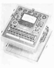
A flexible switching arrangement, a ine voltage control compensating for variations between 105 and 135 volts, and a check for shorts and leakages are provided, the report said.
