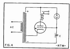
Basic AC operated photoelectric circuit. Capacitor, C, prevents relay chattering when polarity is reversed.
