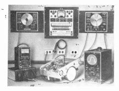
panels, with portable VTVM and fiveinch oscilloscope, as well as a high voltage probe.
