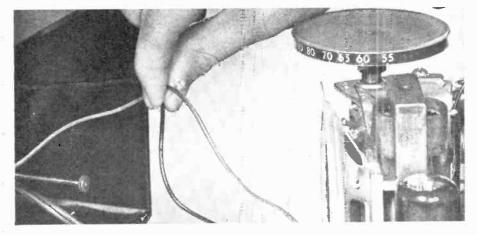
In many cases, difficulty in the clock-radio's cam switching device can be detected by shorting the leads from the switch. In G-E Model 60 pictured, clock housing is removed from the rear, while clock mechanism comes out from the front of the set. Individual replacement parts for clock motor are available.
