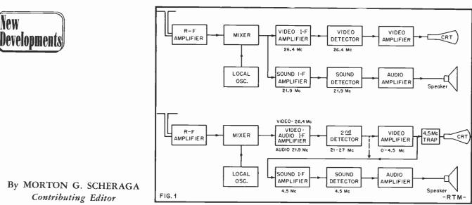
Block diagrams comparing stage relationships of conventional TV receivers and intercarrier sound receivers.
