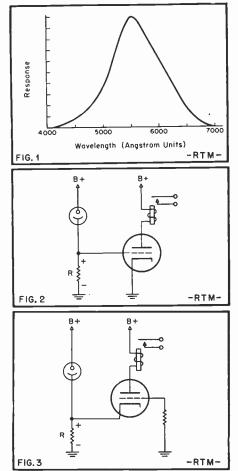
Spectral sensitivity curve (Fig. 1) of a typical phototube. Basic operating circuits of photoelectric control devices, for closing relay when light is turned on and when light is cut off are shown in Figs. 2 and 3.
