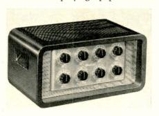
Output of the preamp, measured at 100, 400, and 5000 cycles, is 300 mw, two percent at 600 ohms. Microphone gain is 109 Db on high impedance and 96 Db on low. Phonograph channel gain is 73 Db at 0.5 megohm. Output impedance is 150 or 600 ohms. Hum level is 47 DB below rated output on microphone, 60 Db below rated output on phono. Frequency response is plus or minus one Db, 40 to 20,000 cps.
