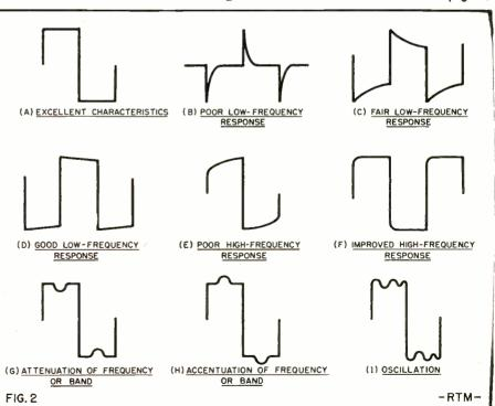
Sample oscilloscope traces resulting from various defects in a piece of audio equipment or a single component, shown with the undistorted wave passed by a first-rate amplifier.
