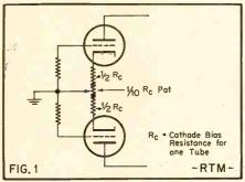
Balancing cathode resistances in a push-pull output stage to equalize the sections.
