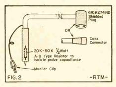
Hum-reducing leads for oscilloscope probes.
