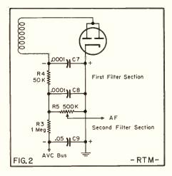
Two-section AVC filter, designed to prevent feedback of audio signal with control voltage.
