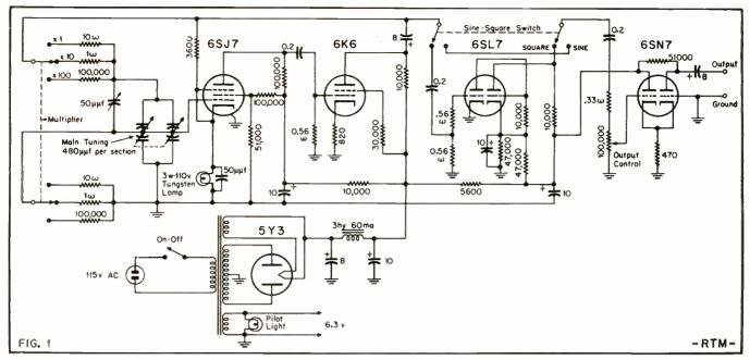
Schematic circuit diagram of the audio generator. For sine waves, the sine-square switch shown simply cuts out the 6SL7 squaring tube.
