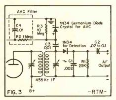
increase when a strong signal generates a high negative voltage, and the amount of bias on this control grid will decrease when a weak signal generates a low negative voltage.
