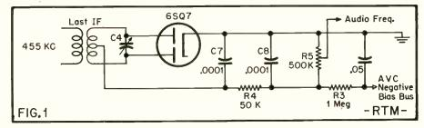
Note similarity of this AVC circuit to that of a full-wave rectifier.
