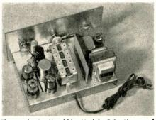
The author's Heathkit Model G<sup>2</sup> Sine and Square Wave Generator, out of its cabinet.
