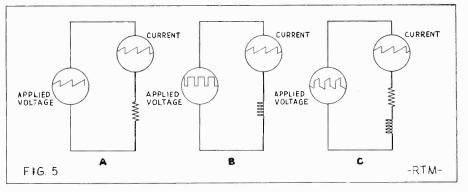
Relationship of voltage and current waveforms when voltage is seen across pure resistance, pure inductance, and a combination of the two, respectively. A applies to electrostatic deflection circuits, and C applies to electro-magnetic circuits.
