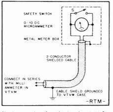
Circuit connections for adapting the VTVM for millivolt measurements. When warmed up, the DC microammeter used by the author drifted from colibration less than 1/50 of the full scale.
