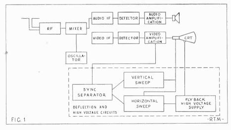
Block diagram of a typical TV receiver employing flyback for the second anode voltage. In this set, brightness of the picture depends on proper operation of the horizontal sweep circuit.
