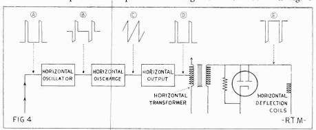
Test points and waveforms in signal tracing of horizontal circuit. Waves shown are "ideal," and may correspond only approximately to those found in actual practice. Settings on the scope are the same as for test of vertical circuit, except for sweep frequency adjustmnt.
