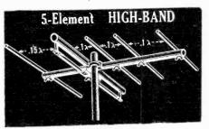
made with one-inch O.D. crossarms, and one-inch and 3/8-inch O.D. elements.
