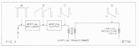
Test points and the proper waveforms to be found in the vertical deflection circuit.
