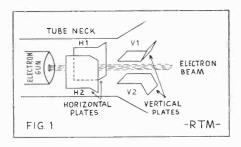
Deflection-plate arrangement in a typical electrostatic-deflection CR tube.
