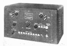
and 60 Mc, with fine tuning control to center the 'scope pattern. The wide band sweep width is 20 Mc, while the narrow band width is 3 Mc.
