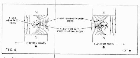
Lines of force created by passing a current through the deflection yoke of a magnetically-deflected picture tube. The action occurs in the horizontal pair of coils and the vertical pair simultaneously, to cause complete scanning of the raster.
