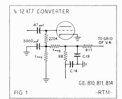
Circuit change in the front end of a typical receiver design, to eliminate 60 cycle buzz (see text).
