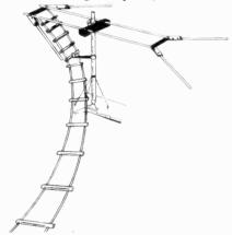
twin leadin. Released figures show 0.5 Db loss per 100 feet at 200 Mc, making possible longer line installations in remote and fringe areas.
