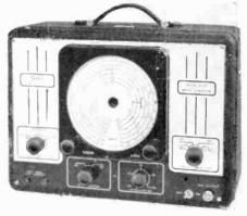
40 Mc, and two harmonic ranges directly calibrated 36 Mc to 120 Mc, are included in the instrument. The range selector is a five-position follow-up coil switch with complete shielding. An RF selector provides high and low RF output, and an output attenuator provides fine control of RF output and a co-axial output cable connector.
