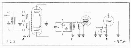
Television input circuits. At A, a balanced 300-ohm input is shown, with a center-tapped choke.
