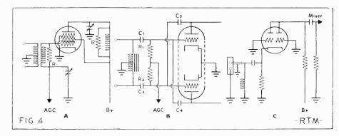
RF amplifier circuits commonly used in television tuners. Respectively, A, B and C are the conventional grid input circuit; the amplifier used in the RCA 630TS circuits; and the grounded-grid circuit. Grid acts as shield between input and output in circuit C.
