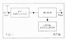
Block diagram of a typical TV tuner.
