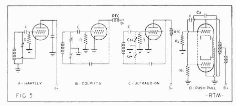
Representative circuit arrangements used for the local oscillators of television receivers. Note similarities of first three circuits. Most commonly used is the ultraudion shown at C.
