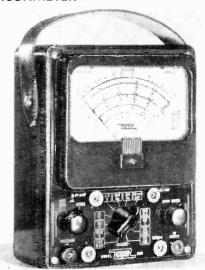
The new 20,000 ohms-per-volt Multimeter. Model 555, just released by the Electronic Instrument Co., Inc., 276 Newport Street, Brooklyn 12, N. Y., incorporates 31 different ranges.
