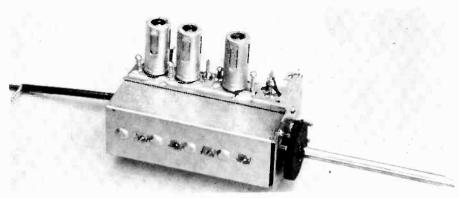
The "Teletuner," a complete front end built by Mallory around its four-gang "Inductuner" (see cut at bottom of page).
