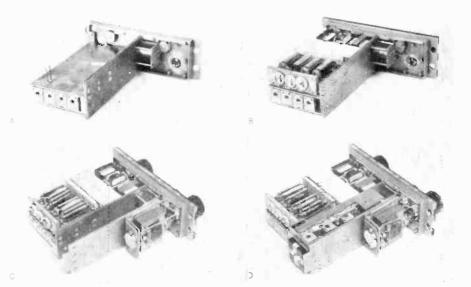
Subassemblies used in the new receiver. A shows tuning assembly and RF inductors in place. At B, RF amplifier and power-filter assemblies have been added. At C, output transformer, patentiometer, and other hardware are in place. At D, IF amplifier, input-output connector are installed and the set is ready to be sealed in its case. Audio output tube assembly is plugged on the outside of case for easy replacement.
