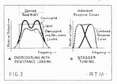
Methods of broadening the response curve of a TV stage.
