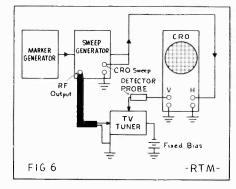
Connections between oscilloscope, sweep, and marker generators for alignment of TV front end.
