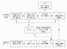
Block diagram of the subminiature set. Conventional superhet circuit is used.
