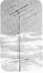
Double Stacked JC Array with full-wave spacing. Provides highest possible gain in low noise areas.
