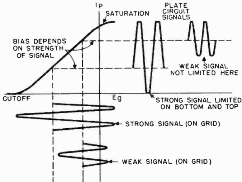
Figure 166. Operation of limiter circuit.
