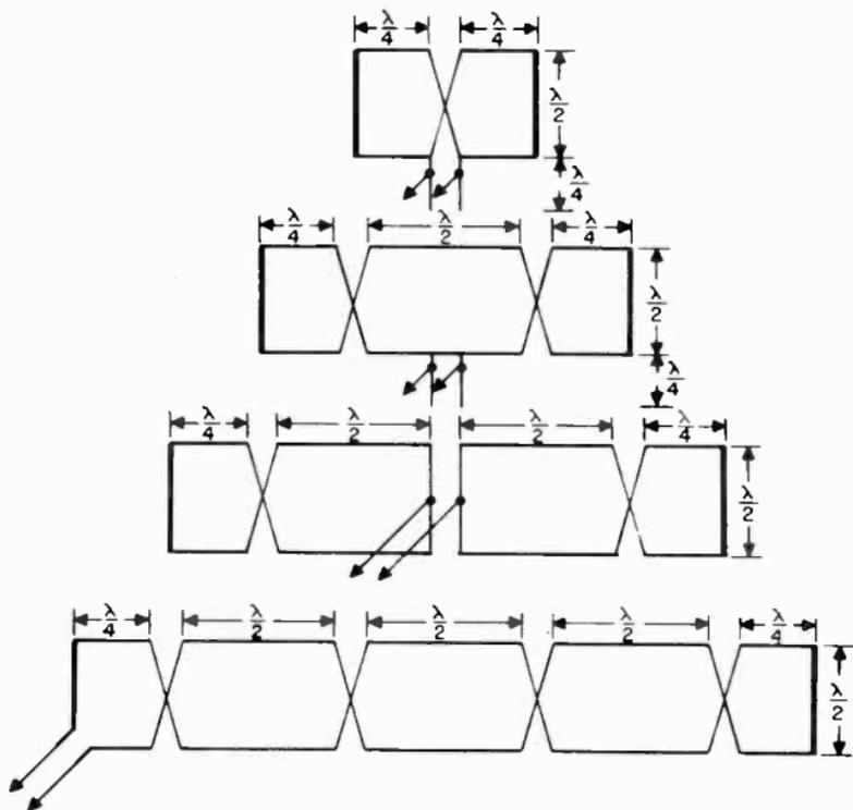
Figure 67. Four types of horizontal sterba arrays.
