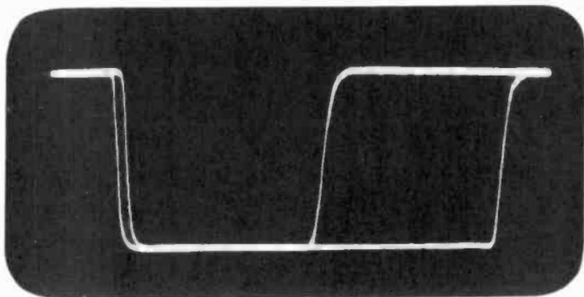
Figure 125. Superimposed horizontal sync pulse and equalizing pulse used to check interlace.
