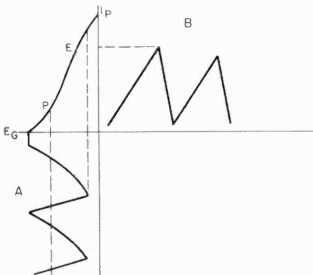
Figure 112. Removal of non-linearity from saw-tooth by operating on curved portion of characteristic curve.
