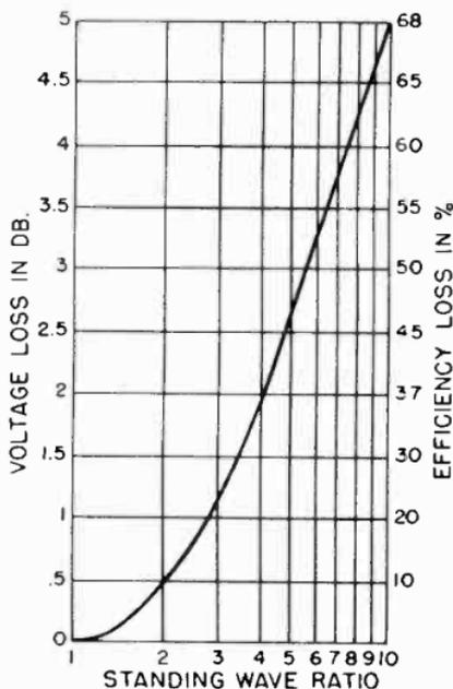
Figure 15. Curve showing the voltage loss in db and the efficiency loss in percent for various standing wave ratios.
