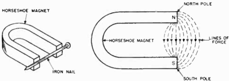
Figure 19. Left, the magnetic field between the poles of the horseshoe magnet pulls the nail to the magnet. Right, the lines of force around a horseshoe magnet.
