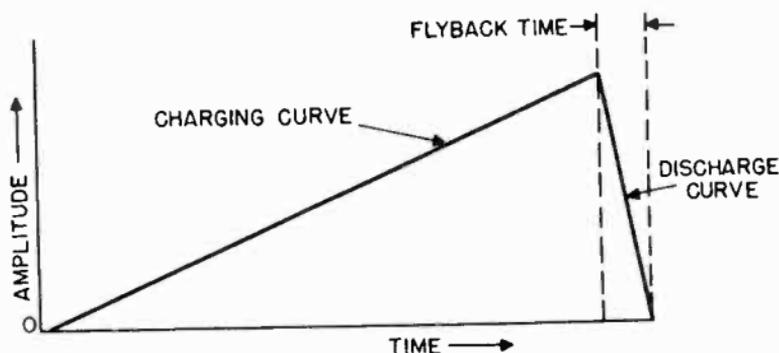
Figure 32. A sawtooth voltage.
