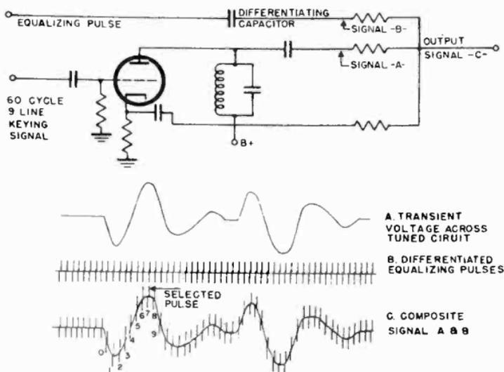
Figure 30. Forming the 60-cycle, three-line keying signal.
