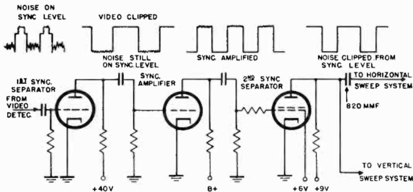
Figure 83. Cascade sync clipper.
