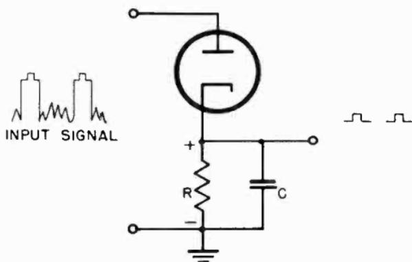
Figure 81. Self-biased diode sync clipper.
