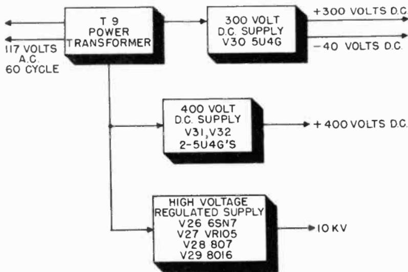
Figure 38. Block diagram of power supply chassis.
