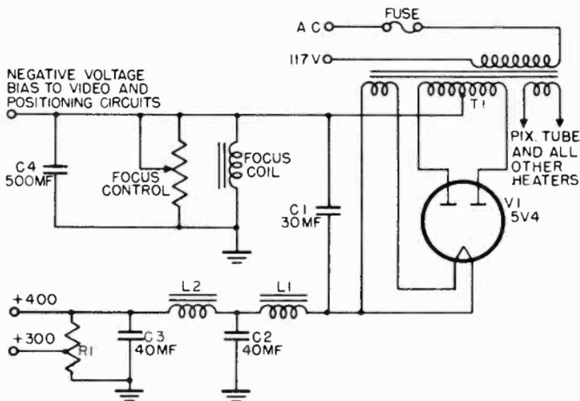
Figure 143. Typical low-voltage power supply.
