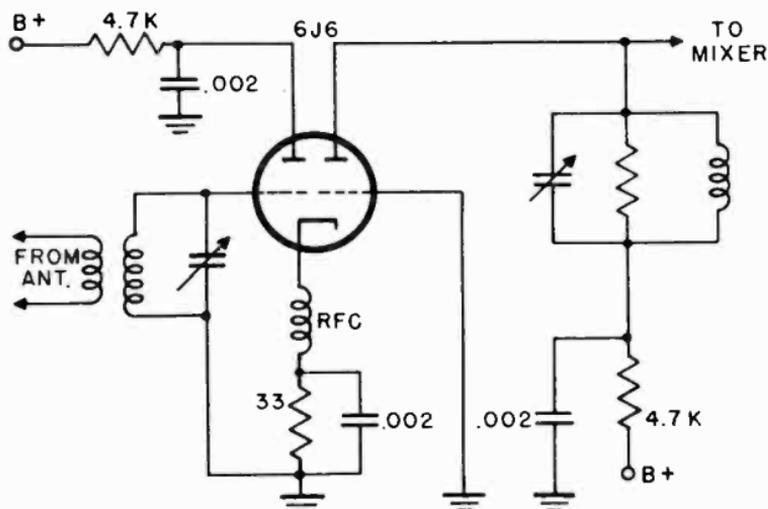
Figure 7. Cathode-coupled r-f amplifier.
