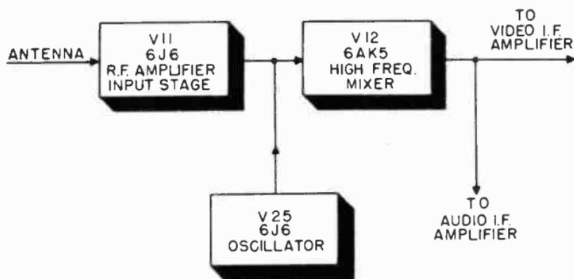
Figure 11. Block diagram of DuMont Inputuner.
