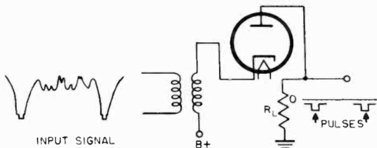
Figure 80. Diode sync clipper.
