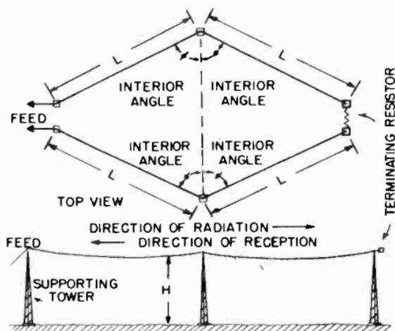
Figure 76. Rhombic antenna.
