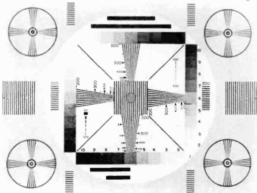
Figure 69. RMA test pattern.
