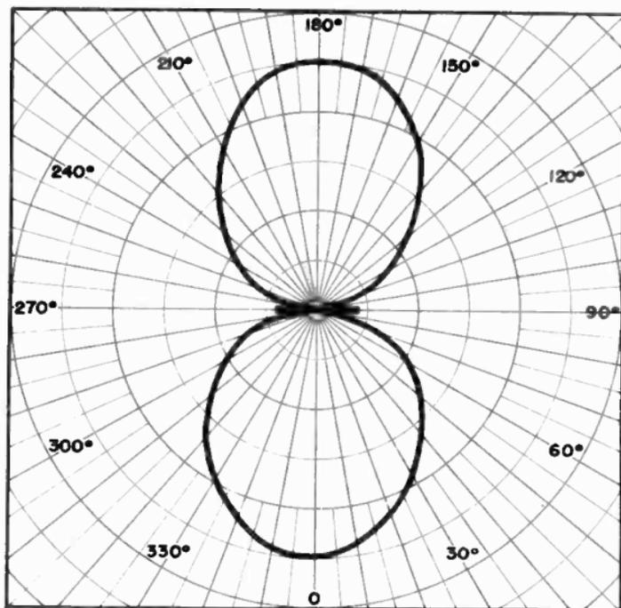
Figure 40. Field pattern of bat-wing antenna at 80 Mc.
