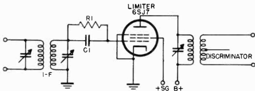
Figure 165. Simplified schematic of limiter circuit.
