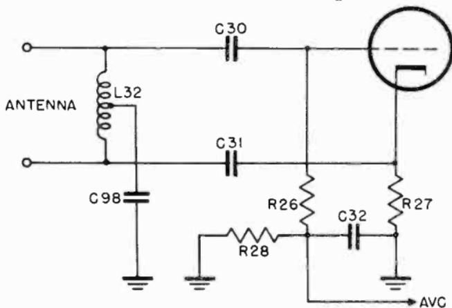
Figure 8. Antenna input circuit.
