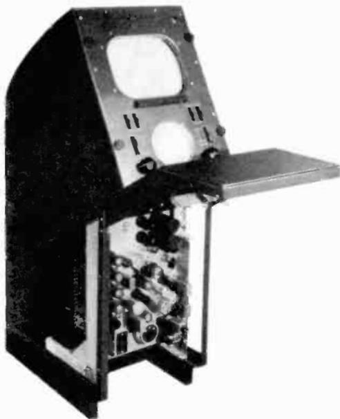
Figure 90. Studio picture monitor. (courtesy RCA)
