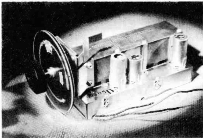
Figure 13. Complete Input tuner assembly for continuous 44-216 Mc coverage, showing manual drive dial. (courtesy DuMont)
