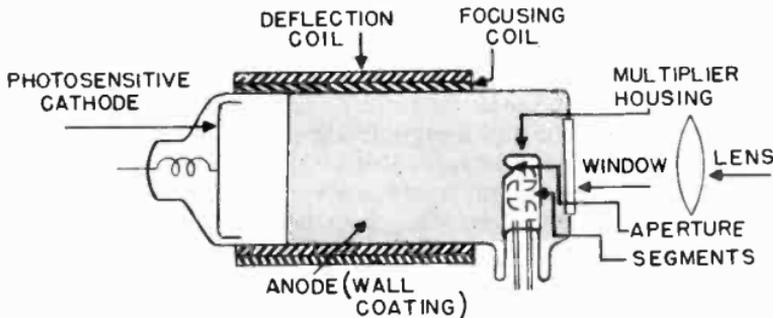
Figure 3. Construction of the image dissector.
