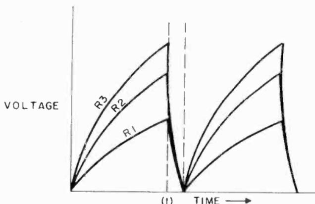
Figure 105. Effect on charging curve of different values of  $R$  in Figure 104.
