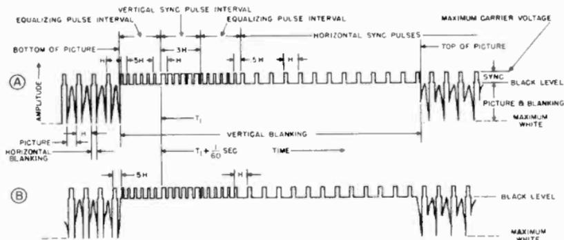
Figure 19. Standard F.C.C. television signal.
