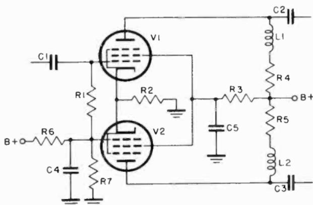
Figure 4. Cathode-coupled output stage.
