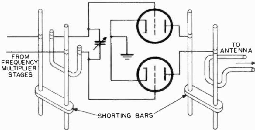
Figure 46. Transmission line tuned push-pull r-f amplifier stage.
