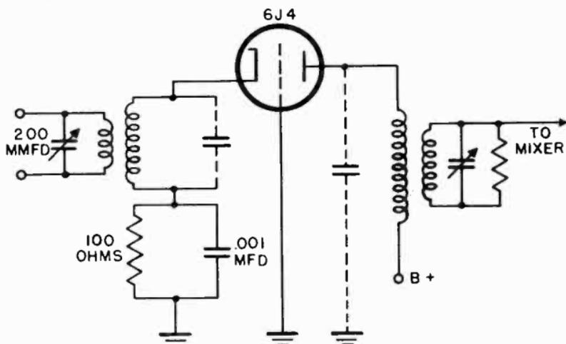
Figure 6. Grounded-grid r-f amplifier.
