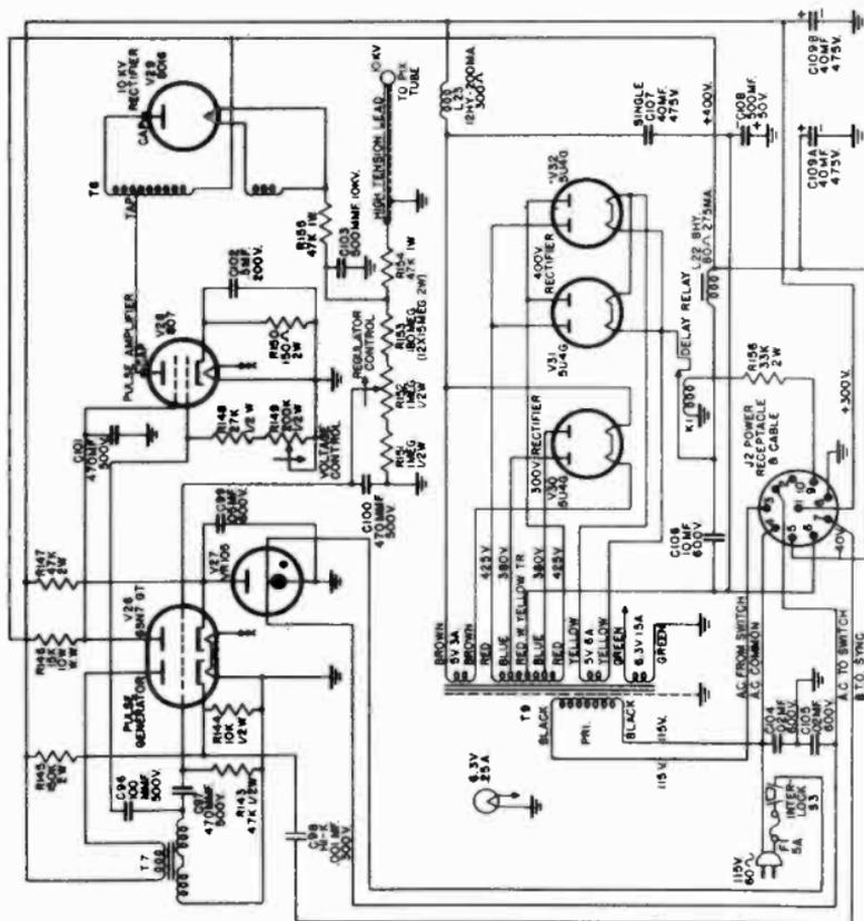
Figure 39. Schematic diagram of low and high voltage power supplies.
