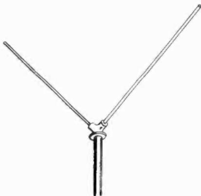
Figure 31. Adjustable V antenna.
