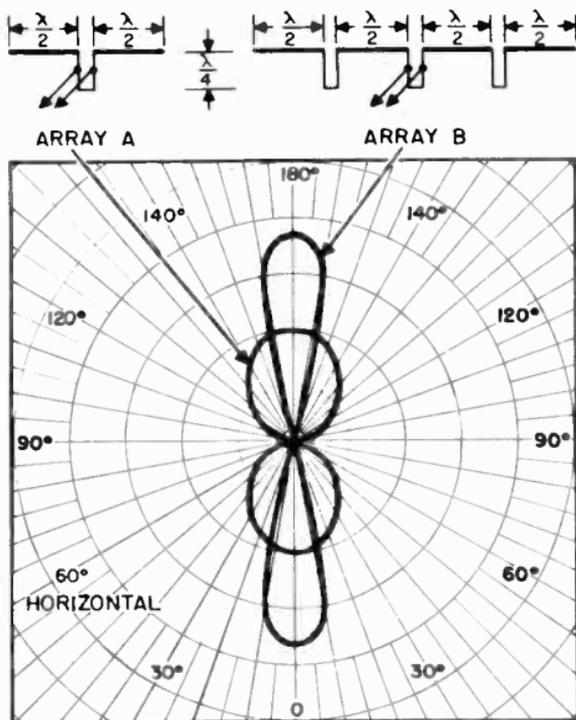
Figure 64. Two types of colinear phased arrays.
