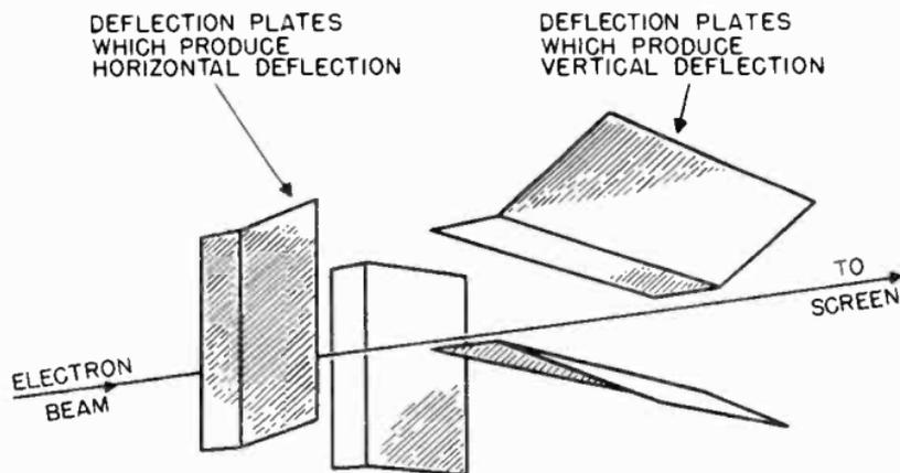
Figure 27. Two pairs of deflection plates mounted at right angles to each other.
