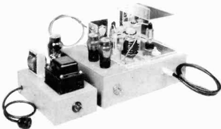
Figure 147. R-F high voltage power supply.
