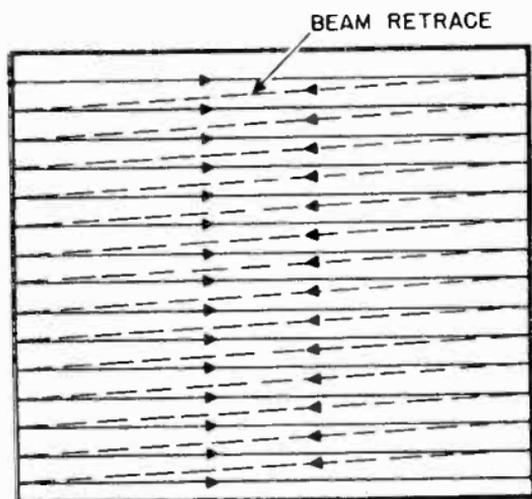
Figure 53A Simple scanning pattern.
