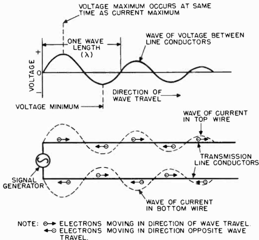
Figure 13. Voltage and current distribution along infinite line.
