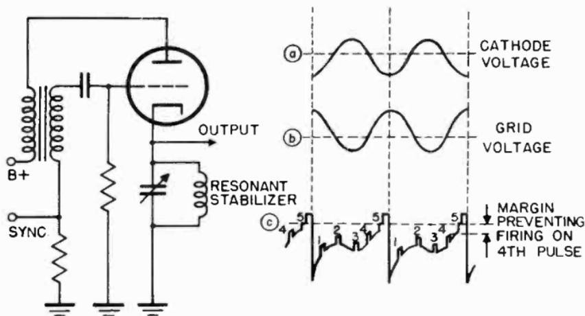
Figure 24. Stabilized blocking oscillator frequency divider.
