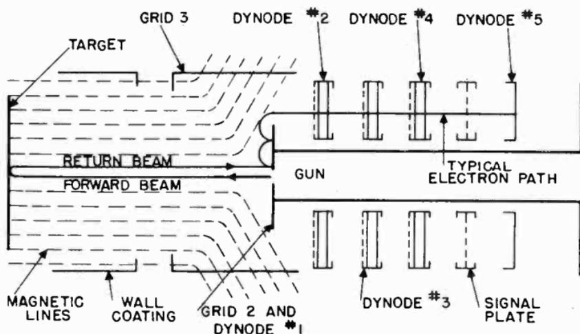
Figure 10. Electron Multiplier Section of the image orthicon.
