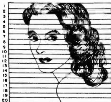
Figure 9. How linear scanning is accomplished.
