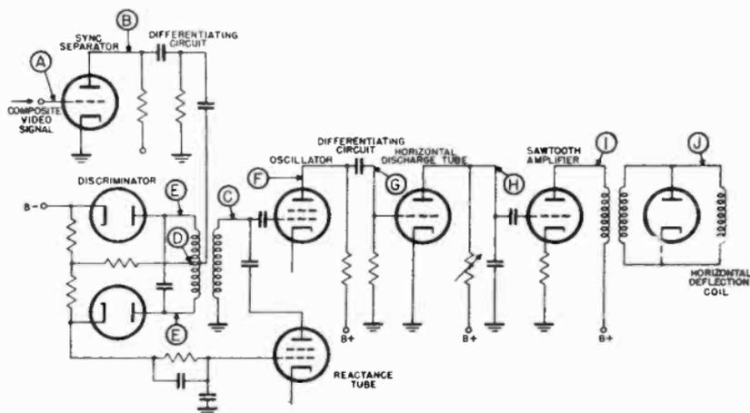
Figure 48. Simplified schematic of horizontal sweep circuit employing fly-wheel synchronization. Waveforms of Figure 47 appear at points indicated.
