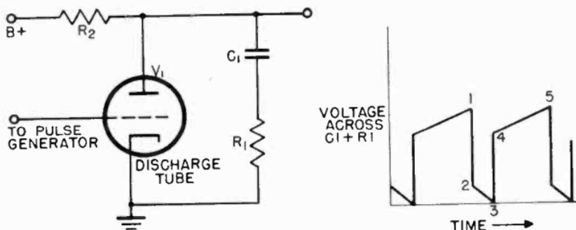
Figure 115. Discharge tube with peaking circuit.
