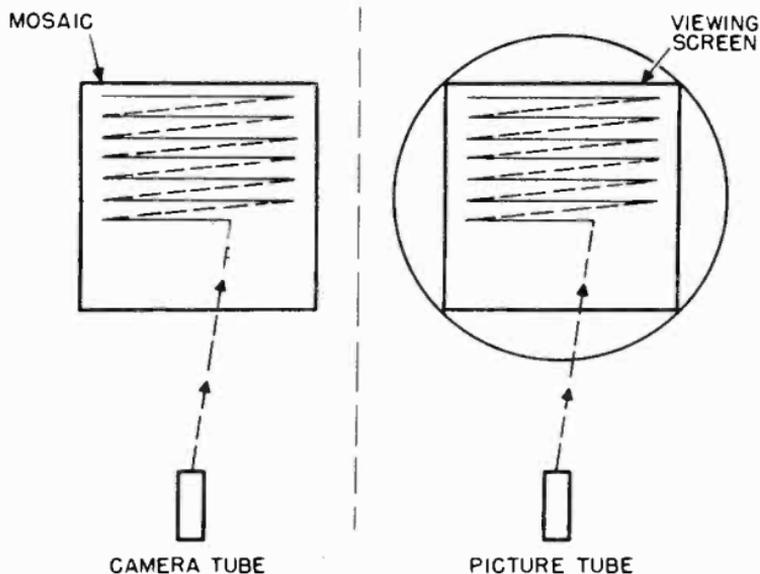
Figure 50. The electron beam scans the mosaic in exact synchronism with the electron beam in the picture tube.
