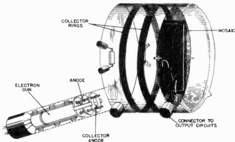
Figure 39. Construction of the Iconoscope.
