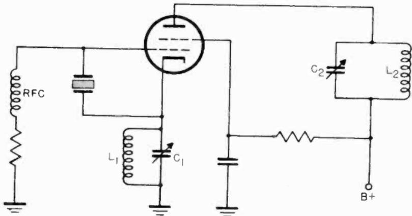
Figure 44. Tri-tet oscillator.
