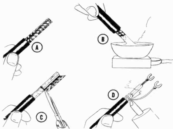
Figure 12. Finishing end of coaxial cable by tinning end of cable and scoring tinned braid. A, cut back rubber insulation. B, dip braid into solder. C, score braid and peel off. D, attach lead and lug to braid.
