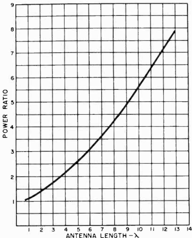
Figure 71. Power gain of long-wire antenna over half-wave antenna.
