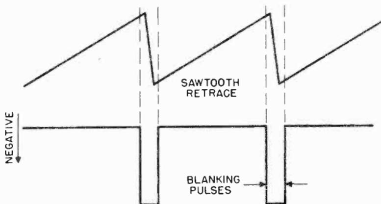
Figure 59. Waveshape and polarity of blanking pulses.
