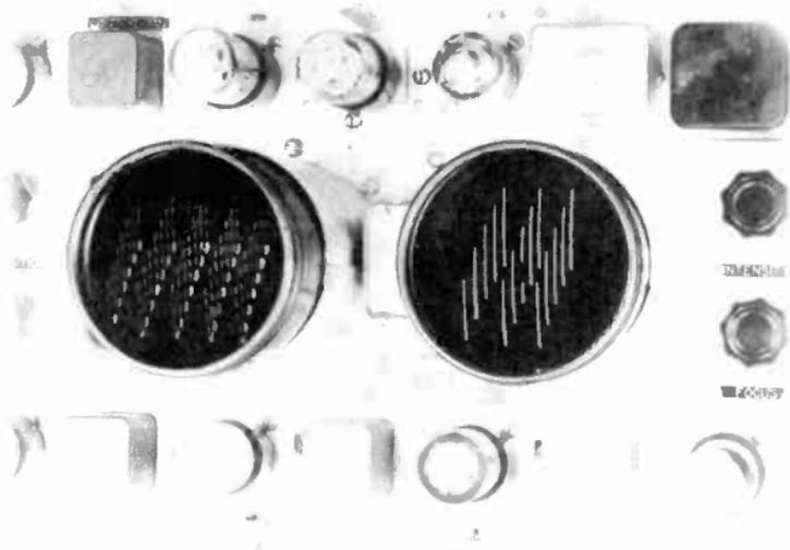
Figure 93. Screens of cathode-ray tube indicators for monitoring synchronizing generator. (courtesy DuMont)
