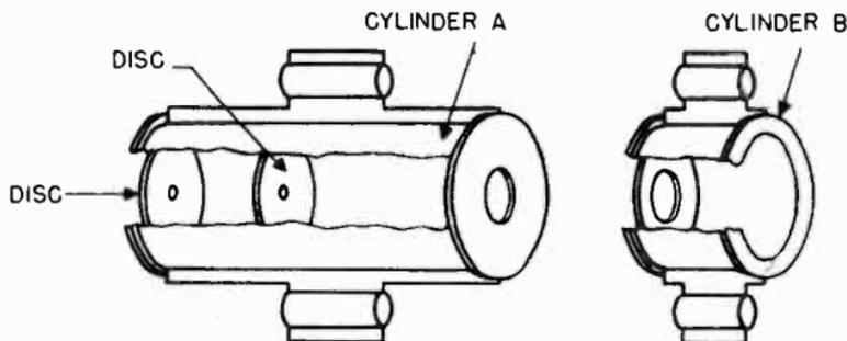
Figure 7. The pre-accelerator electrode assembly.
