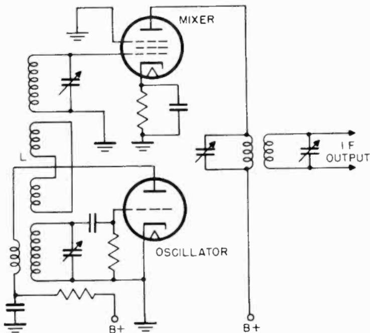
Figure 15. Inductively-coupled mixer-oscillator.
