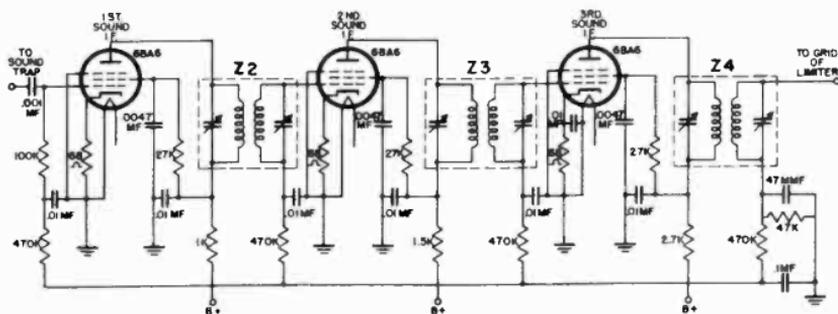
Figure 164. Three-stage sound i-f amplifier.
