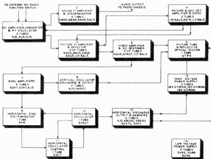
Figure 52. Block diagram of Model 648 PTK.
