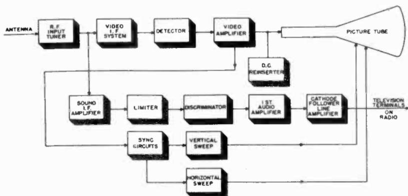
Figure 32. Block diagram of main chassis.
