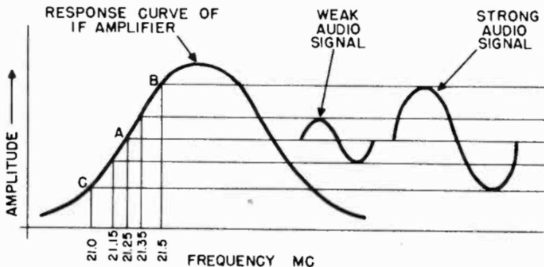
Figure 169. Operation of slope detector.
