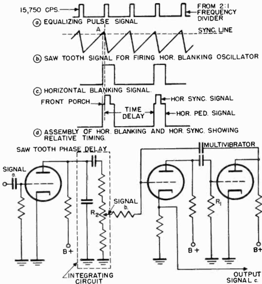
Figure 27. Generation of horizontal blanking pulses.
