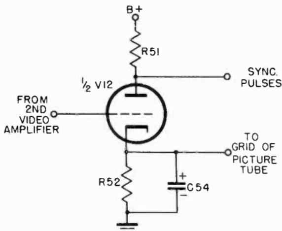
Figure 18. Sync separator and d-c restorer.
