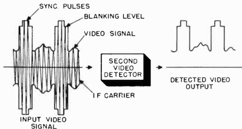
Figure 52. Input and output waveforms of the second detector.
