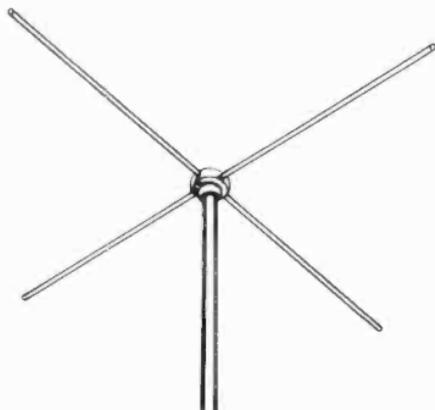
Figure 33. Crossed dipole antenna.
