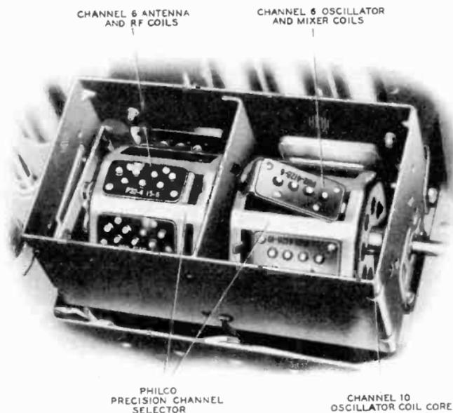
Figure 6. Octagonal turrets used in Philco tuner showing "snap-in" coils. (courtesy Philco)
