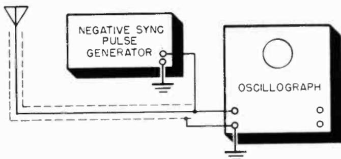
Figure 130. Method used to check antenna impedance match.
