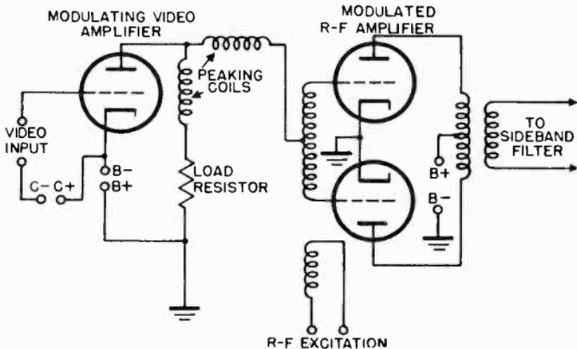
Figure 52. Modulated Class B amplifier.
