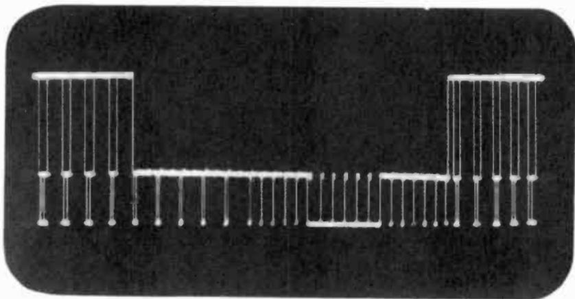
Figure 122. Vertical blanking interval. (courtesy DuMont)
