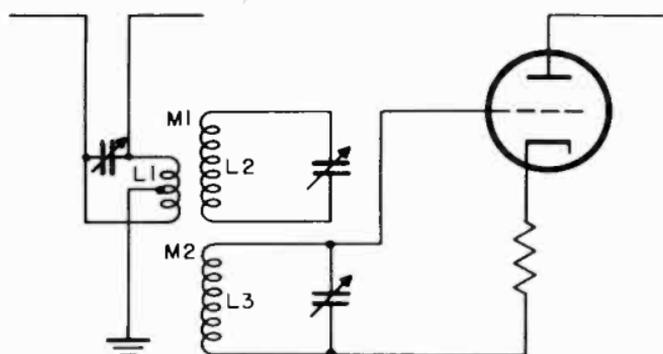
Figure 30. Double tuned antenna coupling circuit with tuned link added.
