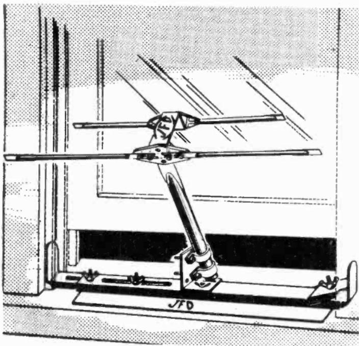
Figure 23. Window sill mounting bracket. (courtesy JFD)
