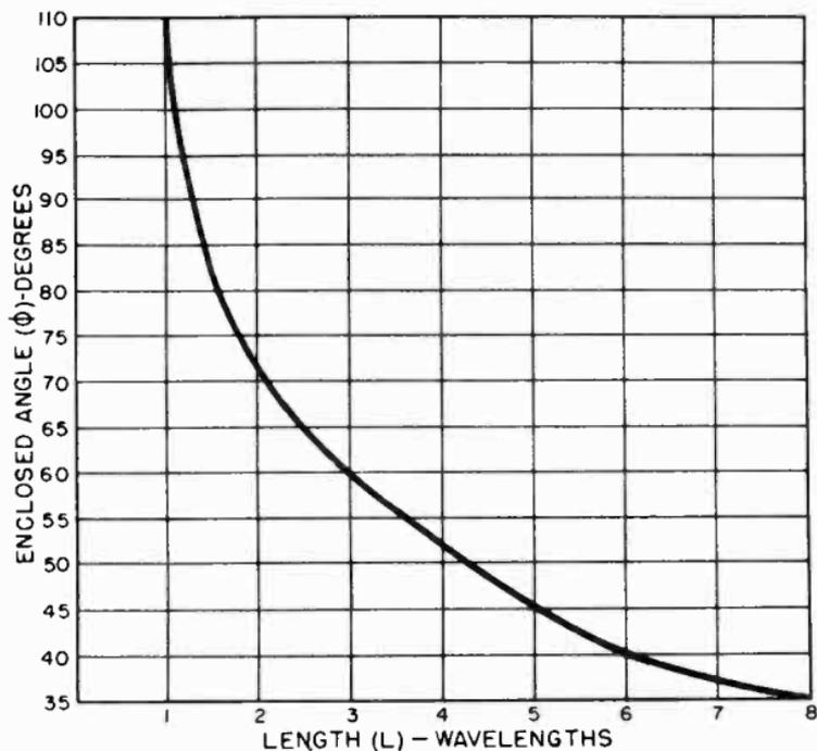
Figure 75. Curve showing change in enclosed angle of V antenna with various frequencies.
