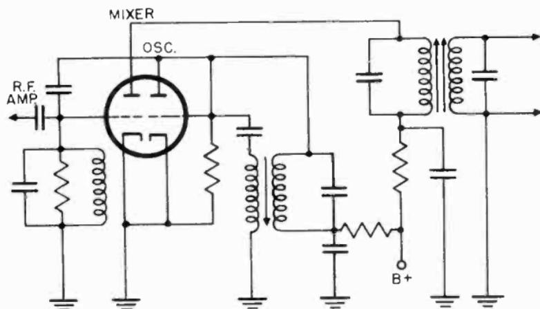
Figure 17. Dual triode mixer-oscillator using grid injection.
