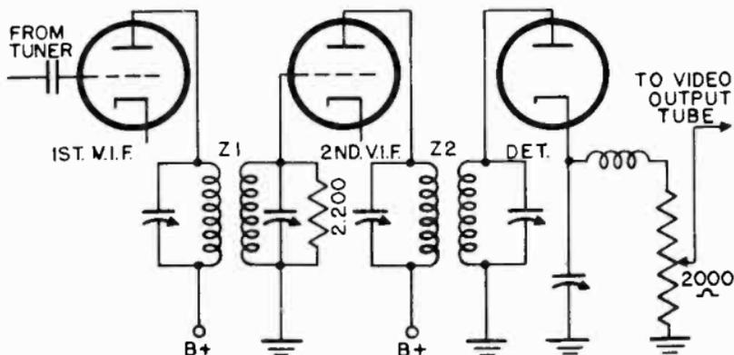
Figure 37. Simplified schematic of broadband overcoupled i-f amplifier.
