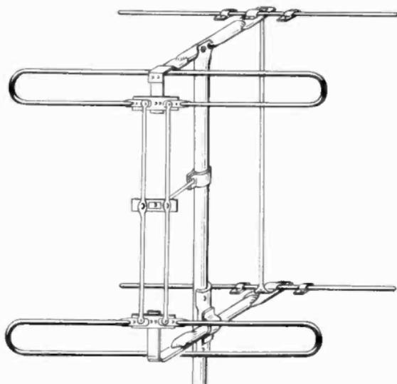
Figure 61. Stacked folded dipoles and reflectors.
