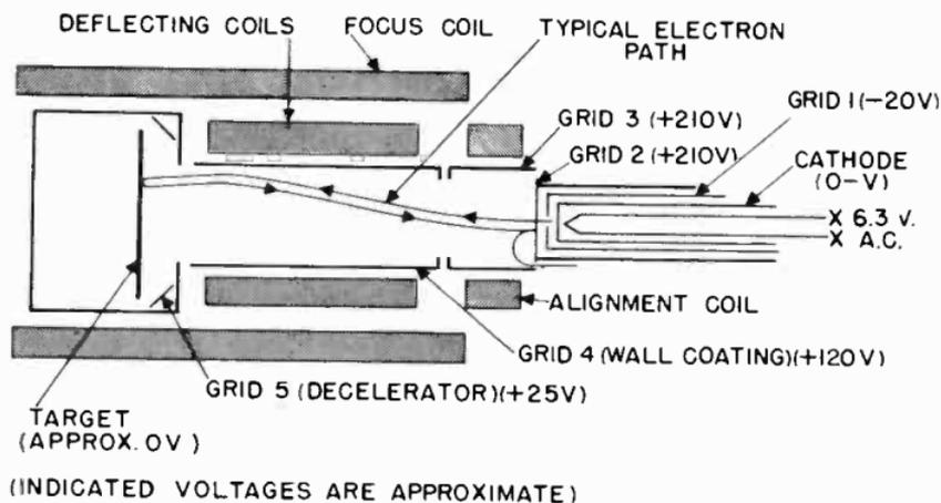
Figure 9. Scanning section of the image orthicon.
