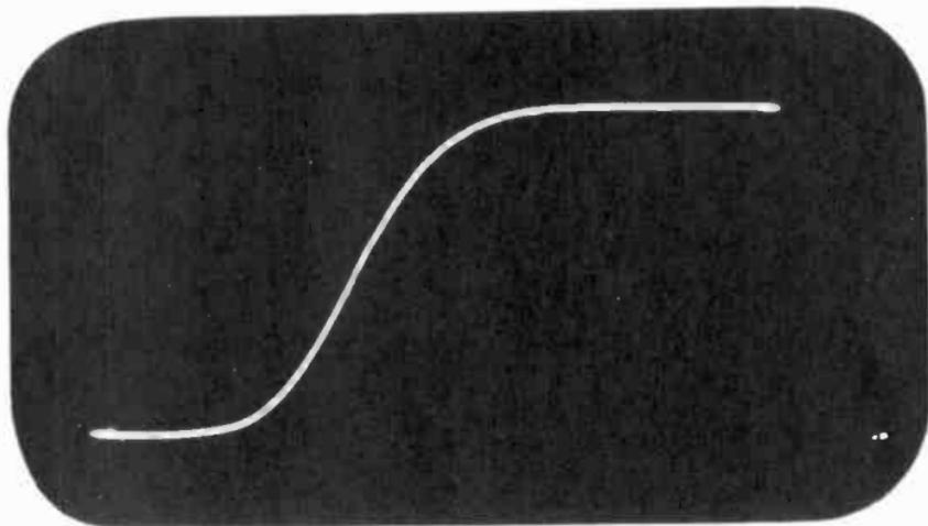
Figure 124. Leading edge of horizontal pulse.
