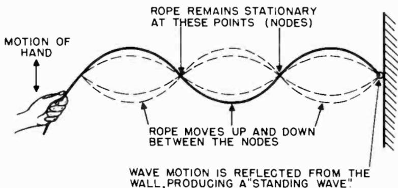
Figure 14. Standing waves produced in a rope.
