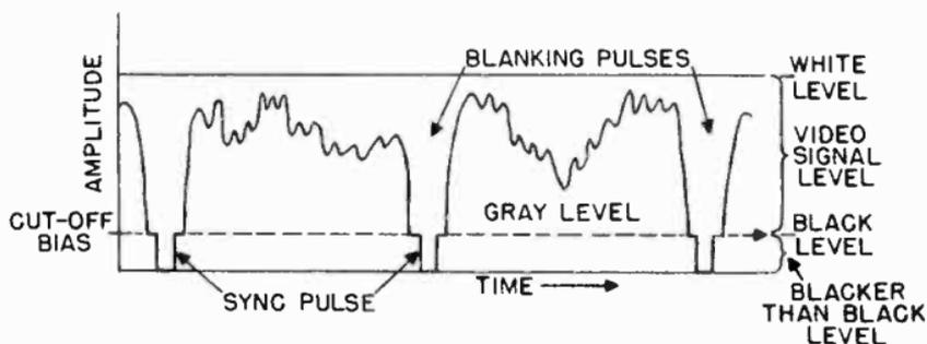
Figure 63. Combined sync, blanking, and video signals.
