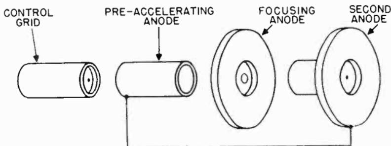
Figure 16. The pre-accelerator electrode is inserted between the control grid and the focusing anode.
