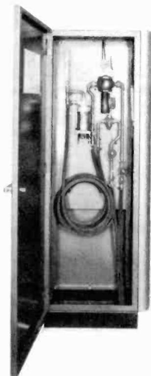
Figure 111. Power output measuring equipment. (courtesy RCA)
