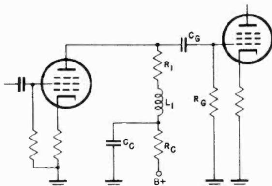
Figure 2. Oscillograph amplifier with high frequency compensation.
