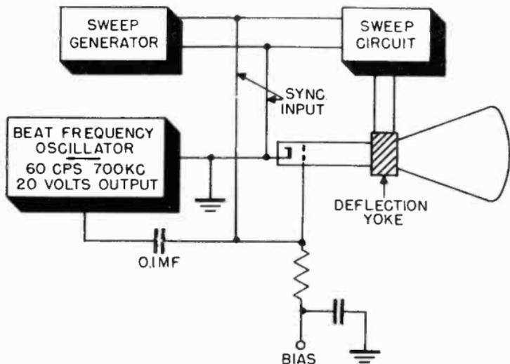
Figure 50. Method used to check linearity of scanning circuits.
