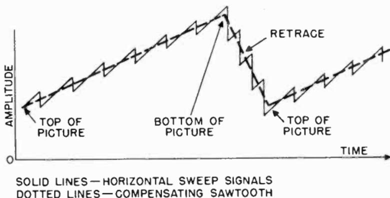
Figure 48. Compensating signal for overcoming keystoneing.
