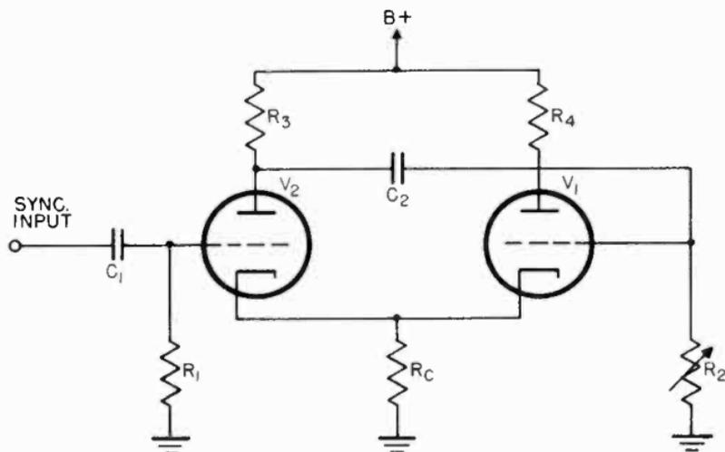
Figure 97. Cathode-coupled multivibration circuit.
