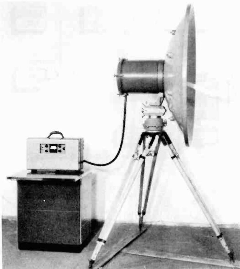
Figure 103. Microwave relay transmitter. (courtesy RCA)
