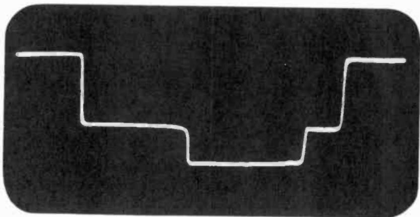
Figure 123. Horizontal blanking and sync pulse.
