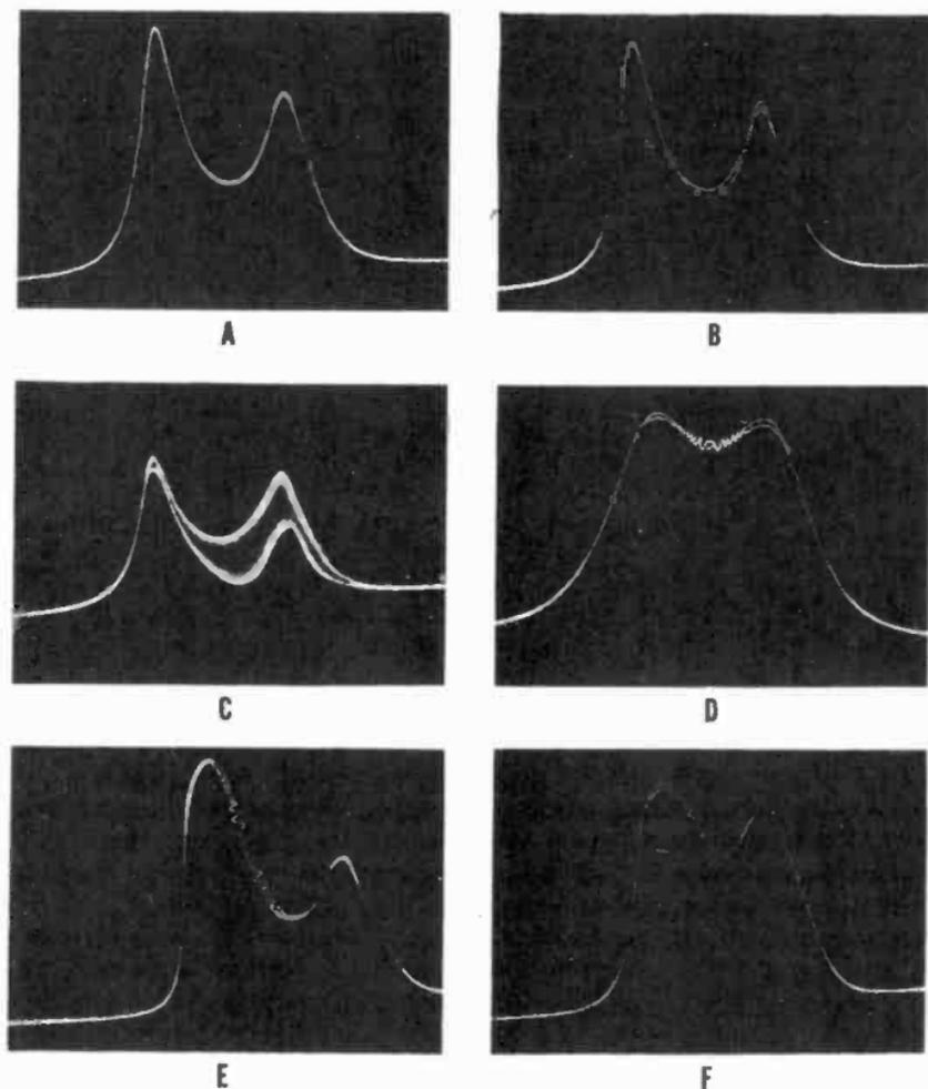
Figure 64. Response curves of sound i-f amplifiers.
