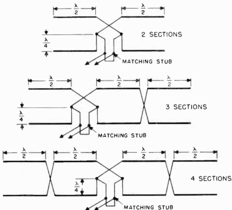
Figure 69. Center-fed flat-top arrays (top view).
