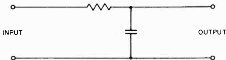
Figure 84. Integrating circuit.
