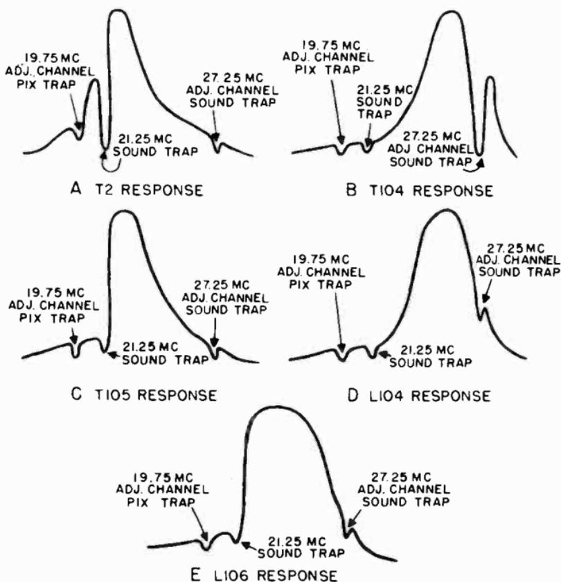
Figure 75. Response curves of stagger-tuned video i-f amplifiers.
