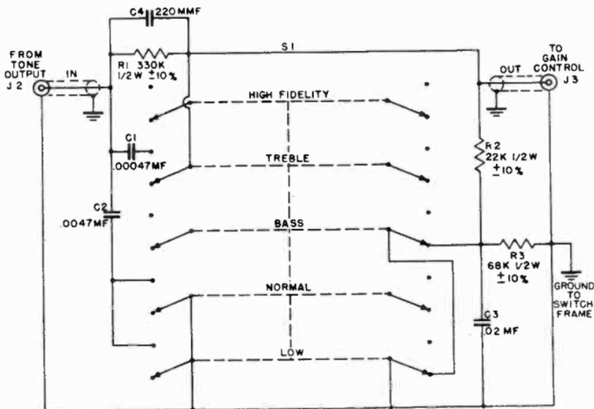
Figure 47. Tone selector schematic.
