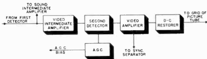
Figure 31. Block diagram of the video channel.
