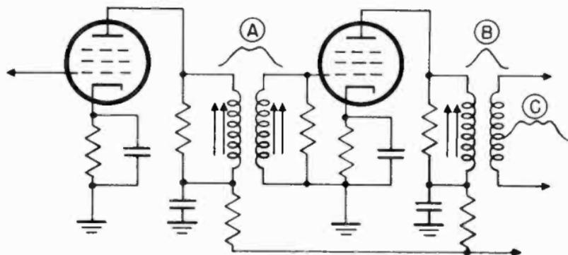
Figure 40. Simplified schematic and response curves of peaked and overcoupled i-f amplifier.
