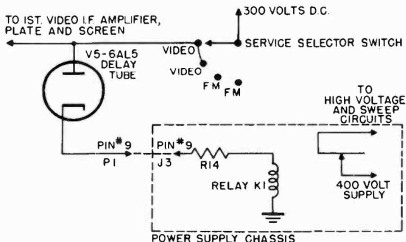
Figure 40. Automatic, high-voltage cutoff circuit.
