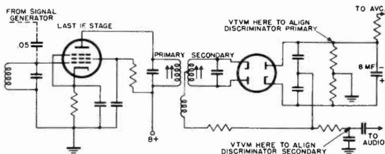
Figure 57. Connections used when aligning ratio detector using v.t.v.m.
