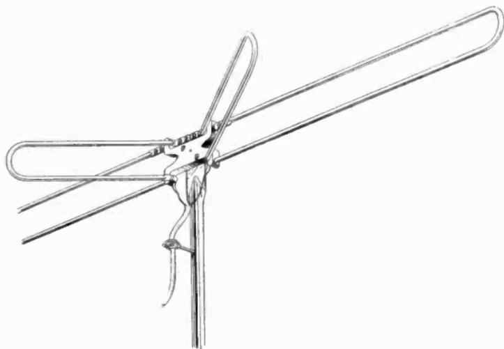
Figure 39. Bat-wing antenna.
