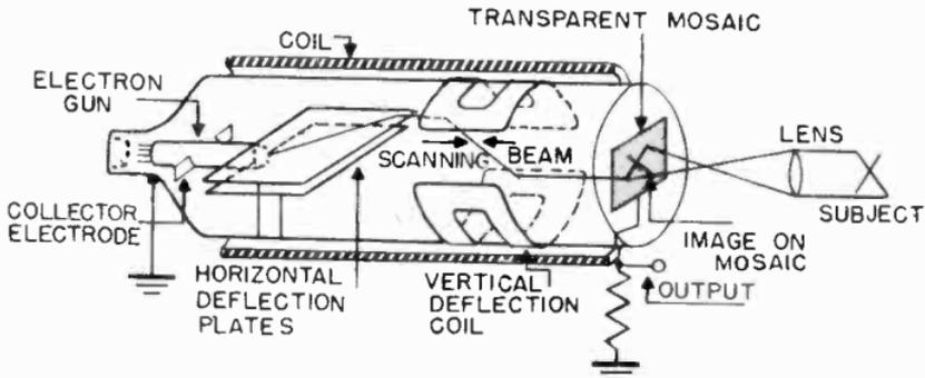
Figure 4. Construction of the orthiconoscope.
