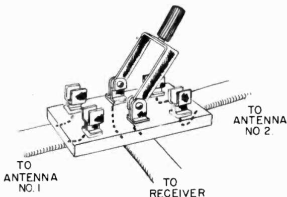
Figure 47. Double-pole, double-throw knife switch for connecting two antennas to receiver.
