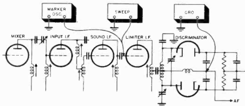
Figure 59. Connections used when aligning discriminator using oscilloscope and sweep generator.
