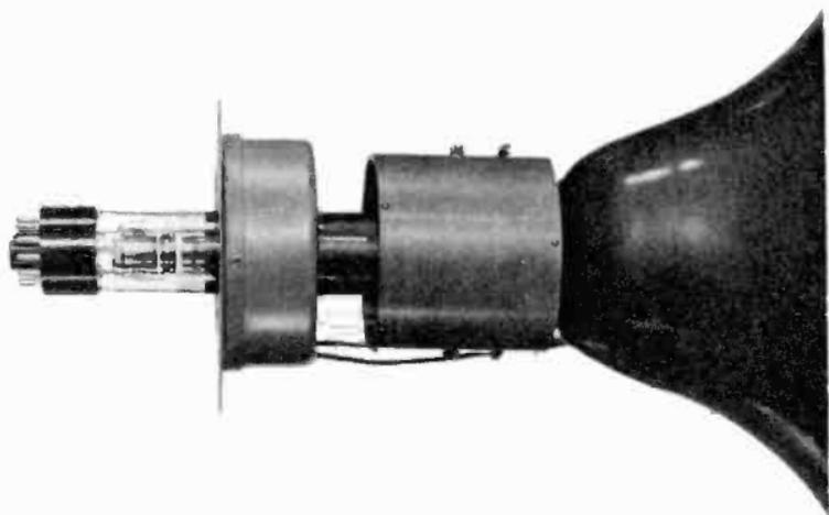
Figure 36. Positions of yoke and focus coils on the neck of a picture tube. (courtesy DuMont)
