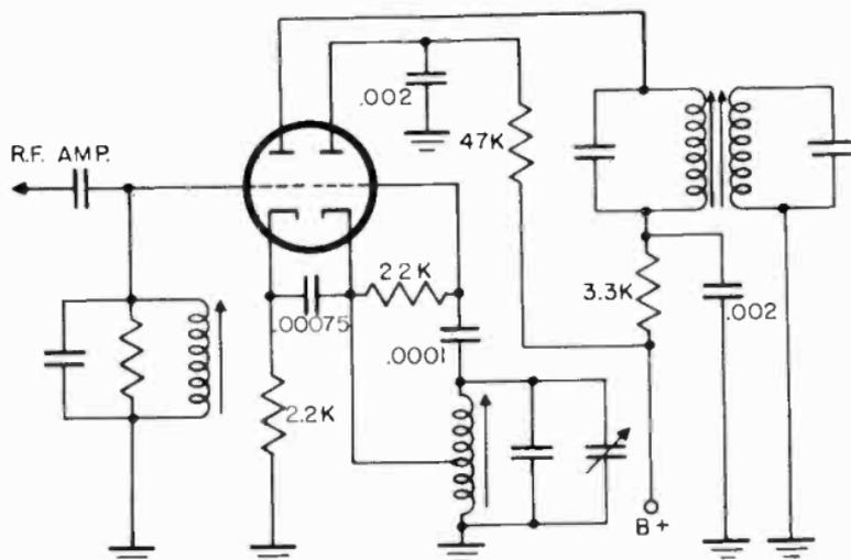
Figure 16. Mixer-oscillator using cathode injection.
