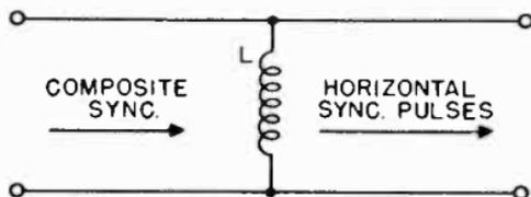
Figure 89. Inductive differentiating circuit.
