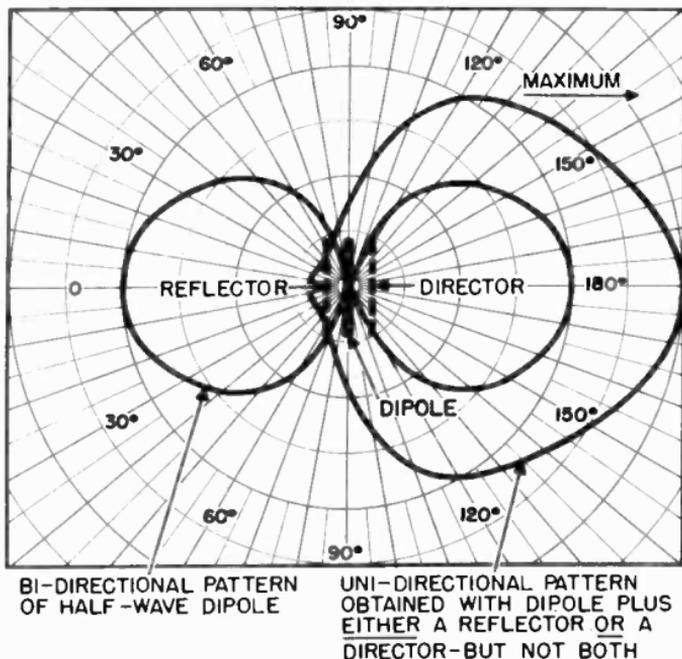
Figure 50. Change in bi-directional field pattern of dipole when either reflector or director is added to dipole.
