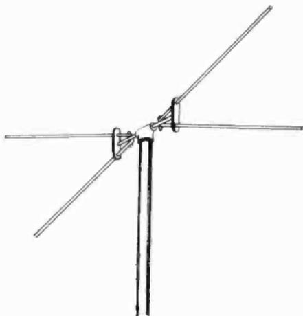
Figure 42. Double-V antenna.
