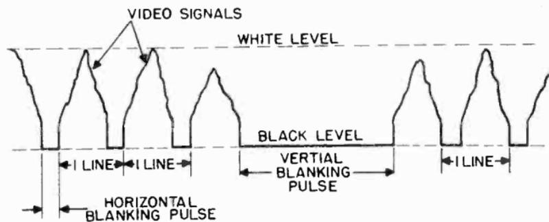
Figure 60. A composite video and blanking signal.
