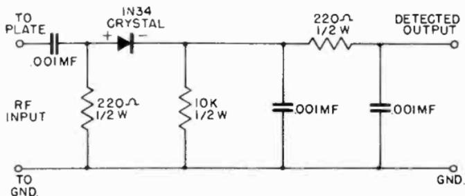
Figure 16. Probe detector.
