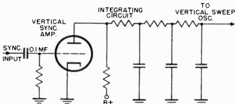
Figure 87. Cascaded integrating circuit.
