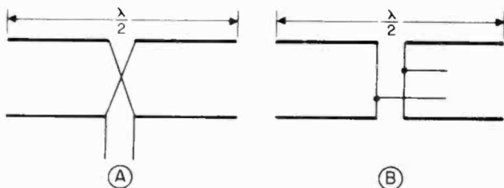
Figure 59. Stacked dipole arrays. (A) center fed; (B) transposed feeder.
