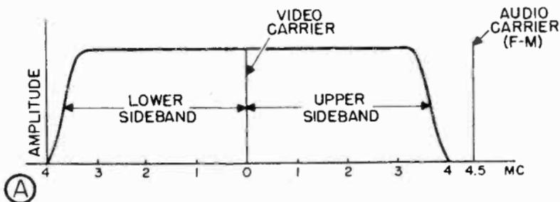
Figure 71A Band of frequencies which would be required for video signal if double side-band transmission were used.
