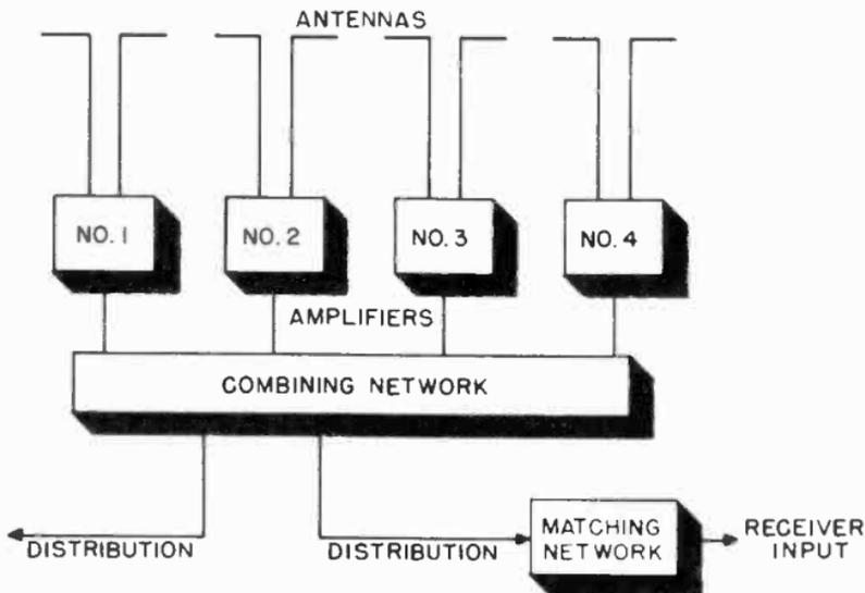
Figure 84. Block diagram of Intra-Video master antenna system.
