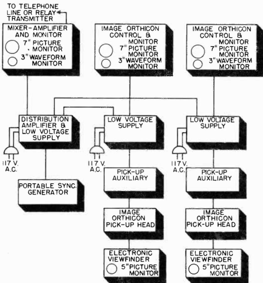
Figure 71. Block diagram of dual image-orthicon camera chain.
