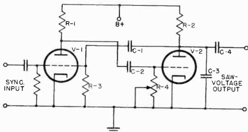
Figure 108. Multivibrator and discharge circuit.
