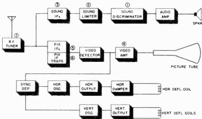
Figure 55. Order in which sound and video circuits are aligned.
