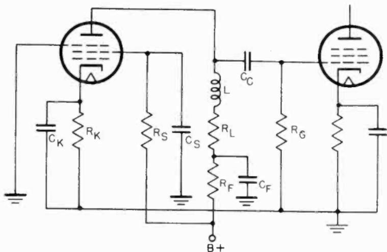
Figure 68. Video amplifier with high and low frequency compensation components.
