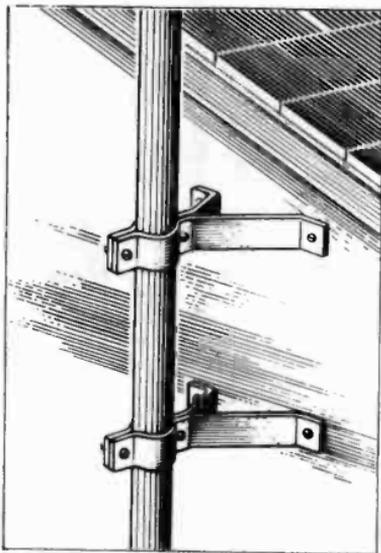
Figure 19. Wall mounting bracket. (courtesy Taco)
