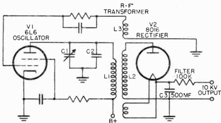
Figure 146. Circuit of an r-f high-voltage power supply.
