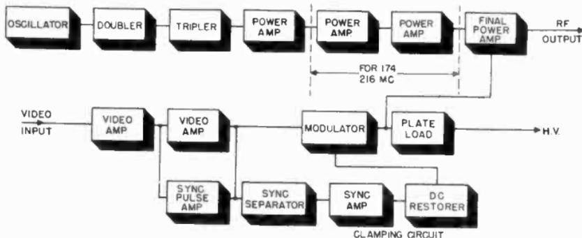
Figure 108. Block diagram of TT-5A transmitter.
