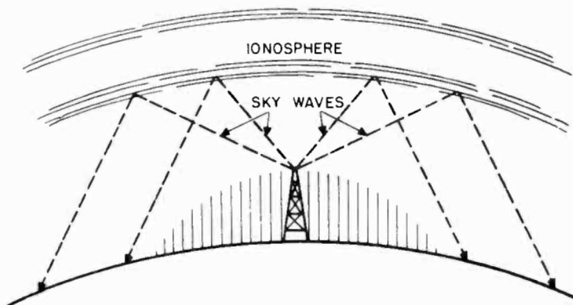
Figure 2. The two principal modes of wave propagation.
