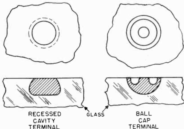
Figure 125. Intensifier terminals.
