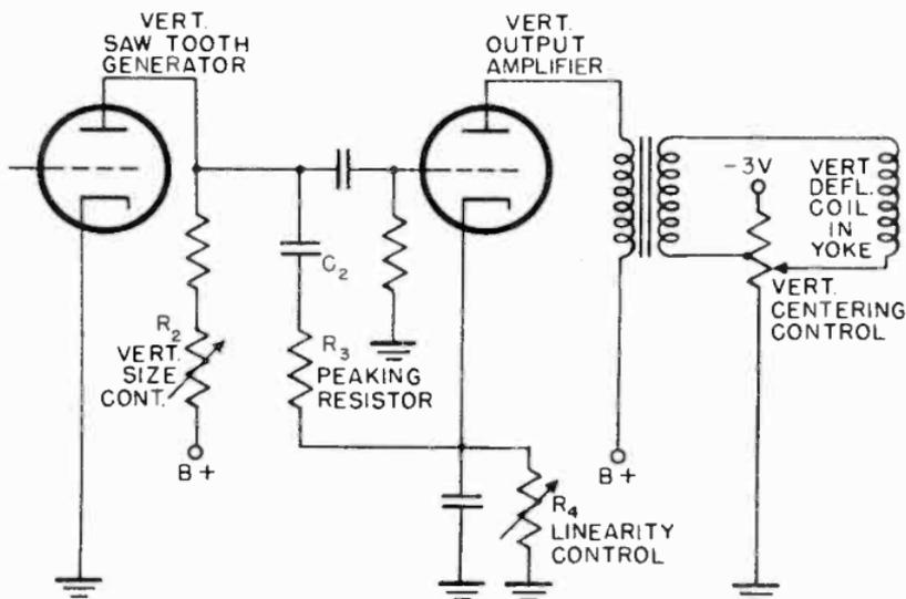
Figure 117. Vertical amplifier circuit.
