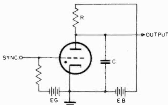
Figure 5. Gas triode sawtooth generator.
