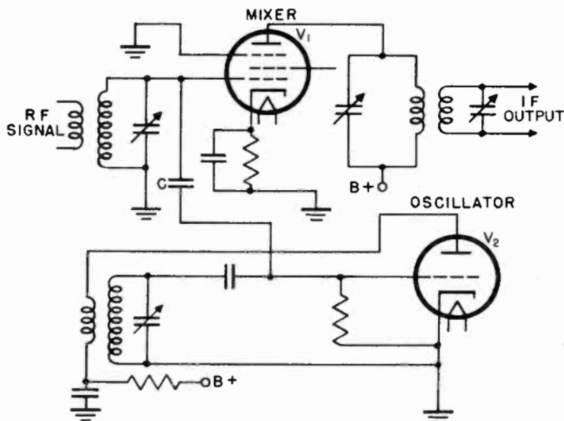
Figure 14. Capacitive-coupled mixer oscillator.
