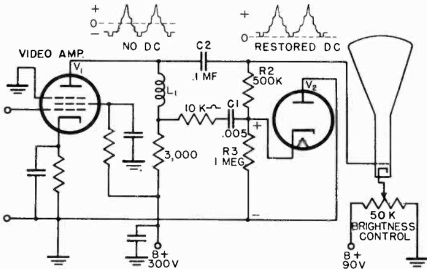
Figure 71. Schematic of diode d-c restorer.
