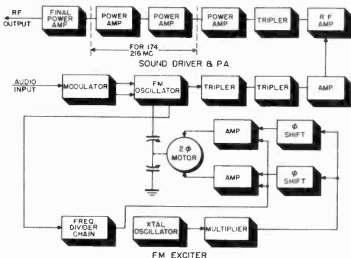
Figure 112. Block diagram of RCA sound transmitter.
