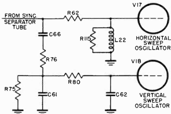
Figure 19. Networks for separating horizontal and vertical sync pulses.
