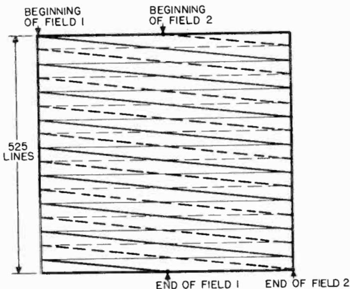
Figure 53B Interlaced scanning pattern.
