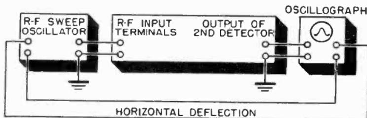
Figure 76. Connections used when aligning r-f section.
