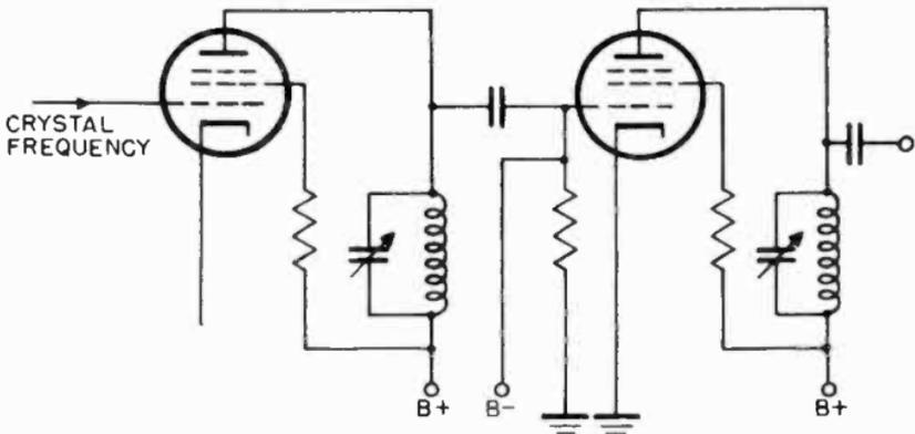
Figure 45. Simplified schematic of frequency multiplying stages.
