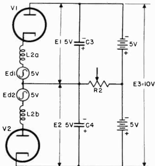
Figure 176. Equivalent circuit of ratio detector.
