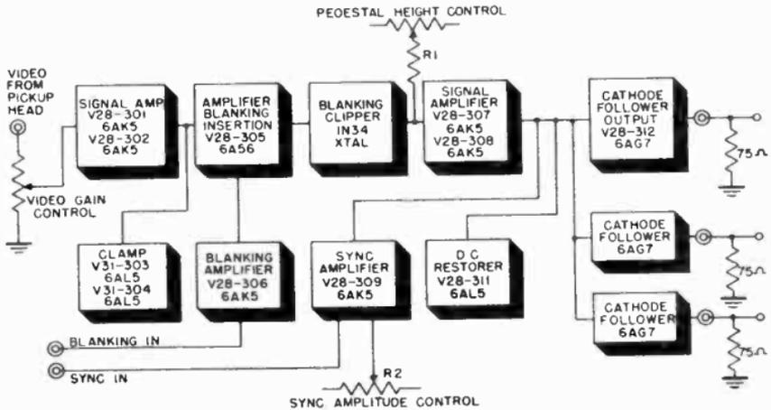
Figure 37. Block diagram of mixing and distribution amplifier.
