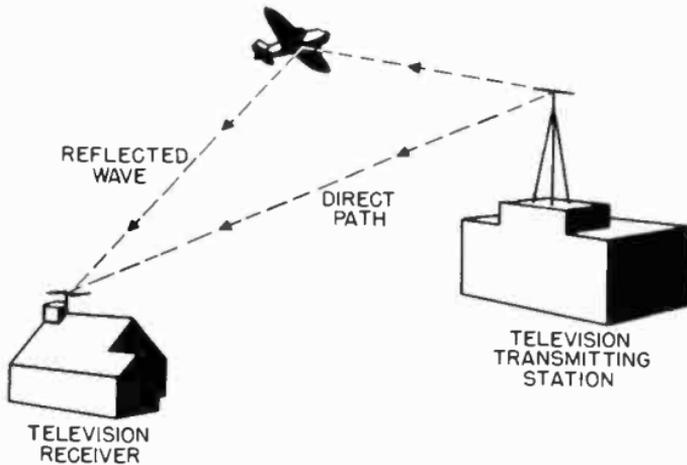
Figure 8. Reflected wave caused by moving airplane.
