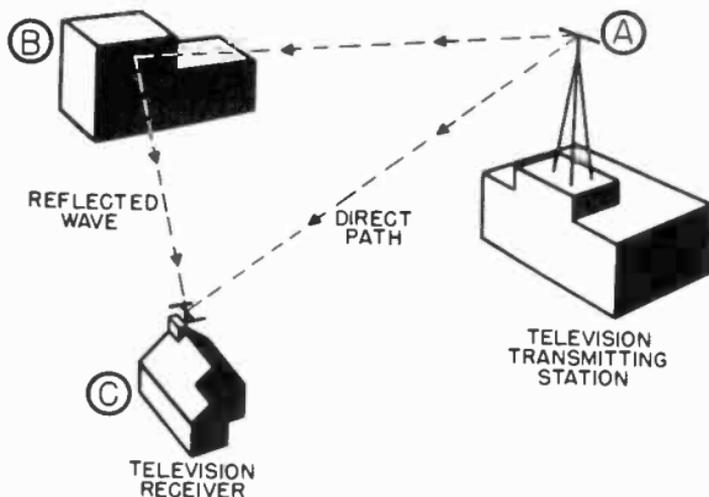
Figure 6. Direct wave and reflected wave striking antenna.
