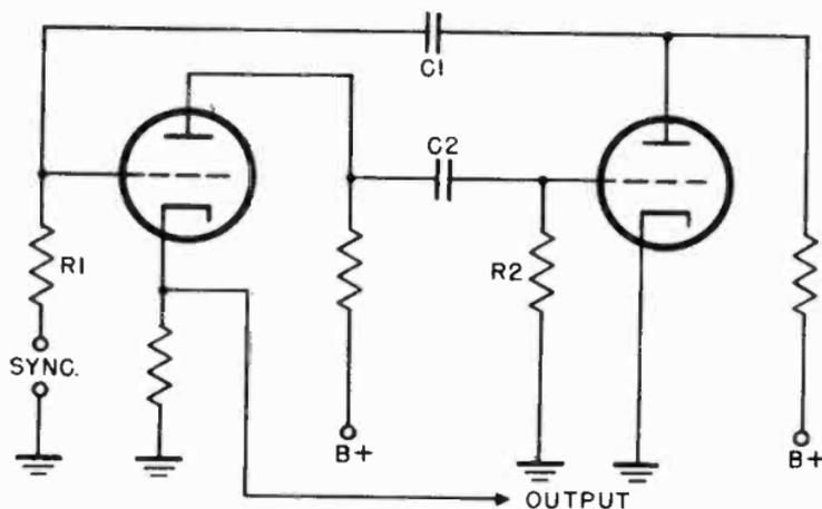
Figure 22. Multivibrator frequency divider.
