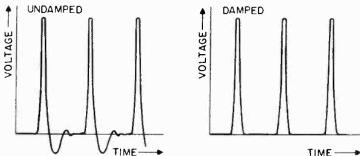
Figure 120. Spurious oscillations which appear across horizontal deflection coil during flyback time.
