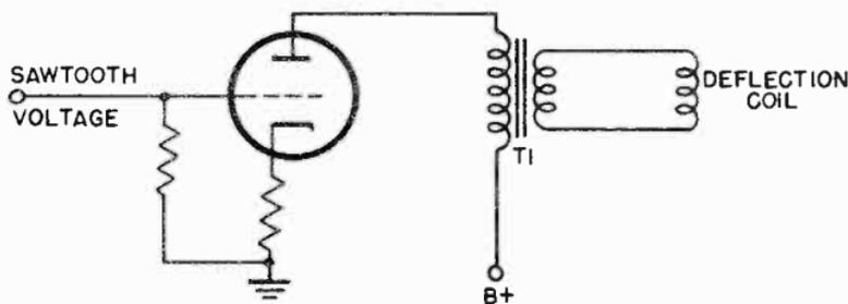
Figure 116. Sweep amplifier for magnetic deflection.
