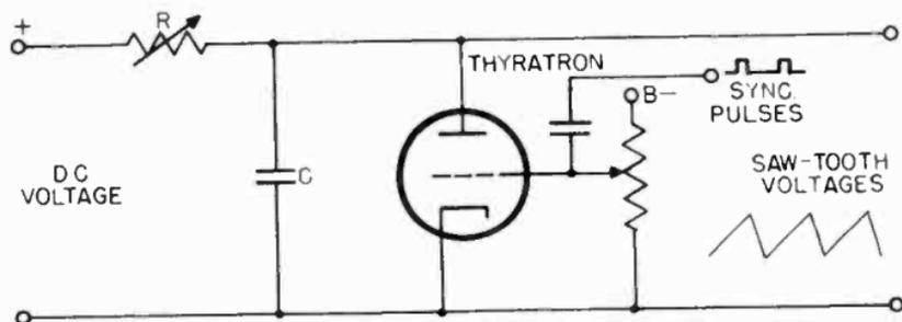
Figure 107. Thyatron saw-tooth generator circuit.
