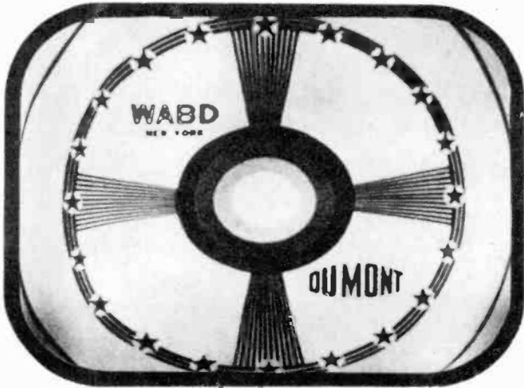
Figure 68A A typical test pattern.
