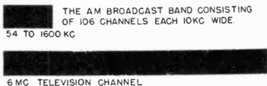
Figure 12. The space occupied in the frequency spectrum by all the a-m stations is less than that allotted to a single television station.
