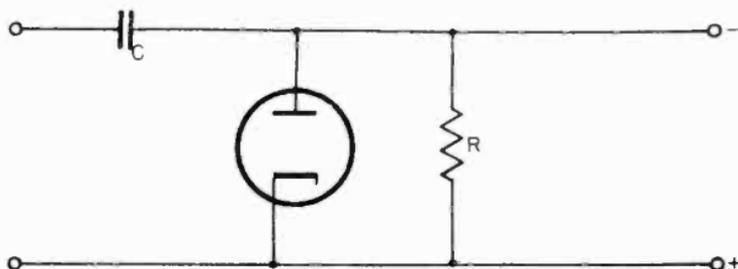
Figure 55. Circuit of diode d-c restoration circuit.
