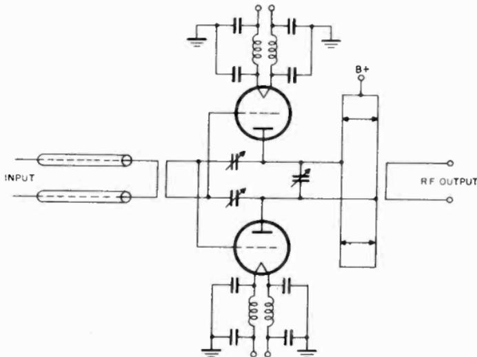
Figure 50. Wideband r-f amplifier circuit.
