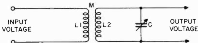
Figure 24. A resonant and coupled coil.
