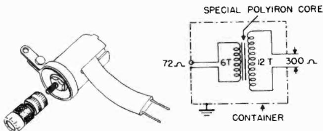
Figure 30. Circuit and appearance of line matching transformer.
