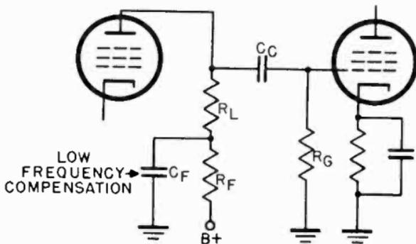
Figure 67. Parallel resistor-capacitor combination for low frequency compensation.
