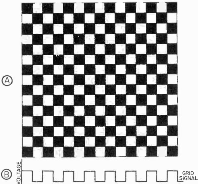
Figure 52. A, checkerboard pattern. Each black and white square is assumed to represent an element in a picture. B, grid voltage which is required to produce checkerboard pattern on the screen of the picture tube.
