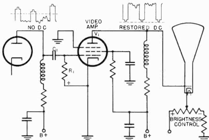
Figure 72. D-C restoration in the video amplifier stage.
