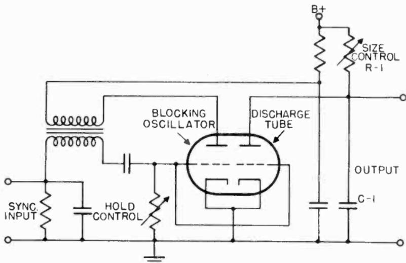
Figure 110. Blocking oscillator discharge circuit using dual triode.
