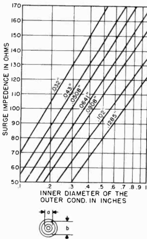
Figure 19. Characteristic impedance of coaxial transmission lines.
