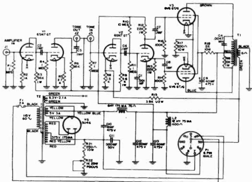
Figure 46. Audio amplifier schematic.
