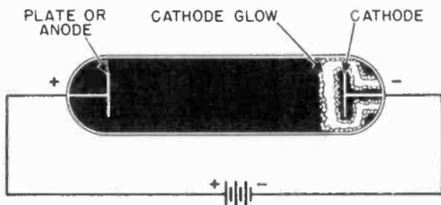
Figure 1. Plucker's simple gas tube.
