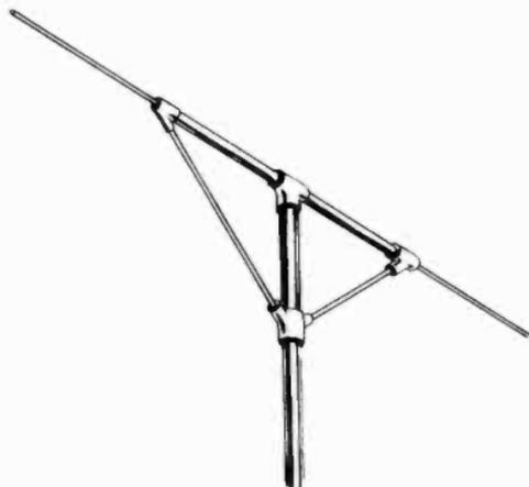
Figure 32. Extended V antenna.
