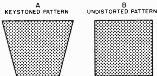
Figure 47. A shows a keystone pattern. B shows correct scanning pattern, obtained on mosaic when keystone distortion is eliminated.
