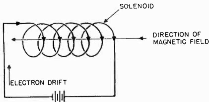
Figure 24. Direction of magnetic field in a solenoid.
