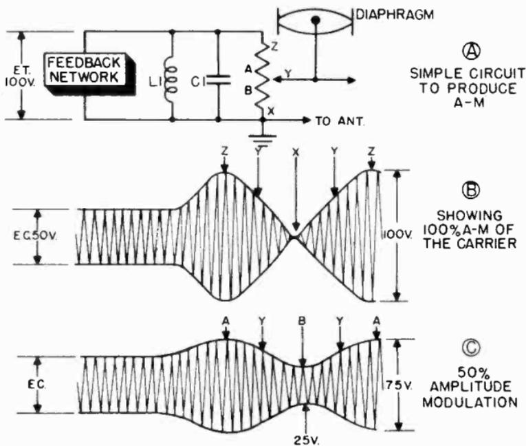
Figure 157. Simple method of amplitude modulation.
