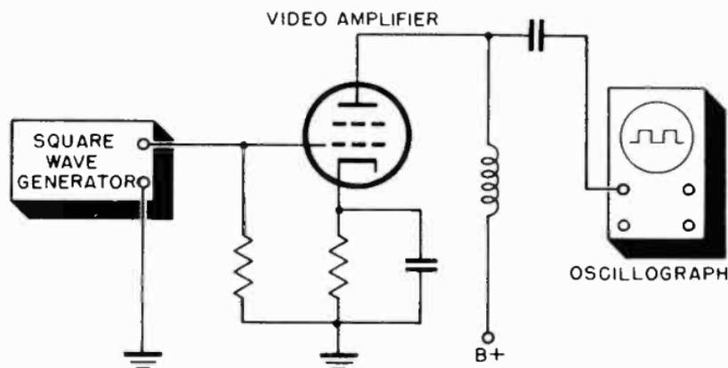
Figure 67. Connections used to adjust video amplifier using square wave generator and oscillograph.
