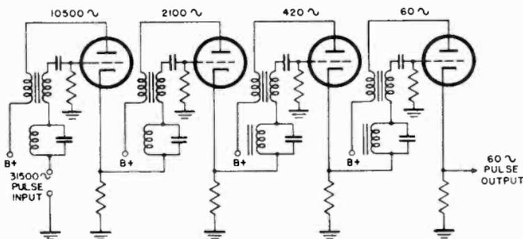
Figure 26. Frequency divider chain.
