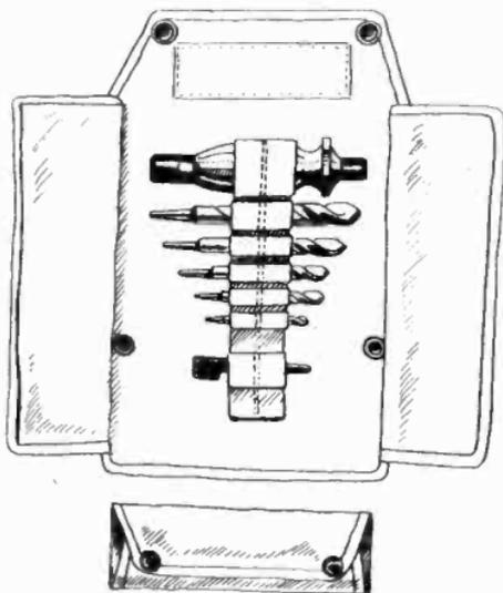
Figure 9. Masonry drill kit.
