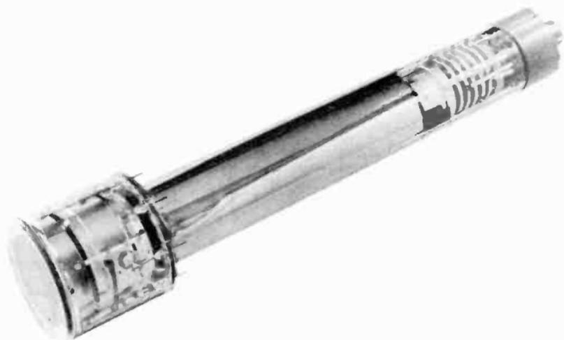
Figure 5. The image orthicon. (courtesy RCA)
