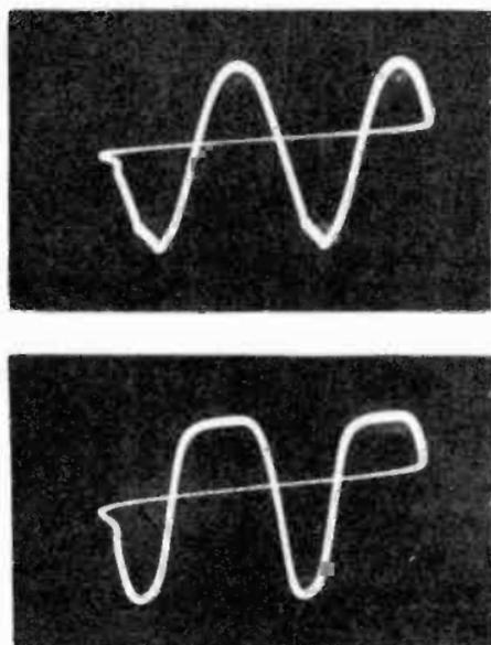
Figure 101. Signals on grid and plate of Hartley oscillator operating at low plate voltage.
