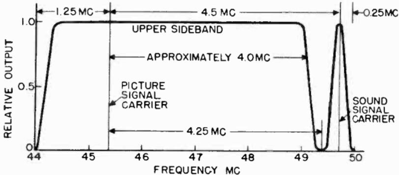
Figure 40. Single sideband television signal.
