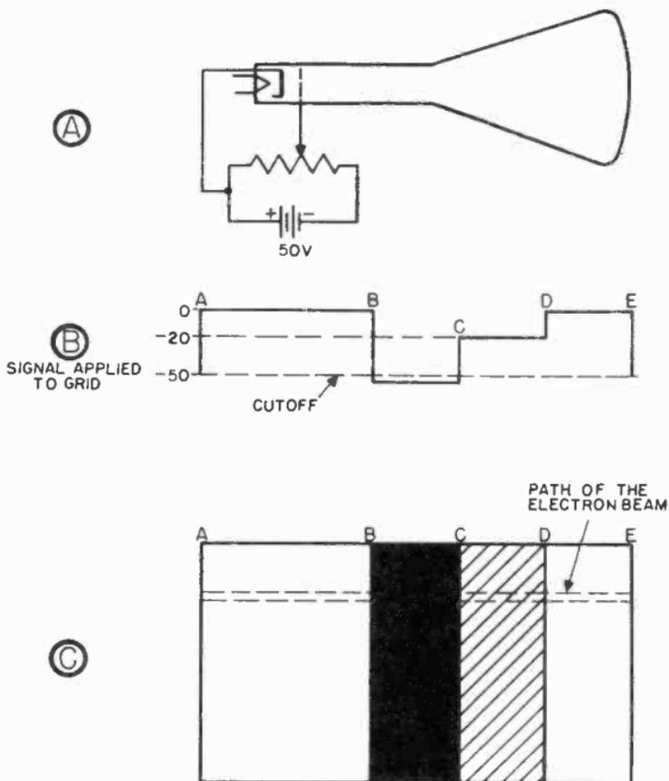
Figure 37. Forming an image on the screen.
