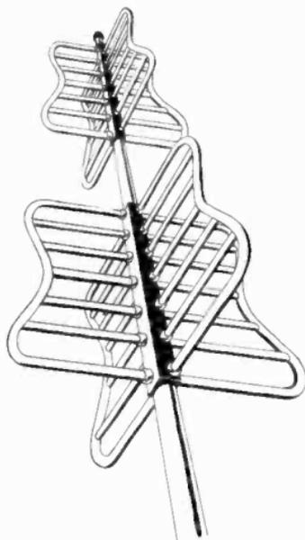
Figure 78. Super-turnstile antenna.
