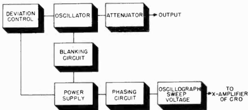
Figure 9. Block diagram of fundamental frequency wobblator.
