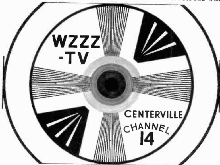
Figure 12. Pattern obtained from monoscope tube.
