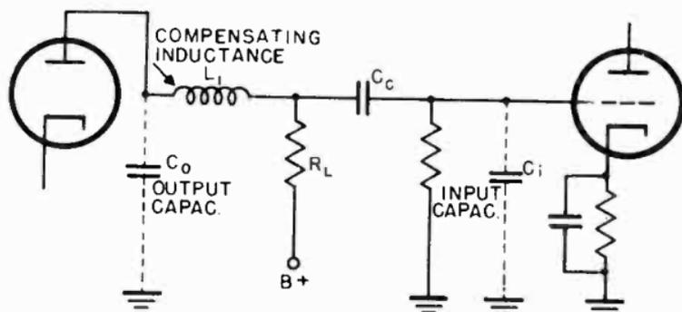
Figure 64. Series-peaking frequency compensation.
