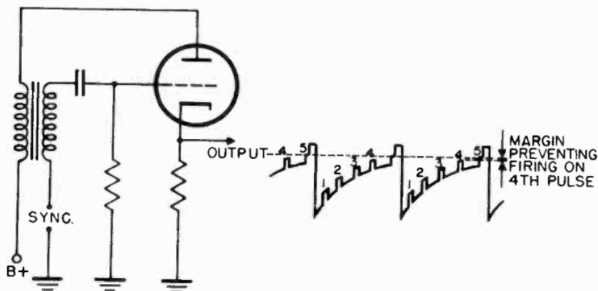
Figure 23. Blocking oscillator frequency divider.
