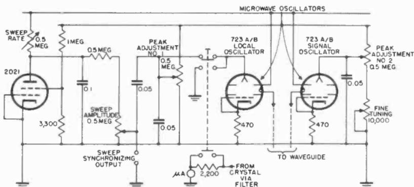
Figure 15. Basic schematic circuit of Mega-Sweep.
