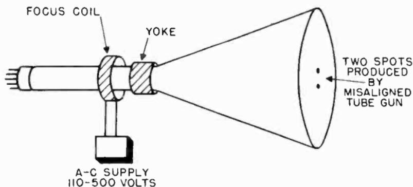
Figure 49. Method used to align focus coil using 60-cycle supply.
