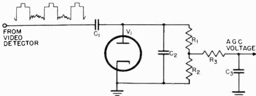
Figure 75. Simplified diagram of a.g.c. circuit.
