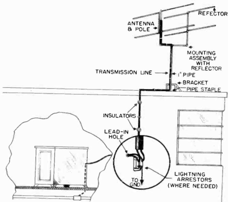
Figure 33. A typical installation.
