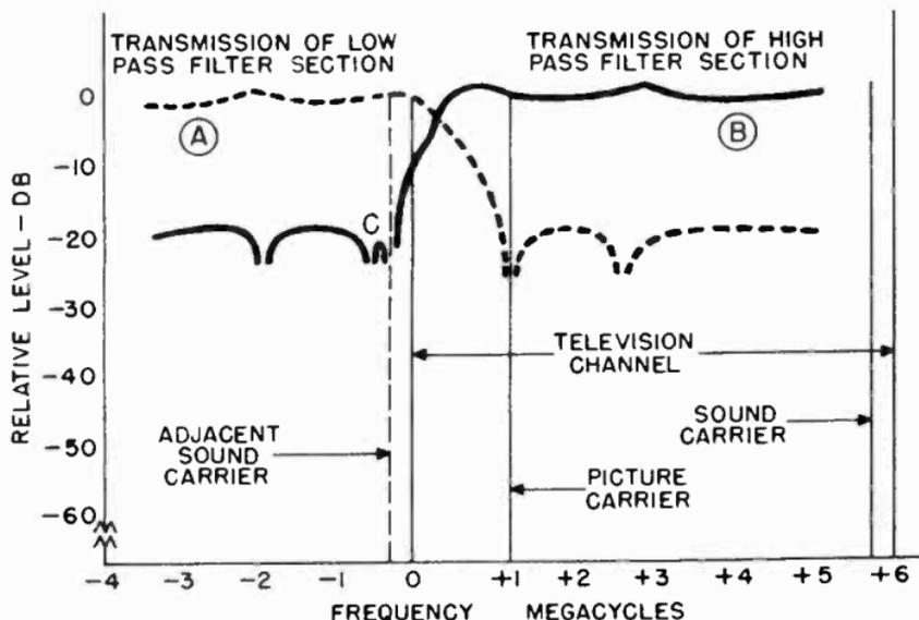
Figure 48. Transmission characteristics of vestigial sideband filter.
