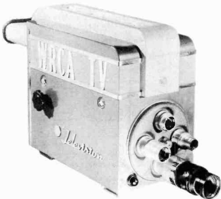
Figure 6. Image orthicon camera. (courtesy RCA)
