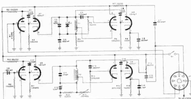
Figure 18. Schematic circuit of Crosshatch Generator
