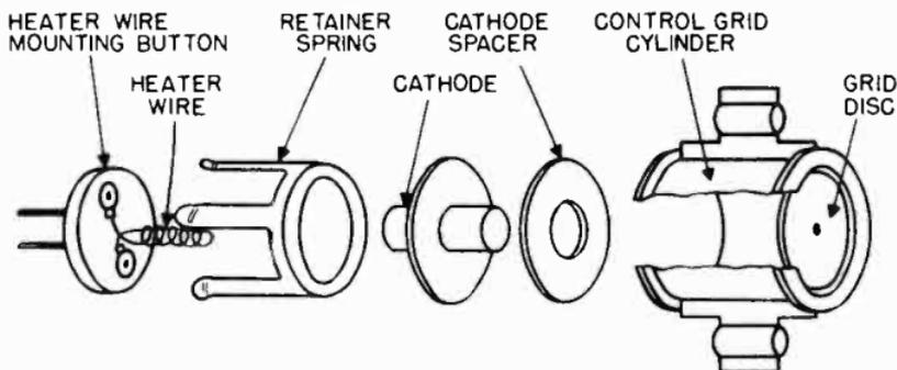
Figure 6. The cathode-grid assembly.
