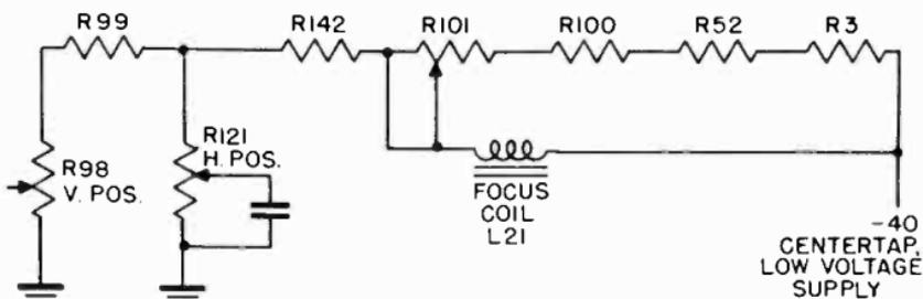
Figure 36. Focus coil circuit.
