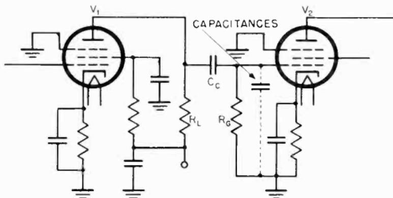
Figure 61. Simplified schematic of resistance coupled amplifier.
