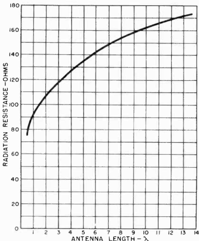
Figure 73. Radiation resistance of long-wire antenna.
