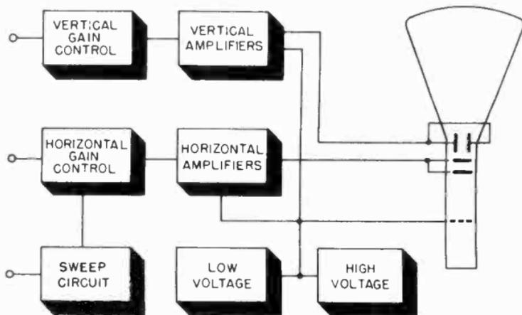
Figure 1. Block diagram of cathode-ray oscilloscope.
