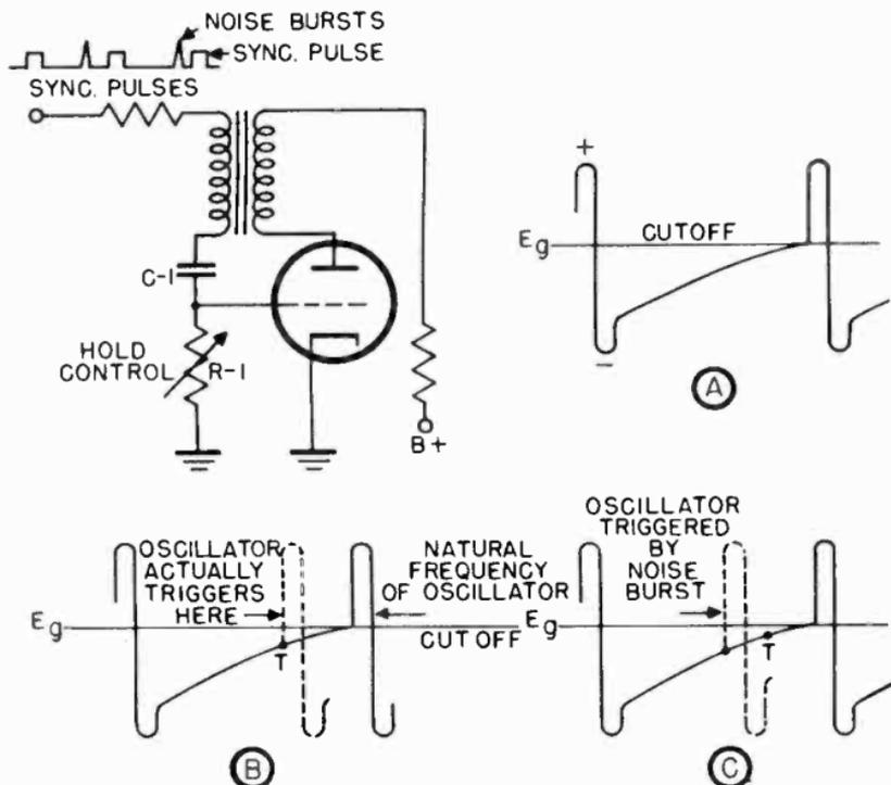
Figure 98. How noise affects the operation of blocking oscillator circuit.
