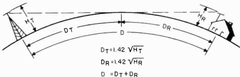
Figure 3. Radio horizon distance between transmitter and receiver.
