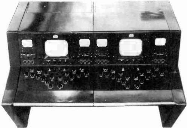
Figure 97. Iconoscope film camera monitor showing shading controls. (courtesy DuMont)
