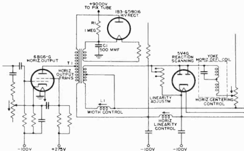
Figure 154. Typical kickback high-voltage supply used in a television receiver.
