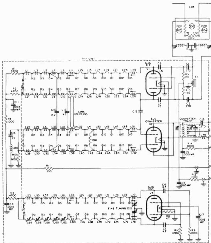
Figure 2. Schematic diagram of RCA tuner.
