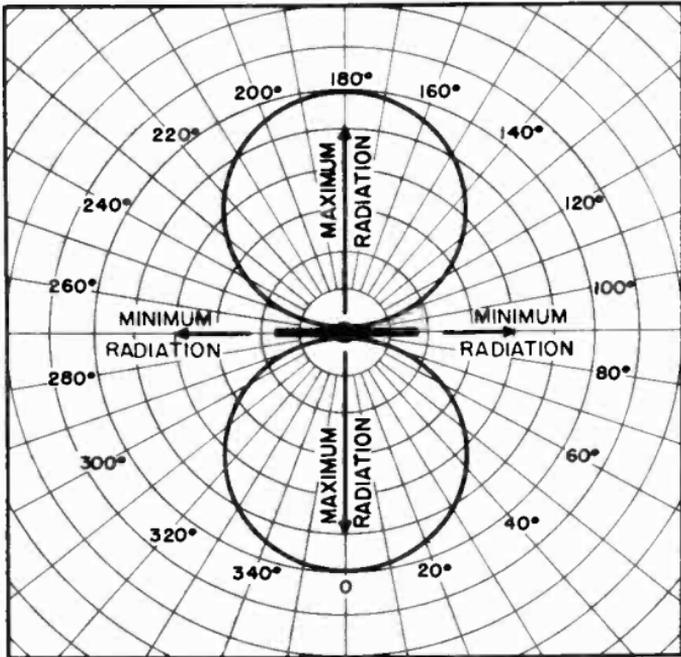
Figure 27. Horizontal field pattern of horizontally polarized half-wave dipole.
