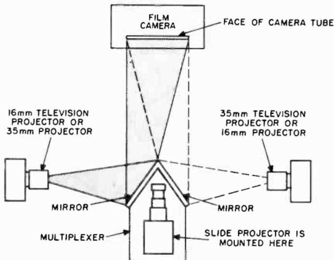
Figure 99. Physical layout of film multiplexer.
