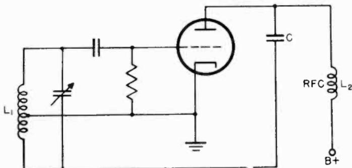
Figure 9. Shunt-fed Hartley oscillator.
