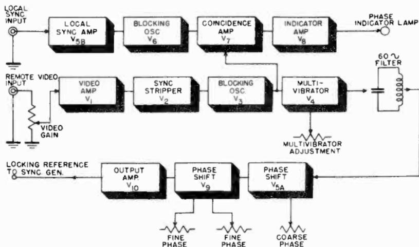
Figure 68. Block diagram of sync phasing unit.
