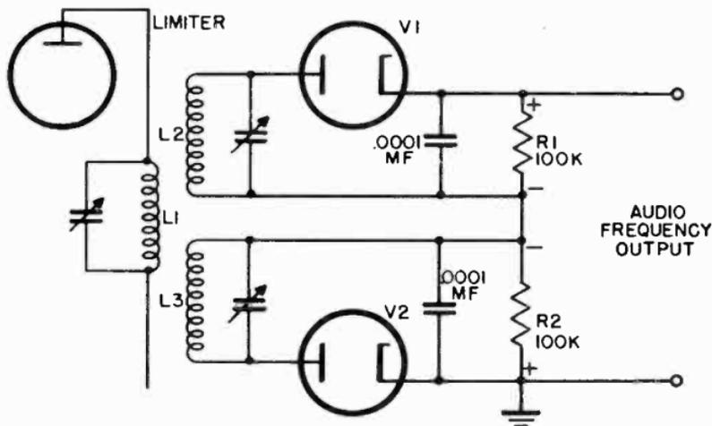
Figure 170. Simple discriminator circuit.
