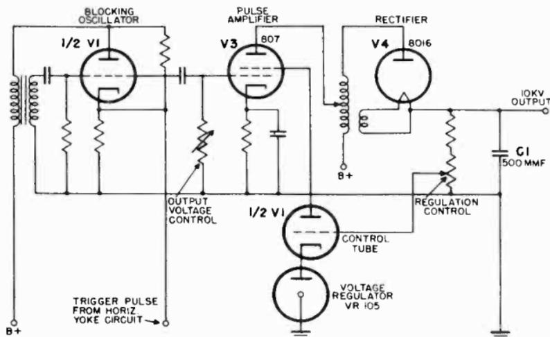
Figure 152. Regulated pulse type supply.
