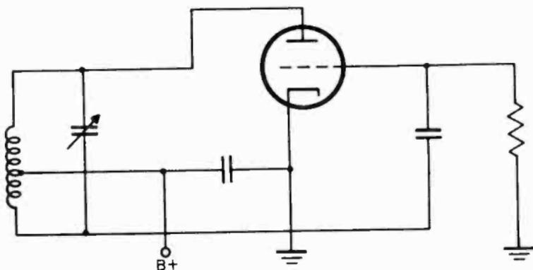
Figure 10. Series-fed Hartley oscillator.
