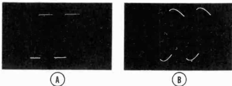
Figure 69. Square wave patterns obtained when checking low-frequency response of video amplifier. A. Good low-frequency response, B. Poor low-frequency response.
