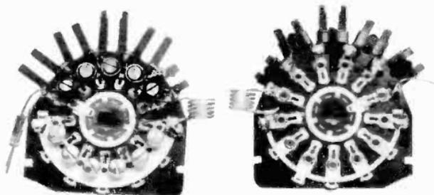
Figure 3. Wafer switches and coils used in RCA tuner. (courtesy RCA)
