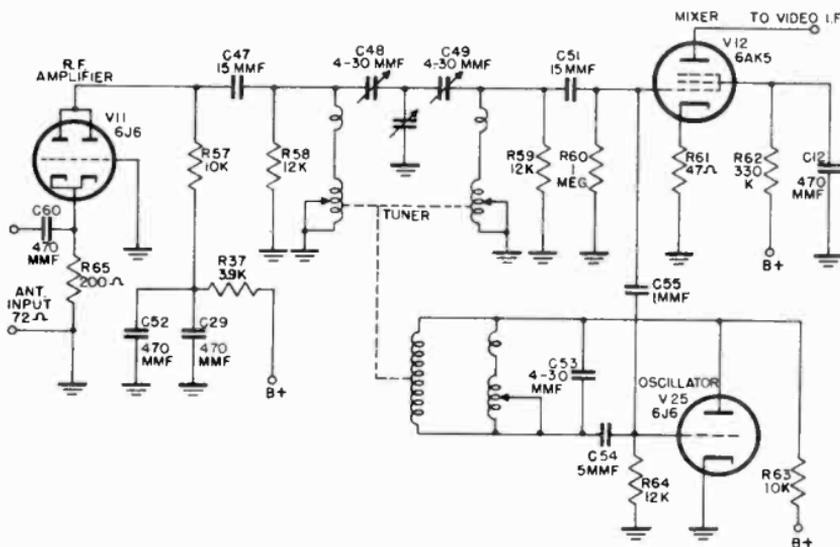
Figure 12. Schematic diagram of Inputuner.
