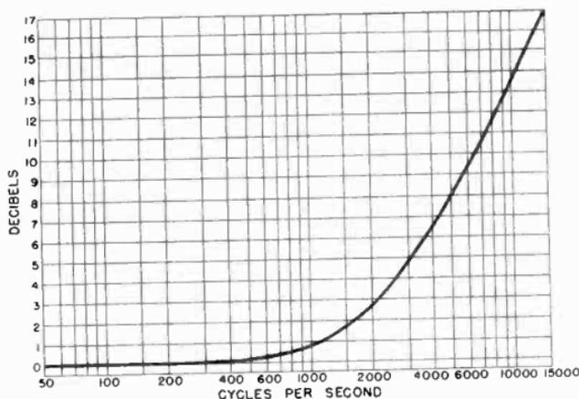
Figure 178. Response characteristic of pre-emphasis filter.
