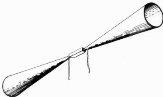
Figure 46. Conical antenna.
