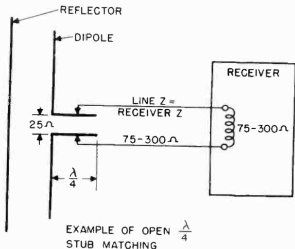
Figure 23. Quarter-wave stub matching section.
