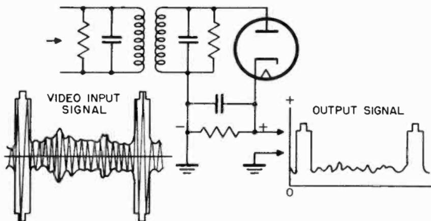
Figure 53. Diode detector and waveform.
