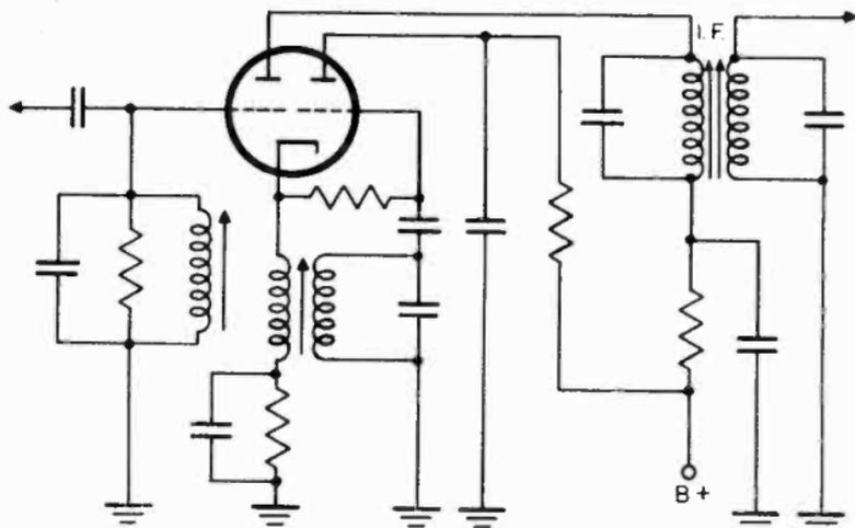
Figure 18. Mixer-oscillator using dual triode with common cathode.
