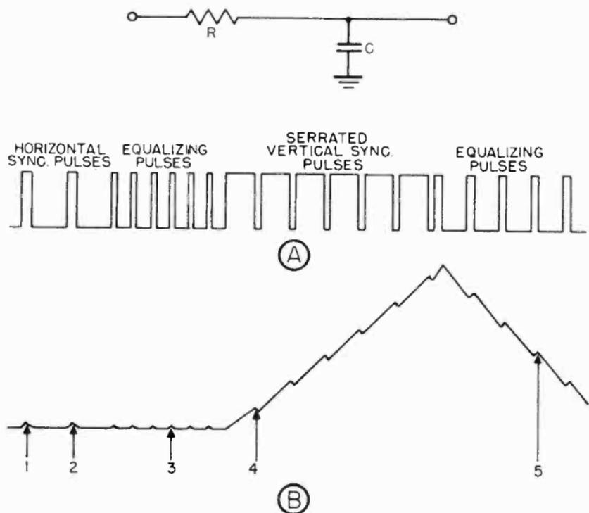
Figure 86. Input and output waveforms of integrating circuit.
