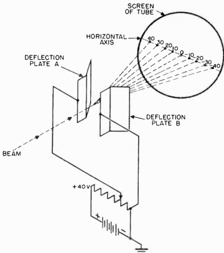
Figure 28. The electron beam is moved horizontally when a d-c potential is applied to the horizontal deflection plates.
