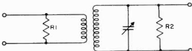
Figure 26. Transformer shunted with resistors to flatten and broaden its response.
