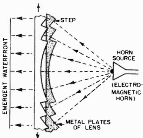
Figure 83. Focusing effect of metal plates of "stepped" construction.
