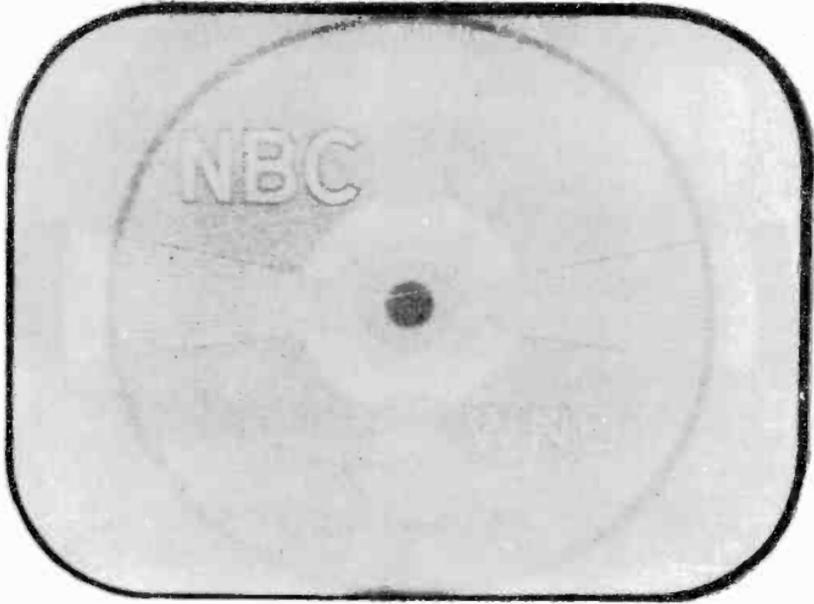
Figure 67A Insufficient contrast.
