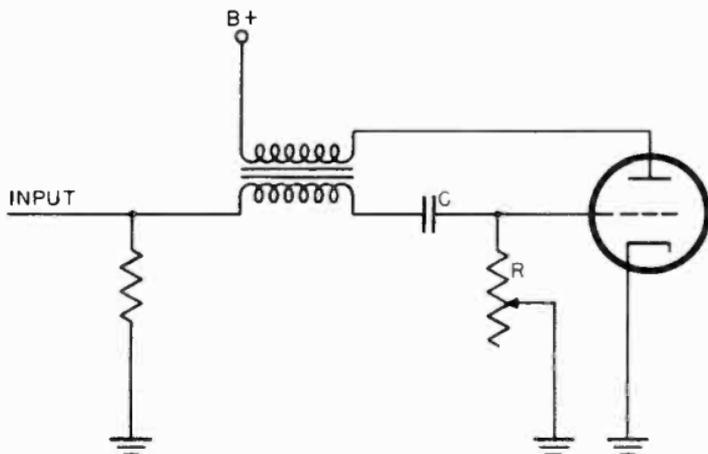
Figure 93. Blocking oscillator circuit.
