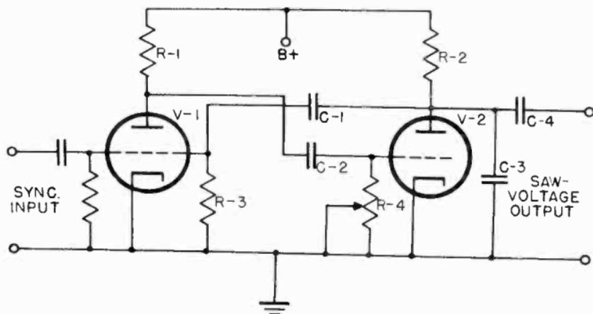
Figure 96. Multivibration circuit.
