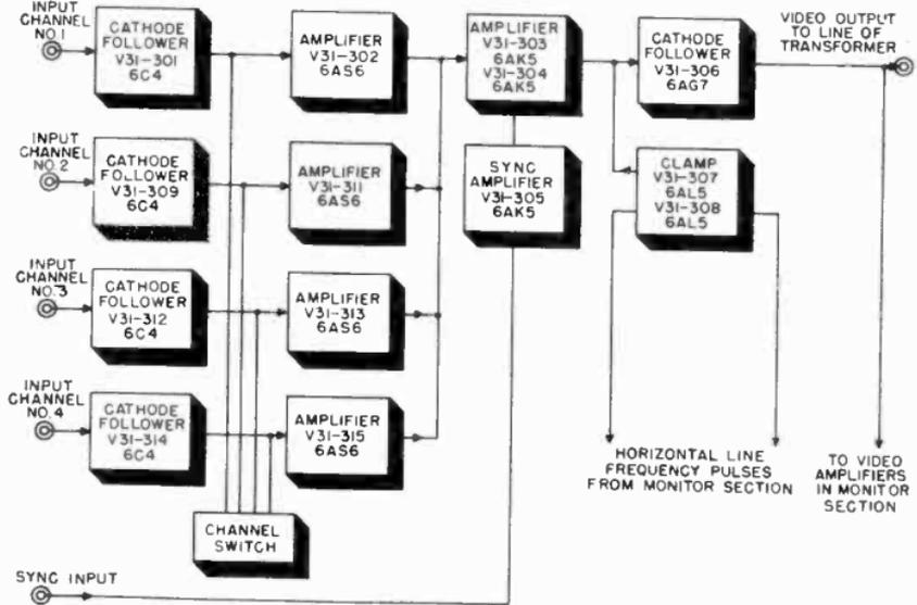
Figure 77. Block diagram of mixer amplifier.
