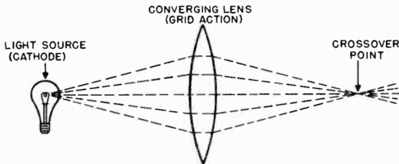
Figure 15. The focusing of an electron beam is similar to the action of a lens on a beam of light.
