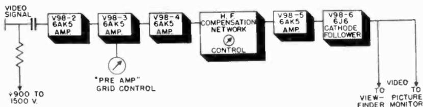
Figure 16. Block diagram of video amplifier used in image orthicon camera.
