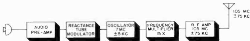
Figure 161. Block diagram of f-m transmitter.
