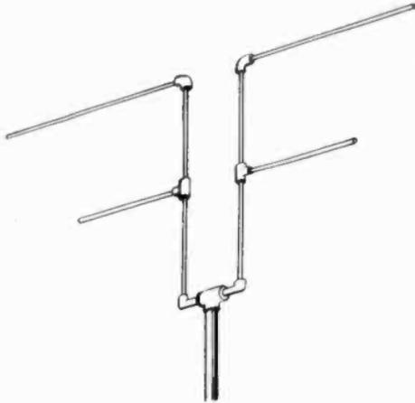
Figure 63. Stub-tuned stacked array.
