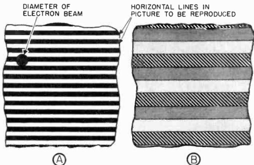
Figure 65 Magnified portion of a picture containing 1,000 horizontal black lines.
