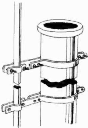
Figure 20. Bracket for mounting on vent pipe.
