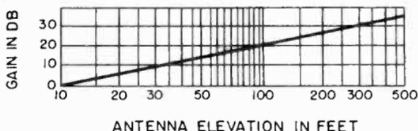
Figure 5. Gain in field intensity of a horizontally polarized dipole antenna when it is raised from low elevation.
