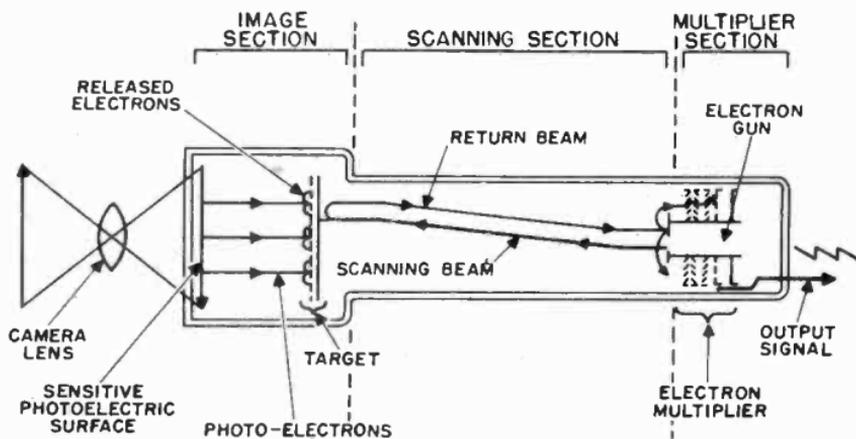
Figure 7. Construction of the image orthicon.
