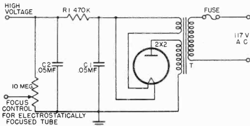
Figure 145. Circuit of a 60-cycle, high-voltage supply.
