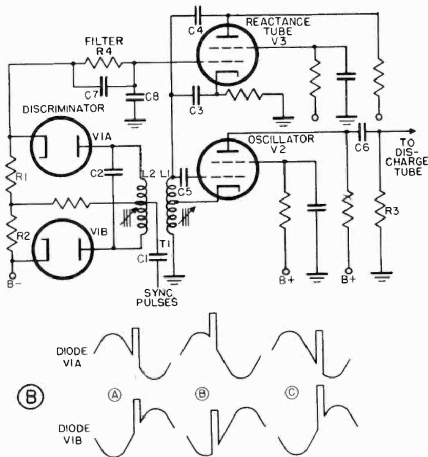
Figure 100. Automatic frequency control circuit which eliminates need for manual hold control.
