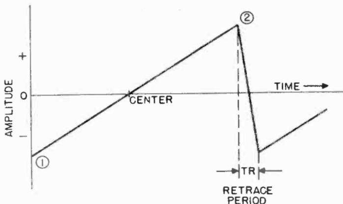
Figure 54. Sawtooth scanning voltage.
