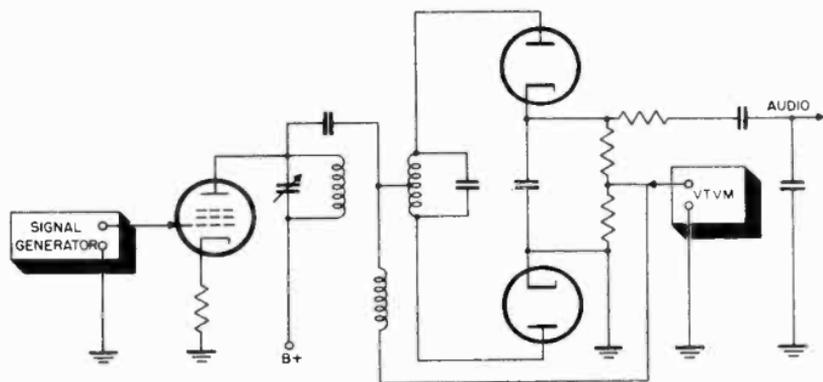
Figure 62. Connections used when checking limiter performance.
