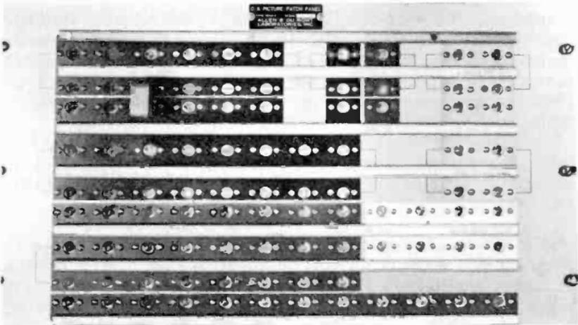
Figure 67. On-the-Air patch panel. (courtesy DuMont)
