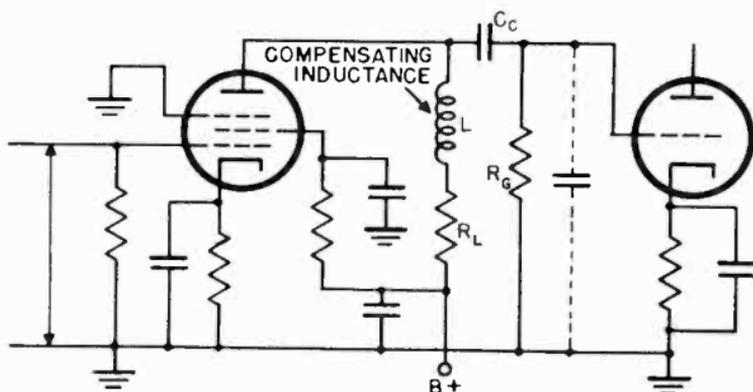
Figure 63. Shunt-peaking frequency compensation.
