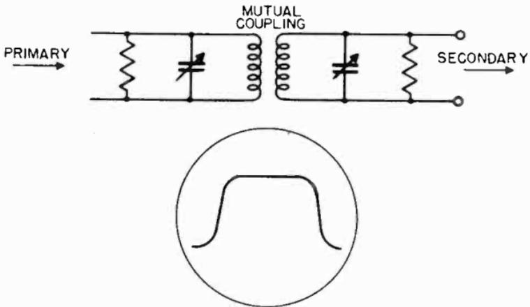
Figure 49. Overcoupled circuit and its response characteristic.
