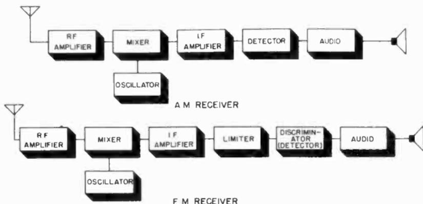
Figure 156. Block diagrams of conventional superhet and f-m receiver.
