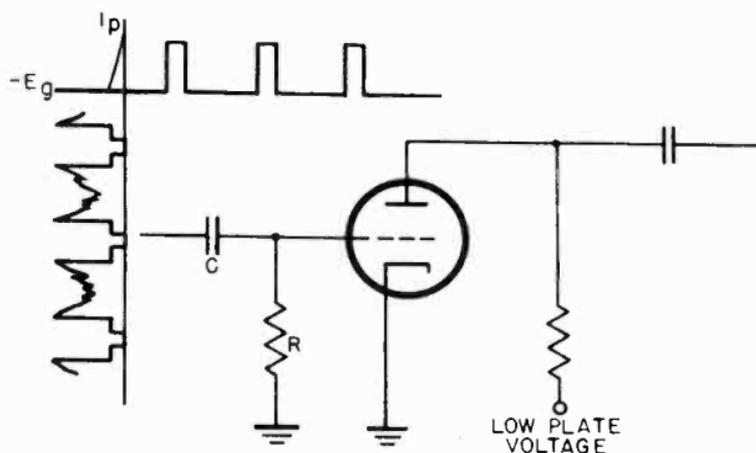
Figure 82. Simplified schematic of triode sync clipper.
