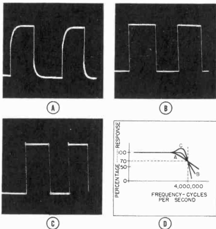
Figure 68. Patterns obtained on oscillograph when checking high frequency response of video amplifier.
