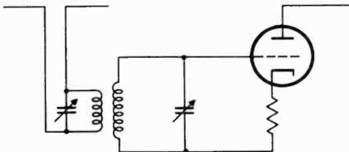
Figure 29. Antenna coupling circuit using tuned primary and secondary.
