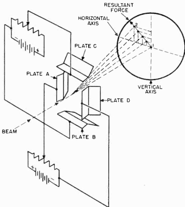
Figure 29. The horizontal and vertical deflection plates, with separate sources of voltage connected to them.
