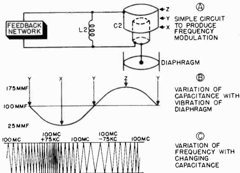
Figure 158. Simple method of frequency modulation.
