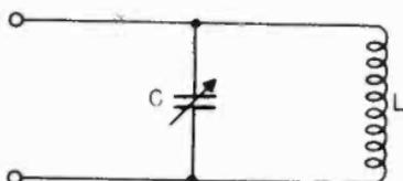
Figure 22. A parallel resonant circuit.
