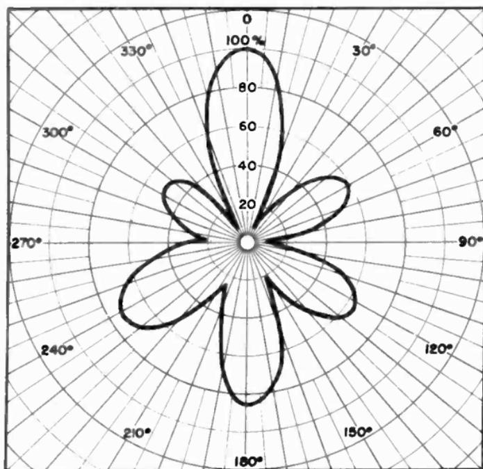
Figure 38. Horizontal field pattern of duo-dipole antenna at 195 Mc.
