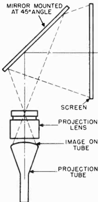
Figure 133. Refractive projection system.
