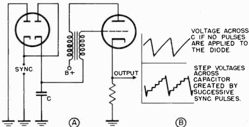
Figure 25. Pulse counting circuit.
