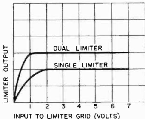
Figure 168. Comparison of single and dual limiter.
