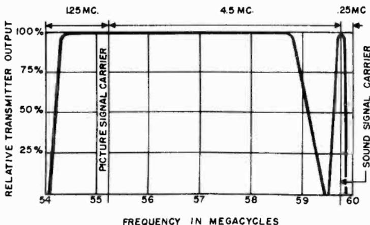
Figure 4. A typical television channel.
