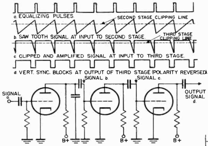
Figure 29. Formation of the vertical sync signal.
