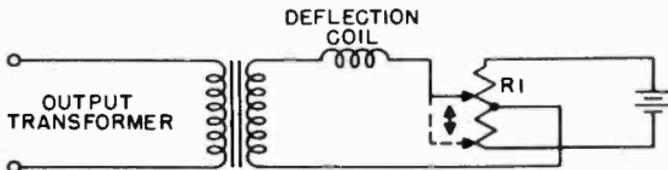
Figure 123. Positioning circuit for electromagnetic picture tube.
