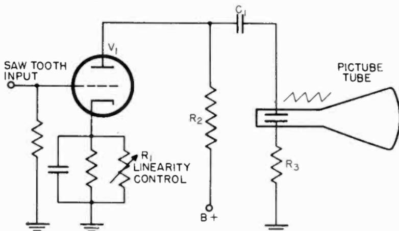
Figure 111. Sweep amplifier for use with electrostatic deflection.
