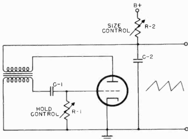
Figure 109. Blocking oscillator and discharge circuit.
