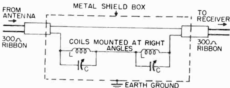
Figure 40. Circuit for wave trap.
