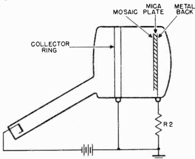
Figure 42. Path of electrons in iconoscope circuit.
