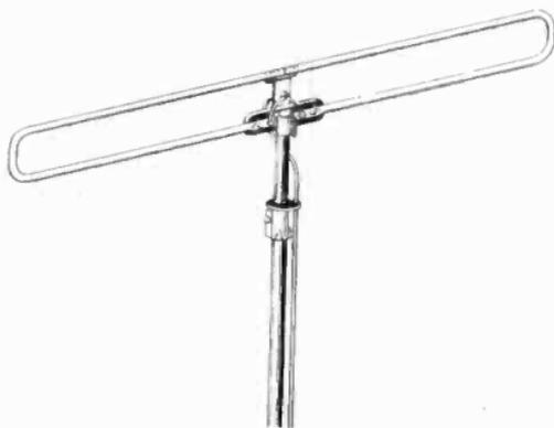
Figure 35. Folded dipole antenna. (courtesy Ward Products)
