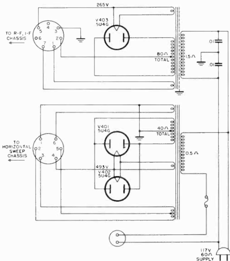
Figure 57. Low voltage power supply.
