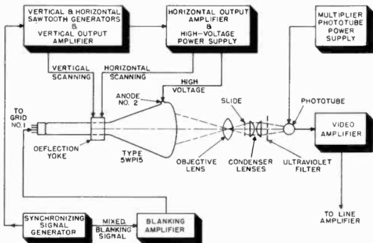
Figure 101. Block diagram of flying spot signal generator.
