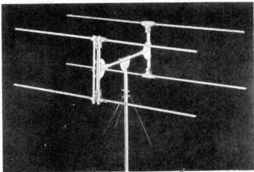
Figure 60. Stacked dipoles and reflectors. (courtesy Cameco)
