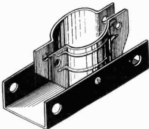
Figure 22. Mast base. (courtesy Taco)
