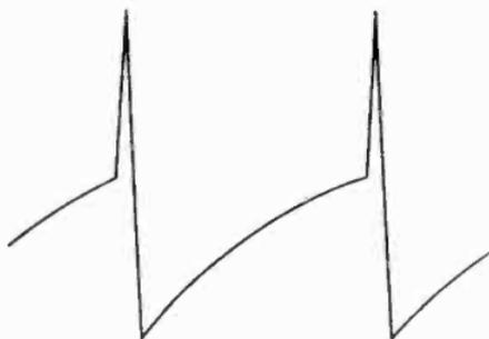
Figure 150. Pulses generated by blocking oscillator.
