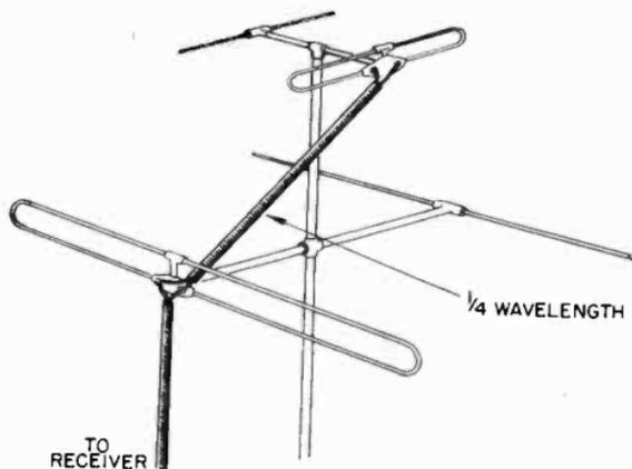
Figure 45. Antennas connected in parallel.
