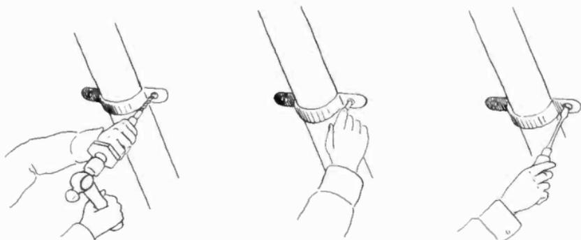
Figure 32. Drilling and mounting to masonry.
