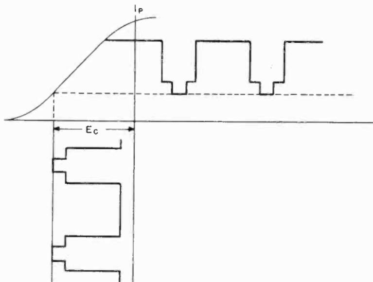
Figure 53. Grid characteristic of Class B modulated amplifier.
