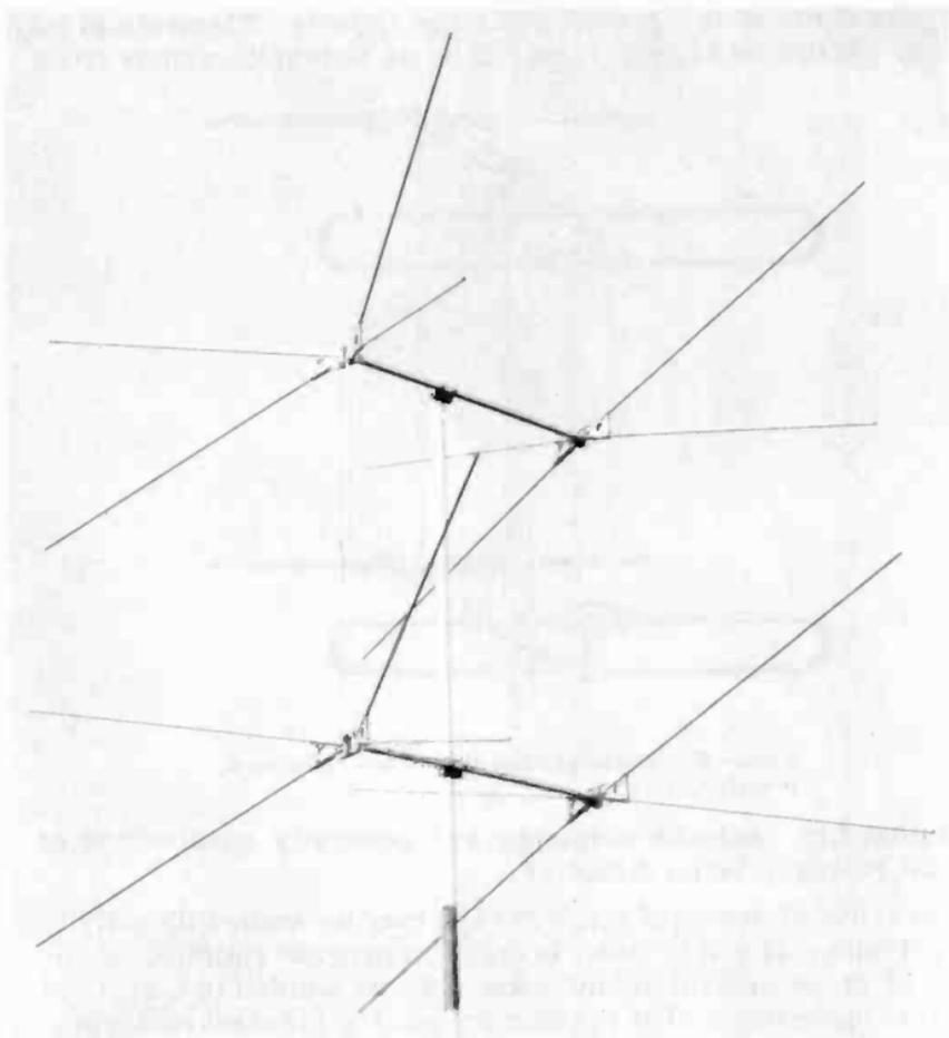
Figure 62. Four-unit double-V stacked antenna.
