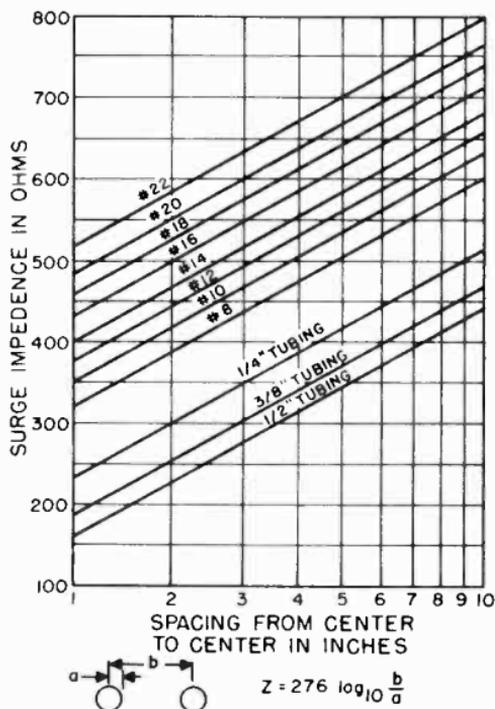
Figure 18. Characteristic impedance of two-conductor parallel transmission lines.
