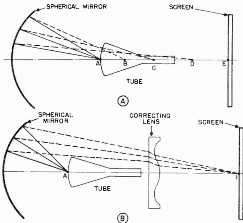
Figure 135. Function of correcting lens in Schmidt projection system.
