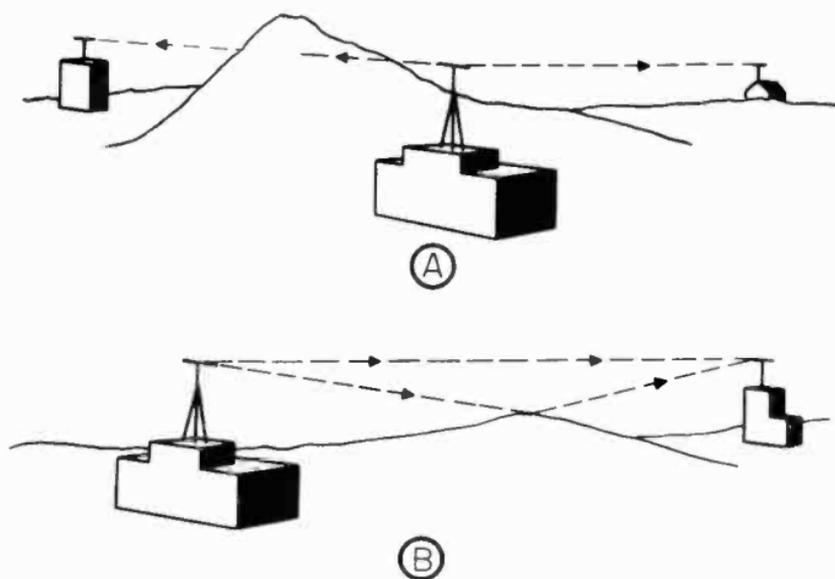
Figure 10. (A) Television signal weakened by intervening hill.
