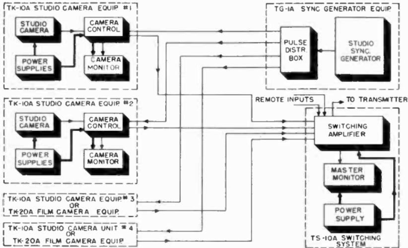
Figure 85. Block diagram of RCA studio camera equipment.
