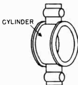
Figure 8. The focusing electrode assembly.
