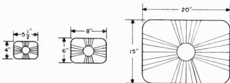
Figure 1. Relative picture sizes of seven inch, ten inch, and projection television receivers.
