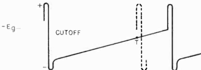
Figure 94. Grid voltage cycle of blocking oscillator.
