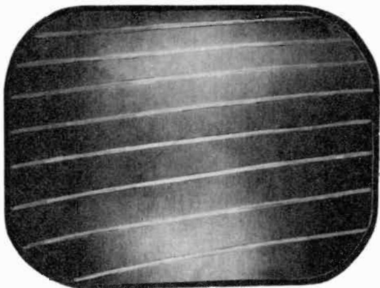
Figure 33. Illuminated pattern produced by applying sawtooth voltages, of different amplitudes, to the deflection plates.
