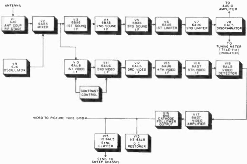
Figure 43. Block diagram of r-f, i-f chassis.
