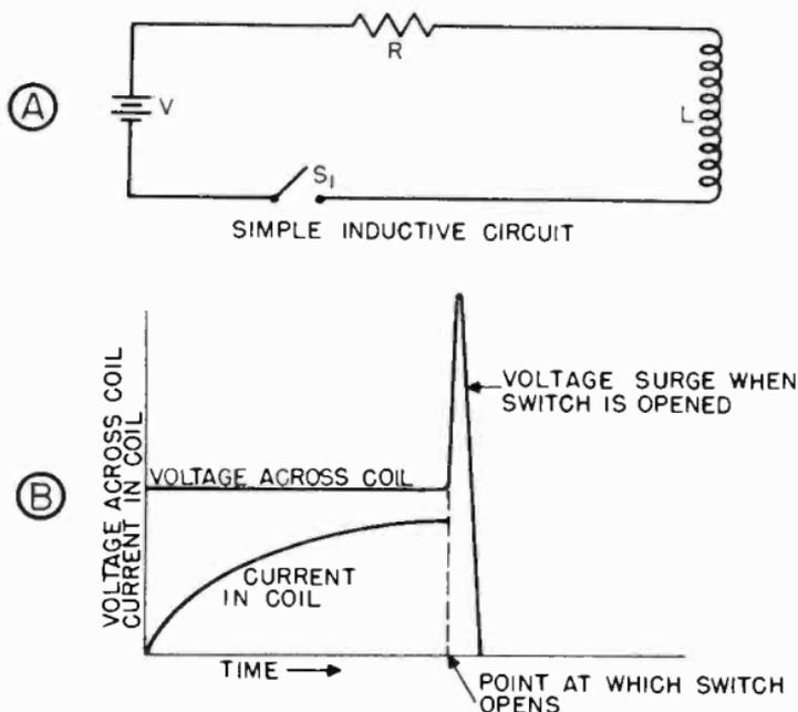
Figure 90. Operation of inductive differentiating circuit.
