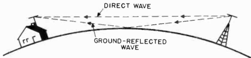
Figure 11. Cancellation of direct wave by ground-reflected wave.
