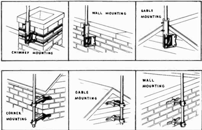
Figure 24. Two types of mounting brackets and the manner in which they are used. (courtesy General Cement).
