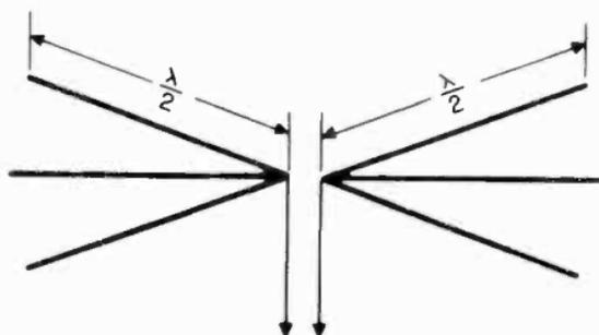
Figure 44. Full-wave fan antenna.
