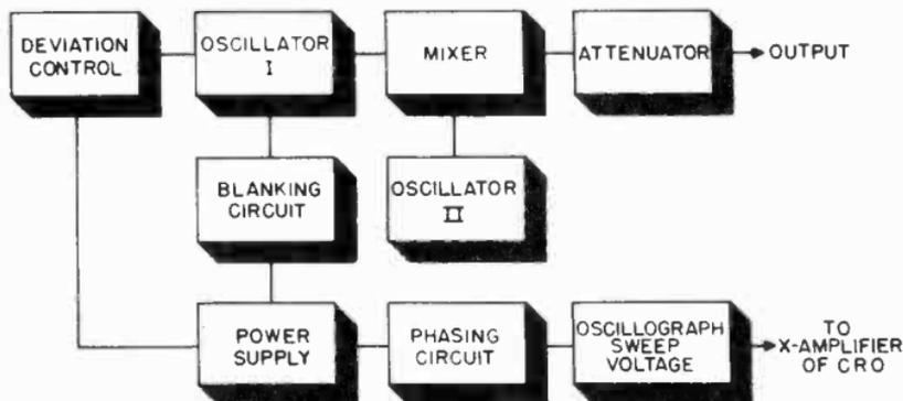
Figure 11. Block diagram of beat frequency wobulator.
