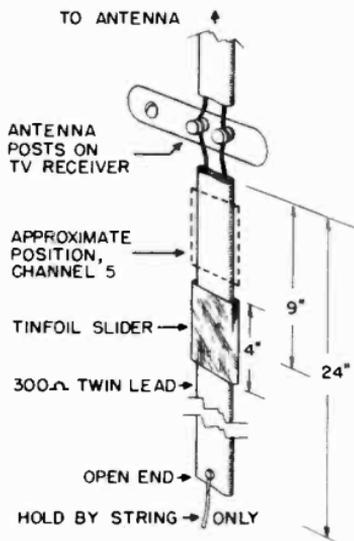
Figure 39. Simple wave trap.
