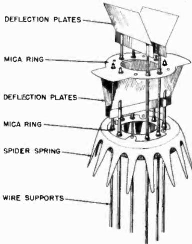
Figure 10. The deflection plate assembly.
