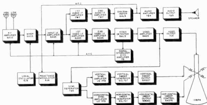
Figure 21. Block diagram of Philco Model 48-1000.
