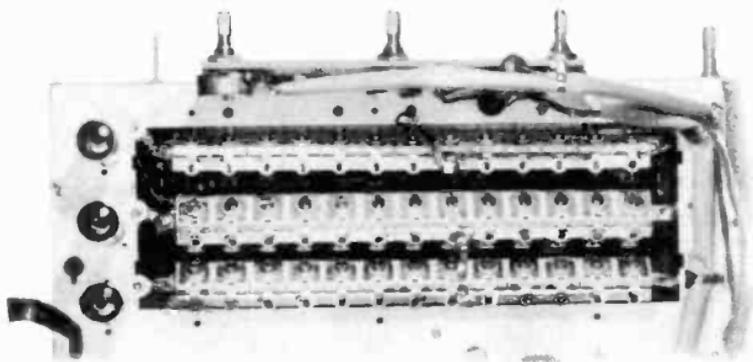
Figure 7. Layout of Hallicrafters thirteen channel, pushbutton tuner. (courtesy Hallicrafters)
