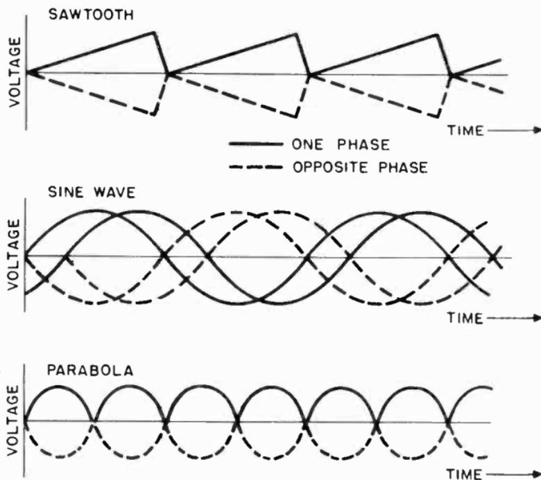
Figure 98. Waveshape used to shade picture.
