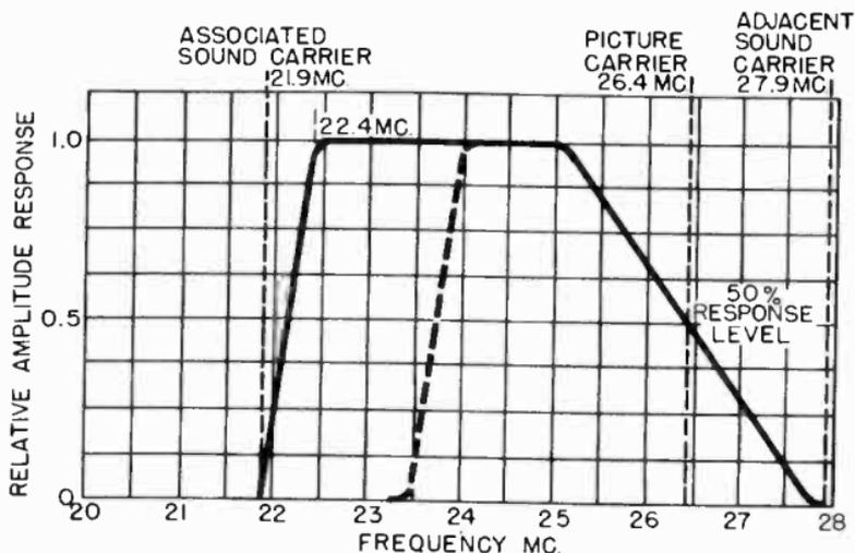
Figure 33. The ideal response curve for a television receiver.
