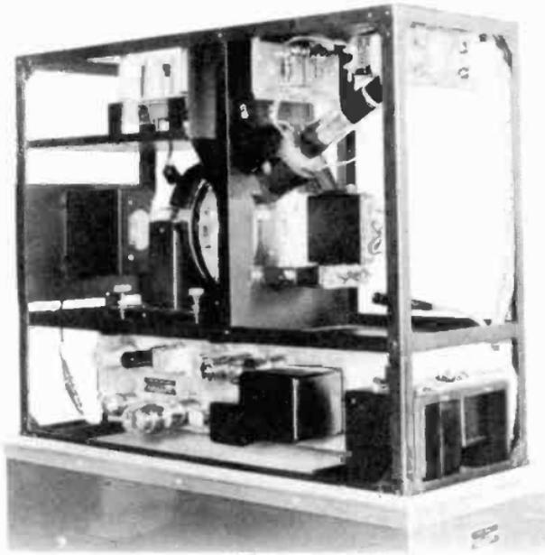
Figure 96. Iconoscope film pickup camera without shield covers. (courtesy DuMont)
