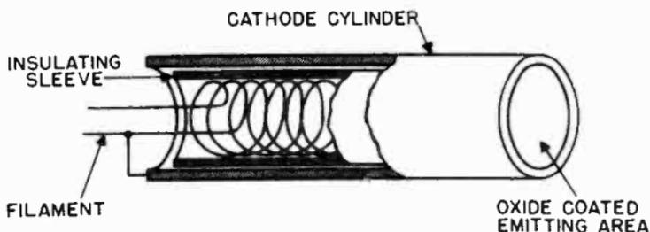
Figure 12. Heater and cathode assembly.
