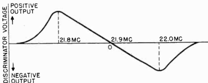
Figure 172. Response curve of typical television receiver discriminator.
