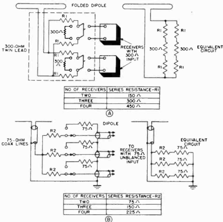
Figure 87. Simple master antenna system.
