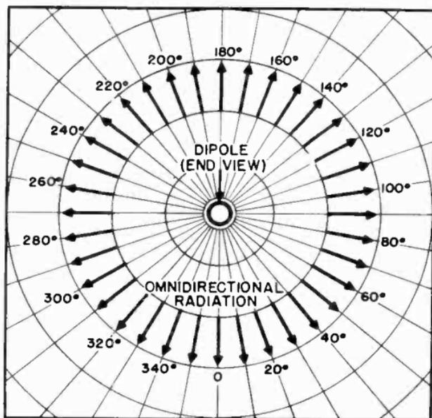
Figure 28. Vertical field pattern of horizontal dipole.
