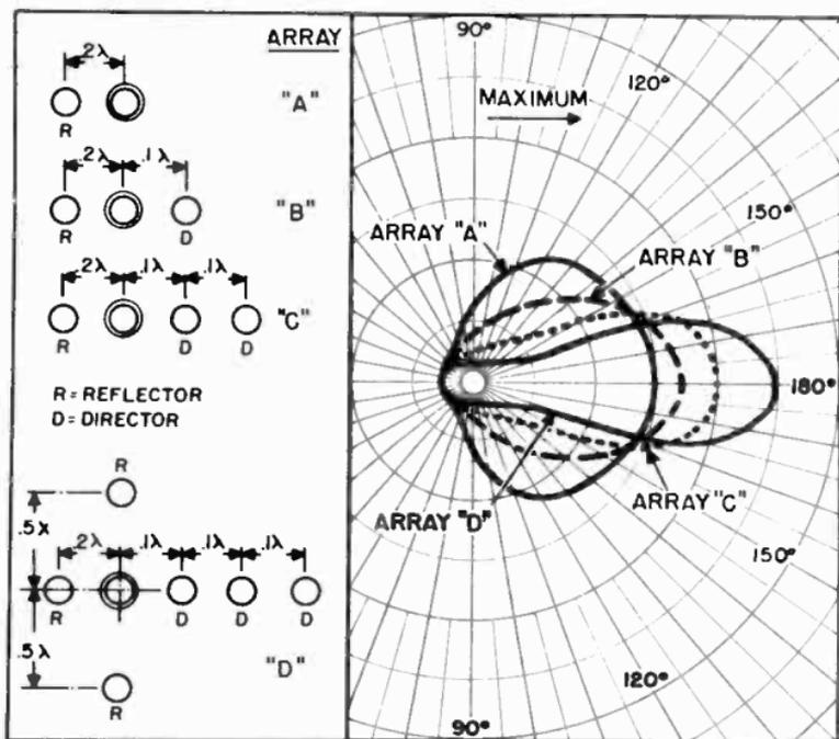
Figure 56. Field patterns of four parasitic arrays.
