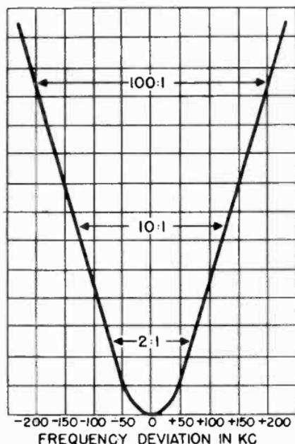
Figure 162. Typical i-f amplifier response curve.
