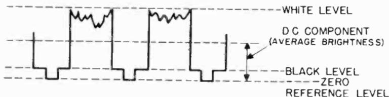
Figure 69. Composite video signal at the output of the video detector.
