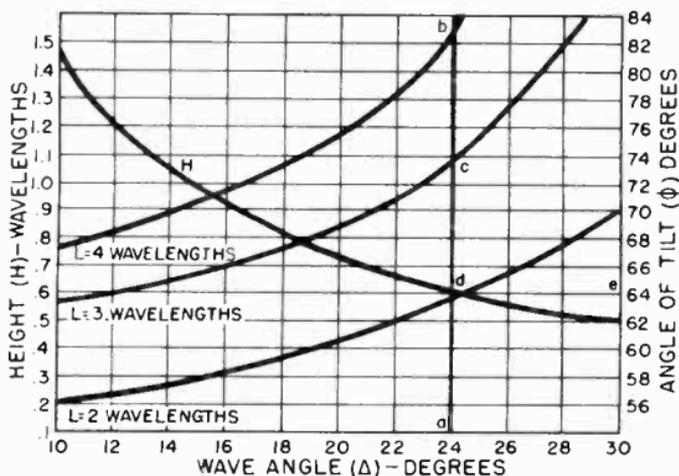
Figure 77. Design chart for rhombic antenna.
