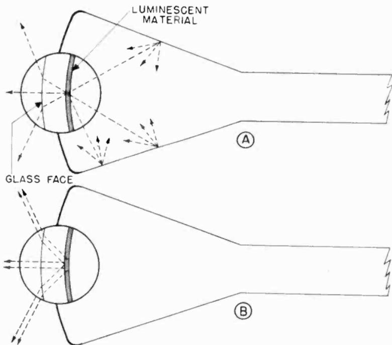
Figure 126. How aluminum backing increases image brightness.
