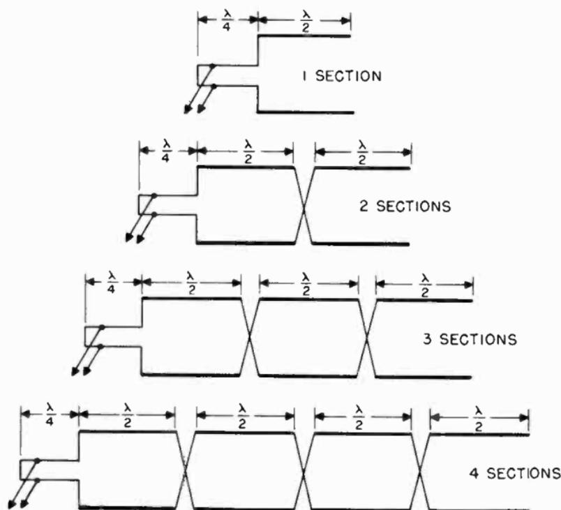
Figure 70. End-fed flat-top antenna arrays (top view).
