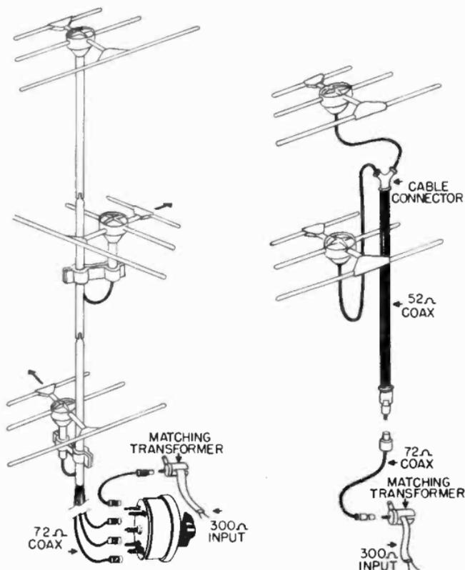
Figure 44. Typical application of coaxial switch.
