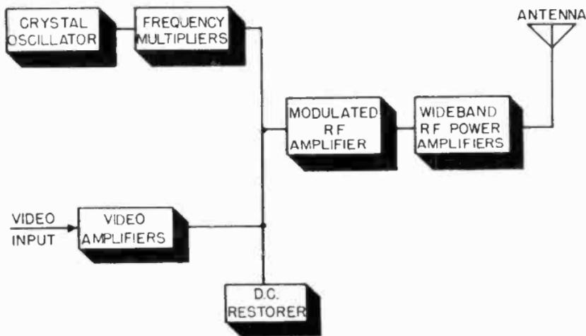
Figure 43. Block diagram of low level modulated transmitter.
