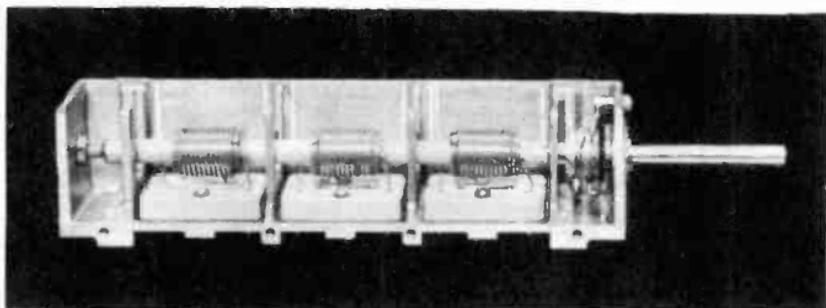
Figure 10. The Inductuner. (courtesy DuMont)
