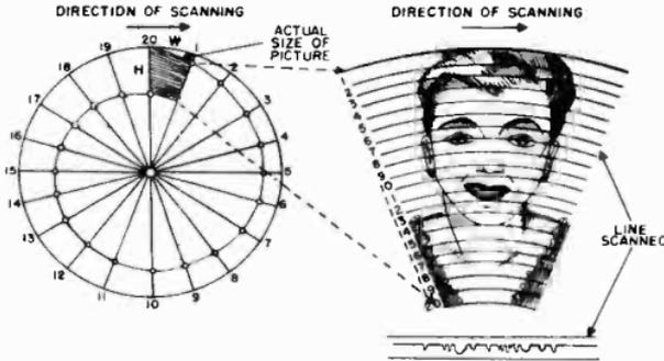
Figure 10. Rotating disc used in Nipkow's television system.
