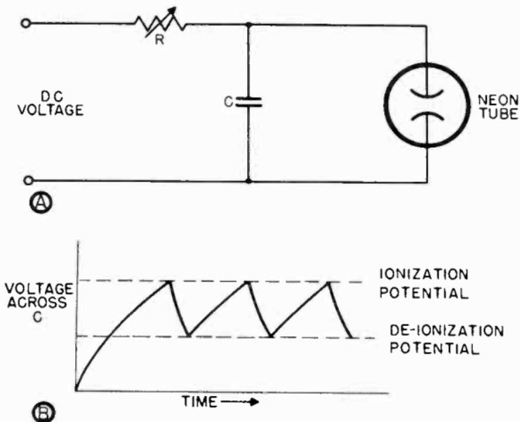
Figure 106. Simple electronic saw-tooth generator.
