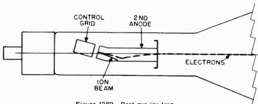
Figure 128B. Bent gun ion trap.
