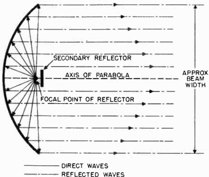
Figure 80. Reflecting action of parabolic surface.
