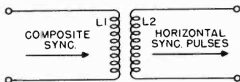
Figure 91. Transformer type differentiating circuit.
