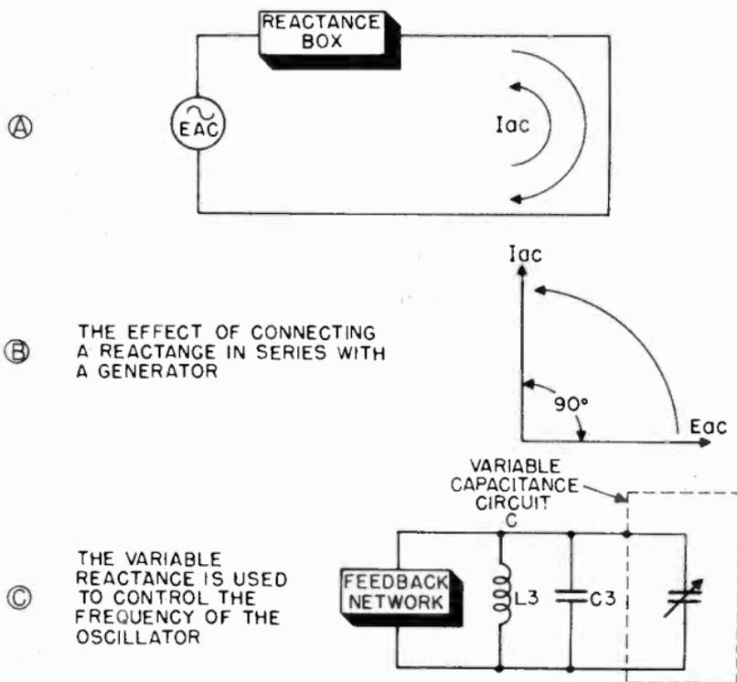
Figure 159. Operation of reactance modulator.
