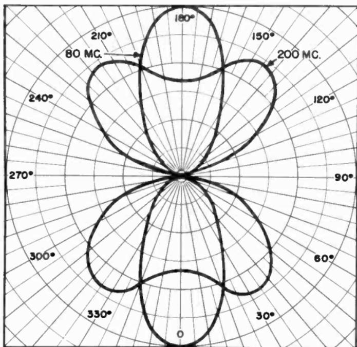
Figure 43. Horizontal field patterns of fan antenna at 80 Mc and 200 Mc.
