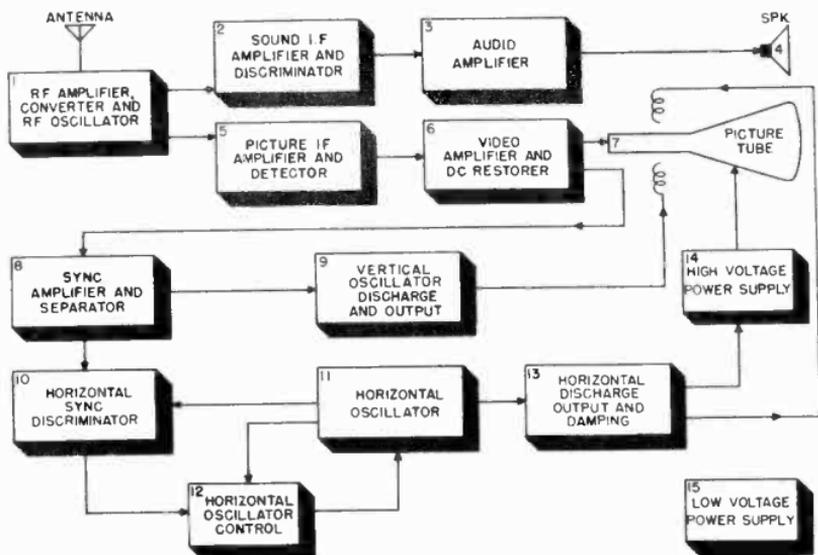
Figure 181. Block diagram of television receiver using ten-inch tube.
