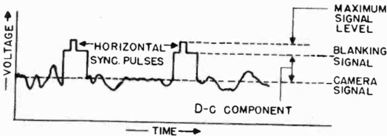
Figure 39. The completed composite video signal.
