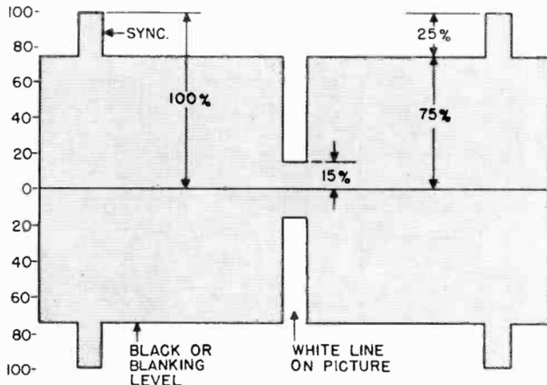
Figure 54. Modulation limits of transmitter.
