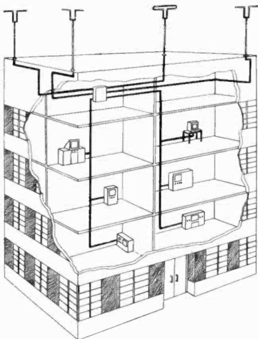
Figure 85. Typical master antenna installation.
