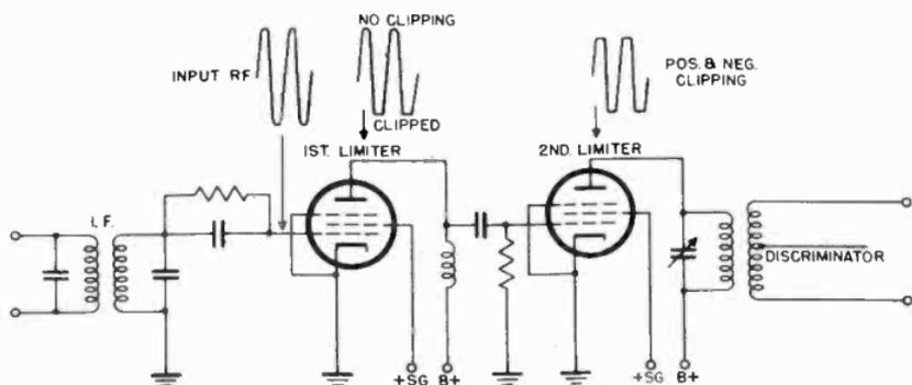
Figure 167. Dual or cascade limiter.
