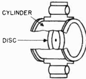
Figure 9. The accelerating electrode assembly.
