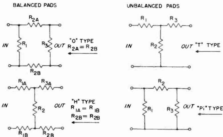
Figure 38. Attenuator network and component values.
