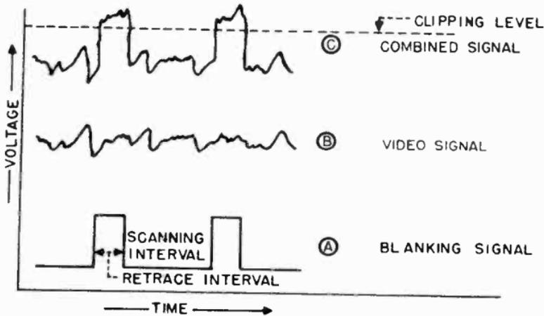
Figure 38. How blanking signal is combined with video signal.
