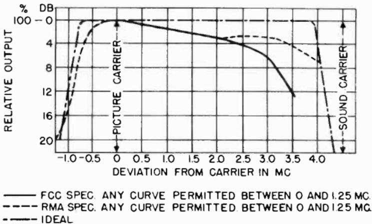
Figure 41. RMA and FCC specified transmission channels.
