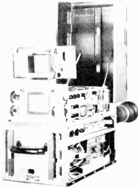
Figure 14. Pickup head and electronic viewfinder.
