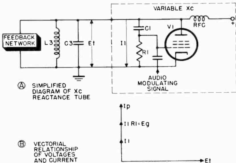
Figure 160. Simplified schematic of a reactance tube modulator.
