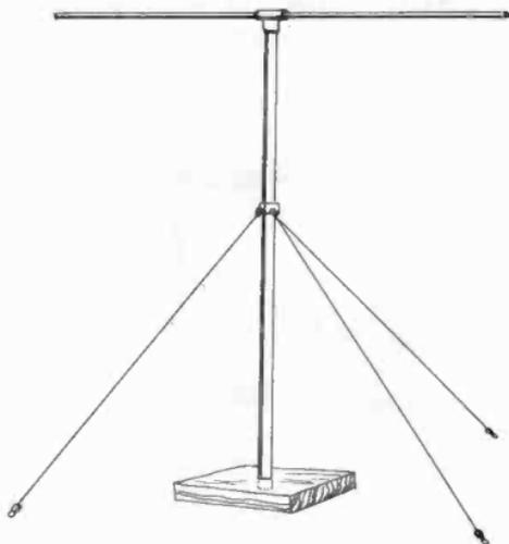
Figure 21. Mounting antenna on a roof.
