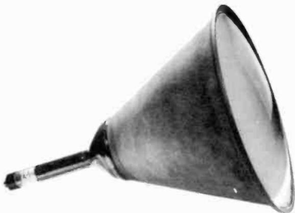
Figure 130. Picture tube with metal funnel.
