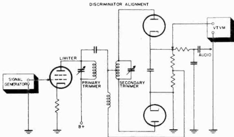
Figure 56. Connections used when aligning discriminator using v.t.v.m.
