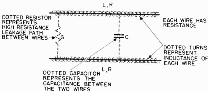
Figure 12. Distribution of resistance, capacitance, and inductance along section of two-wire transmission line.
