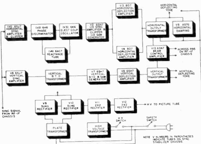
Figure 48. Block diagram of sweep chassis.
