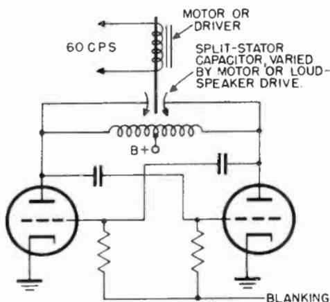
Figure 10. Variable capacitor circuit for wobblator.
