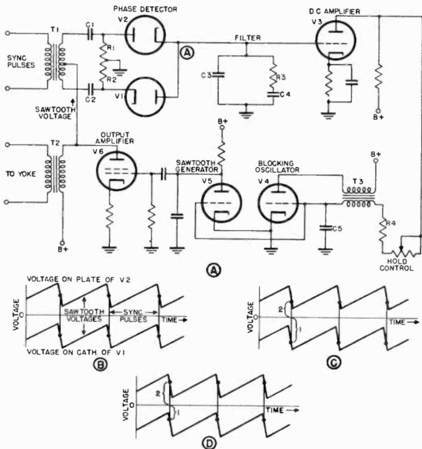
Figure 99. A.F.C. sync circuit and operating waveform.
