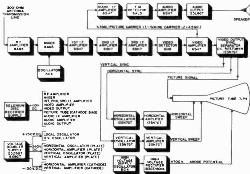
Figure 14. Block diagram of Hallicrafters Model T-54.
