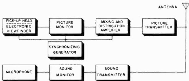
Figure 1. Block diagram of simple television transmitter.
