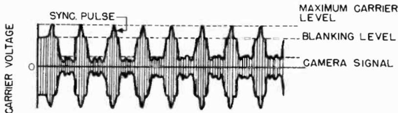
Figure 57. Modulated television carrier.
