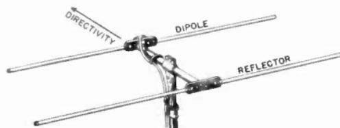
Figure 51. Dipole and reflector.
