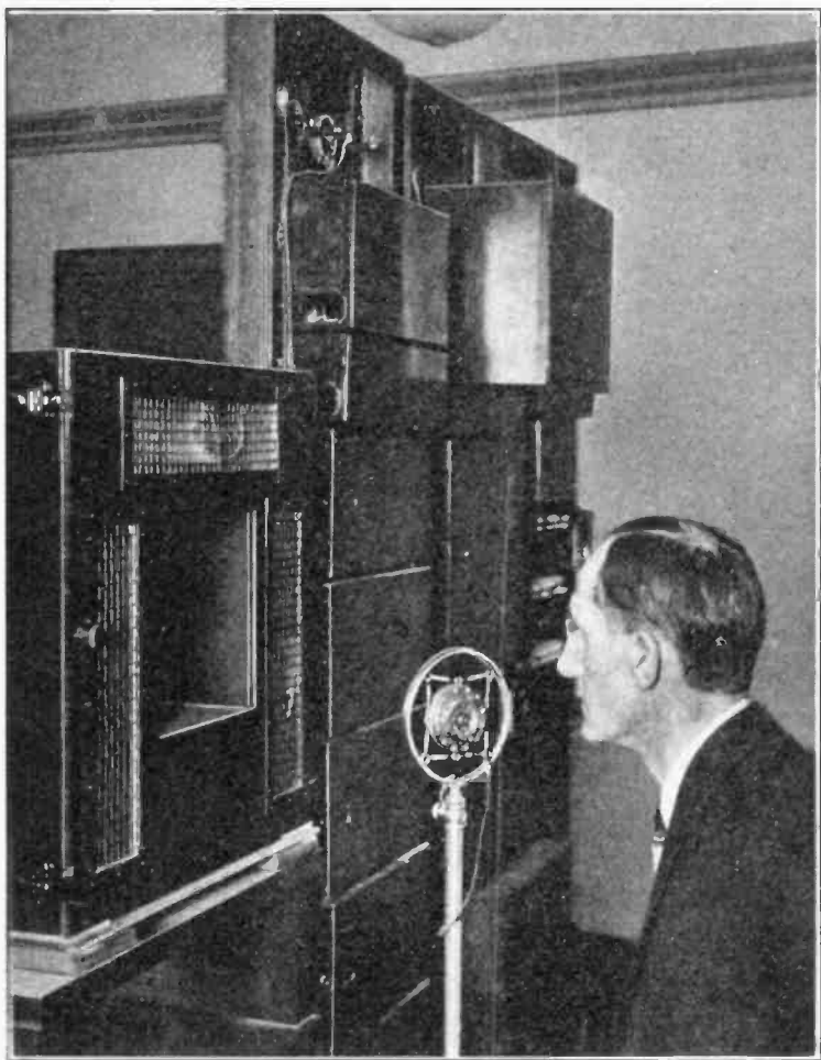
This is the television transmitting apparatus installed at Washington, D. C., which enabled an audience in New York to see as well as hear Secretary Herbert Hoover as he spoke via the long-distance lines of the A. T. & T.
