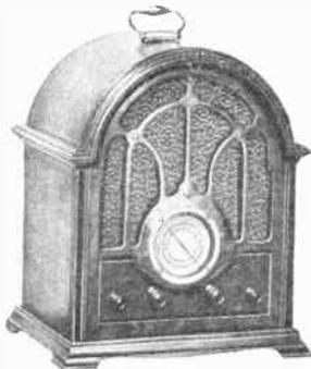
**MODEL K-64**—Dual-band table model with a short-wave band from 19 to 49 meters and a standard broadcasting band from 540 to 1500 kilocycles. A-c. superheterodyne circuit. American broadcasts, foreign stations, amateur and aviation signals. Cabinet of two-toned walnut and Oriental wood veneers.
