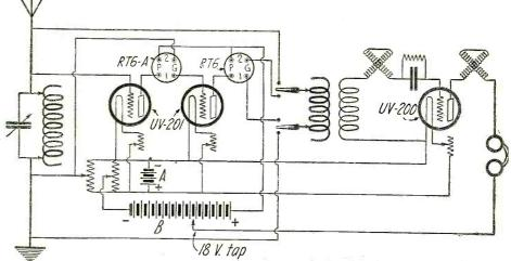
Hook-up of the DX Receiver. By Means of Two SPST Switches Only the Regenerative Set May Be Used. The Tubes May Be of Any Suitable Make, Such as Radiotron, Cunningham, etc.
