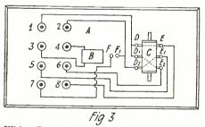
Wiring Connections of the Selector Including the Electro-Magnets B and the Revolving Drum C.
