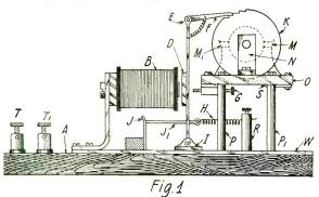
The Automatic Selector Used to Open and Close Various Local Circuits.
