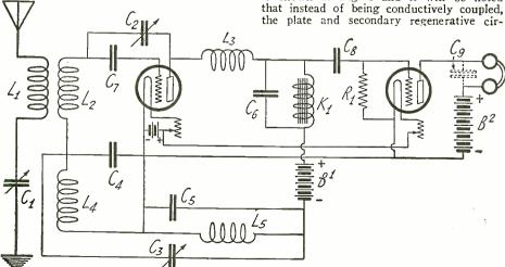
Feb. 2. The Same Circuit with the Addition of a One-Stage Choke Coil Audio Frequency Amplifier.
