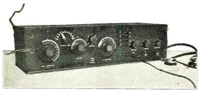
View of the Tuner and De-tector-Amplifier Units. An Ar-ticle on the Construction of the Tuner Ap-peared in the October Issue of Radio News
