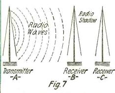
Station B Absorbs and Reflects Wave Energy, Preventing Any from Reaching C, Thus Making a "Radio Shadow" Behind B.
