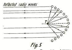
Vertical Section Showing Transmitting Antenna T, and the Wires Forming an Electrical Mirror.
