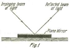
Illustrating the Reflection of a Beam of Light from a Mirror.
