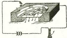
1- Bell receiver. 2- Second contact piece 3- Point of contact. 4- Contact piece Tastened to membrane.
