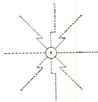
Fig. 45. Kinks Produced on Radial Electrolines of an Electron E When the Latter Suddenly Jumps Forward. The Dotted Lines Denote the Jumps Forward. Electrolines.
