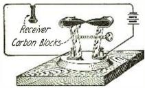
22. Another Form of Carbon Microphone Provided with an Adjusting Screw.
