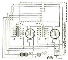
The Proper Way of Connecting Two Stages of The Proper Way of Connecting Two Stages of Radio Frequency to a Westinghouse R.C. Receiver is Shown Above. It is Not Necessary to Disturb the Interior Wiring of the Set, All of the Connections Being Made Directly to the Binding Posts. A 45-Volt "B" Battery Is Used for All Four Amplifying Tubes.
