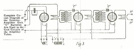
The proper voltage will have to be inet. ascertained by trial. This will probably be found to be somewhere between four and eight volts. As the "C" battery supplies practically no current, small two-cell flashlight batteries of ten-cent store variety may They will last indefinitely.
