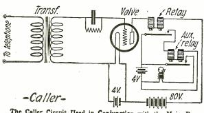
The Caller Circuit Used in Conjunction with the Main Receiver. The Bell is Arranged to Ring on the Wave-Length for Which the Receiver is Tuned.
