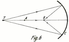
Intensity of Radio Waves at B May be Much Greater Than at A, Even if A is Nearer T, on Account of the Reflected Waves from C Adding to the Original Waves at B.
