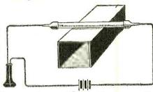
Fig. 19. One of Hughe's Microphones. The Glass Tube is Filled with Bronze Powder. Its Action is Similar to That of the Carbon Grain Type of Microphone.
