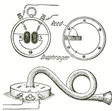
Fig. 14. The Gower Receiver. The First of the Watch Case Type. This Used a Magnet That Would Lift 11 Lbs.
