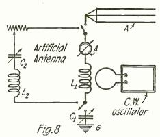
System Used of the Measurement of Antenna Resistance.
