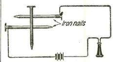
Fig. 20. The Hughe's Nail Microphone Its Function Resting on Imperfect Contact.
