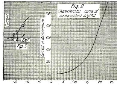
Characteristic Curve of a Curve of a Carborundum Crystal Showing the Relative Current at Various Ap-plied Poten-tials.
