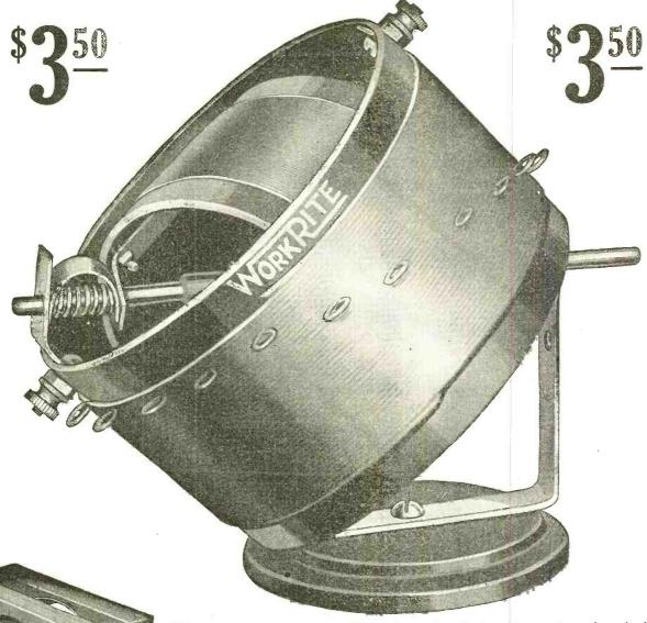
This instrument represents perfection in getting all dimensions and number of wire turns JUST RIGHT. Both primary and secondary are made from molded Bakelite and are wound with green silk wire. Range from 180 to 800 meters. Has 12 taps. Tunes twice as sharp as the ordinary 90° coupler. One WorkRite Super 180° Variocoupler and two WorkRite Super Variometers make up the WORKRITE TUNER TEAM—the most selective circuit obtainable. Can also be used in single circuit.
