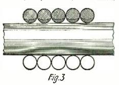
The Current Density in a Coil of Wire is Greatest on the Inside as Shown by the Shaded Portions.
