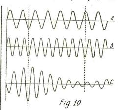
The Effect of Wave Motions A and B, Acting Together in the Same Space, is Shown in C.
