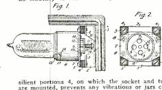
silient portions 4, on which the socket and tube are mounted, prevents any vibrations or jars contributed to the casing to which the bracket 2 is attached, from seriously affecting the lamp.
