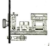
post in electrical contact with the shielding may be put on the back, in a position so as not to interfere with the battery connections. This post may then be connected with a short length of wire to the regular ground connection.
