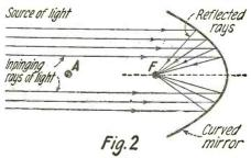
Light is More Intense at F Than at A (on Account of Concentrated Reflection at F) Even Though A is Nearer the Source of Light Than F.
