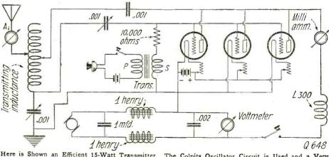
Here is Shown an Efficient 15-Watt Transmitter. The Colpits Oscillator Circuit is Used and a Very Good Range Can Be Obtained.
