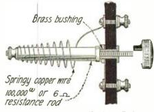
Here is a Unique Means of Varying a Resistance. This Makes a Very Effective Rheostat or Variable Grid Leak.
