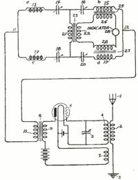
of direction and magnitude, a condition is ob-tained where the intereference effects are balanced out, and the indicating instrument responds only to the signals which are to be received.
