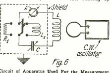
Circuit of Apparatus Used For the Measurement of Resistance. In This Case a Standard Resistance is Employed.
