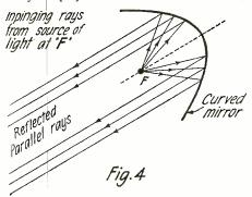
Showing How Shifting the Mirror Without Moving Source of Light F Results in Shifting Direction of Parallel Reflected Rays, Thus Enabling Us to Control Direction in Which Reflected Light is Flashed.
