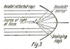
Showing How Source of Light at Focus of Parabolic Mirror Reflects Parallel Rays in One Direction.
