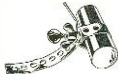
a good permanent ground on water pipes, etc.
