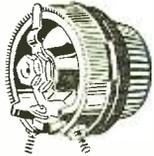
The rheostat shown in the illustration was submitted to the Radio News Laboratories for test by the Pilot Electric Mfg. Co., 113-119 Broadway, Brooklyn, N. Y. This rheostat has a rate of resistance of six ohms and operates satisfactorily as a filament control in radio receivers.
